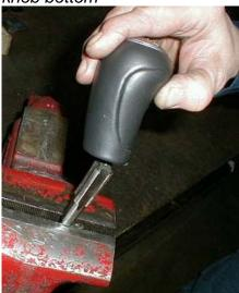
D. Place supplied tap (5/8x16NF) into a vise and proceed to tap the shifter knob hole till tap bottoms in shifter knob hole. Remove any plastic chips from shifter knob hole.
