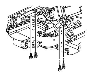
D. Remove the inner transmission mounting bolts.
