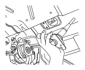
16) Remove the shift control assembly from the transmission. Remove the shift control assembly from the vehicle.
