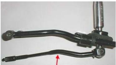
28) Reinstall shift rod onto shift lever, noting correct shift rod position and that the flat portion of the shift lever labeled FRONT is facing the front of the vehicle.
