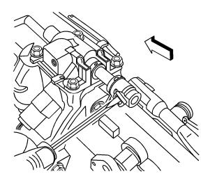
14) Using a flat blade tool, release the center shift control rod pin retainer. The graphic shows the transmission removed for clarity.
