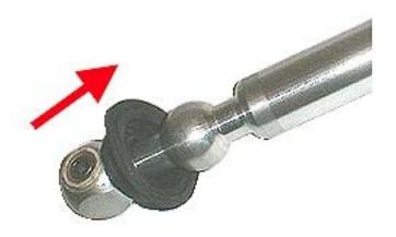
23) Remove the shifter boot black seal from old shifter.
