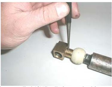
22) <u>Using supplied 1/16" roll pin punch, drive out the roll pin retaining the T-shaped shifter end.</u>
