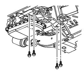
B. Install the inner transmission support mounting bolts. Do not tighten at this time.
