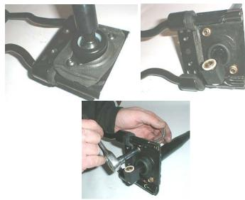
27) Insert the supplied pan head bolt through the top retaining plate rivet holes and secure underneath the baseplate with supplied flanged nuts.
