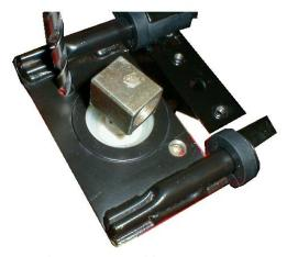
After removing the shifter assembly from the vehicle, secure the shifter baseplate and prepare to drill out the two rivets that retain the shifter cover to the baseplate with the supplied 5/16 drill. Debur the drilled out rivet holes.
