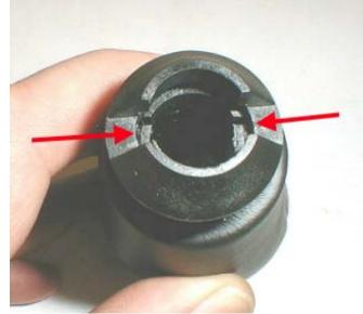
B. Remove shift knob retaining clip located underneath the shifter boot by depressing the two tabs on the shift knob with needle nose pliers. Discard removed retaining clip. Remove shift knob from shifter boot.
