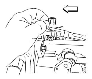
2. Install the center shift control rod pin retainer.
