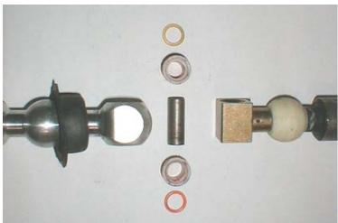
21) Remove the bushing, seals and spacer from the end of the shifter
