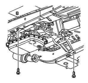
C. Remove the outer transmission mounting bolts.
