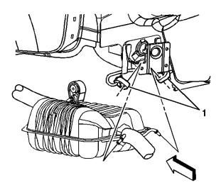
D. Press the tail pipe hangers (1) over the tail pipe hanger rods.
