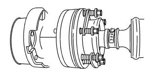
B. Reference mark the location of the propeller shaft CV joint to the differential flange.
