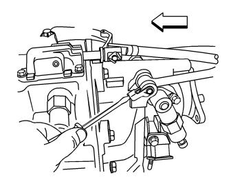
12) Using a flat blade tool, release the left side shift control rod pin retainer. The graphic shows the transmission removed for clarity.
