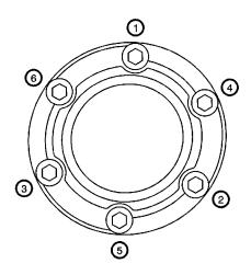
L. Install the propeller shaft CV joint-to-differential flange bolts. **Tighten**
