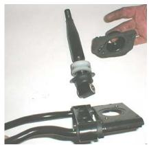
26) Place the shift lever into the base plate and place the top retaining plate over the shift lever till it contacts the base plate.
