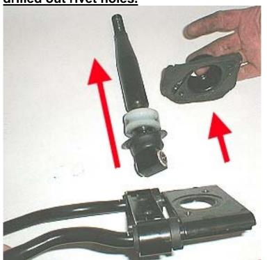
19) Pull up on the shifter to remove the shifter and shifter cover from the baseplate.
