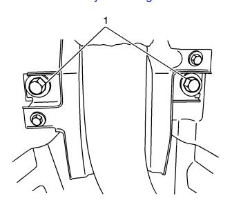
A. Remove the bolts (1) securing the support bearing to the vehicle underbody.
