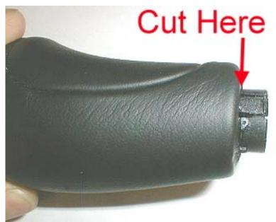
C. Cut off bottom of shift knob collar so that it is flush with leather portion of shift knob bottom
