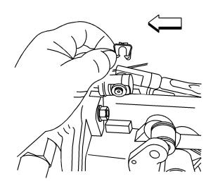
15) Remove the center shift control rod pin retainer.
