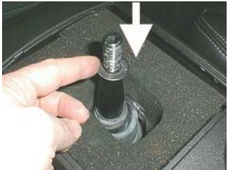
A. Place flat washer over threaded end of shifter.
