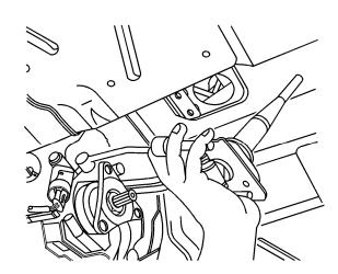
1. Install the shift control assembly to the transmission.
