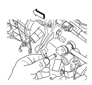
3. Install the left side shift control rod pin. Rotate the pin in order to lock the retainer into place on the transmission.
