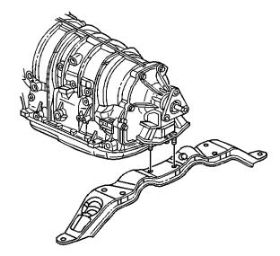
A. Install the transmission support to the vehicle.
