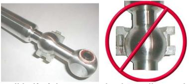
25) Install half of the removed nylon collar as shown with the shift lever sphere positioned near the top of the collar. Apply a light coating of grease to the sphere surface and snap the other half of the collar in place.
