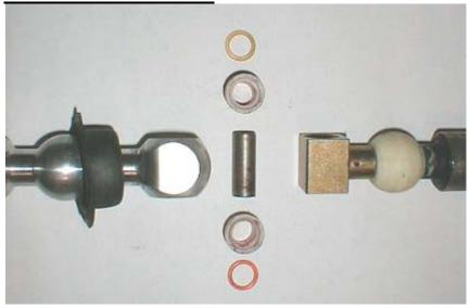
24) <u>Install removed bushing, seals and spacer onto shift</u> rod end of shifter.
