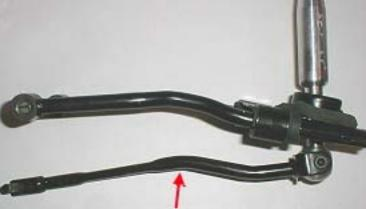
17) After noting the orientation of the horizontal shift rod, remove the shift rod from the shift lever.
