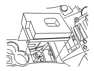
2) Remove the sound insulator foam block from the console.
