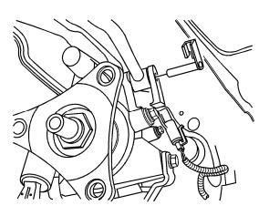
4. <u>Install the right side shift control rod pin. Rotate the pin in order to lock the retainer into place on the transmission.</u>
