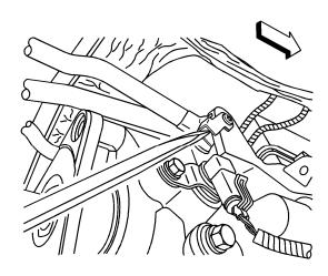
10) <u>Using a flat blade tool, release the right side shift control rod pin retainer.</u>
