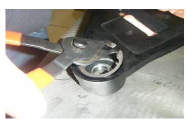
16. Using a pair of snap ring pliers, install the supplied snap ring into the groove directly above the bearing in the rear tensioner bracket bearing housing.
