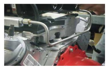
29. It there is sufficient clearence under the rear jackshaft pulley, re-install the stock fuel line onto the fuel rail. If there is not enough room for the stock fuel line, as is true with a 3.49" rear jackshaft pulley, install a new fuel line that allows clearance for the new rear pulleys or modify the stock fuel line accordingly.
