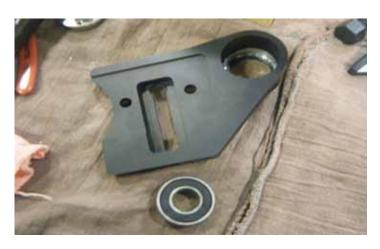
13. The adjacent illustration shows the LPE supplied rear tensioner bracket and it's bearing, which will be installed in the following step. Make sure to apply lubricant to the bearing before attempting to press the bearing into the bracket.
