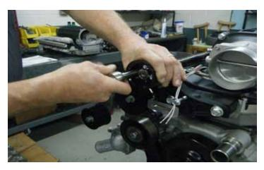
4. Using a 10mm socket, remove the front supercharger pulley.
