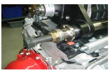
20. Slide the front of the jackshaft into the foward bearing housing. After lubricating the end of the shaft, install the pulley hub onto the shaft. Whatever method you use to install the pulley hub, make sure that the hub stays square as you tighten it, or else you may damage the hub.
