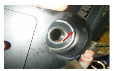
15. After pressing the bearing into the rear tensioner bracket to the correct depth, the snap ring groove inside the bearing housing should be visible, as shown in the adjacent picture.
