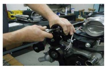
36. Using a 10mm socket, re-install the front supercharger pulley. Torque the bolts to 106 inlbs.
