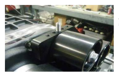
33. Lower the tensioner pulley into position. Install the proper set screw for your pulley/belt configuration. There are three different size set screws supplied in this kit.
