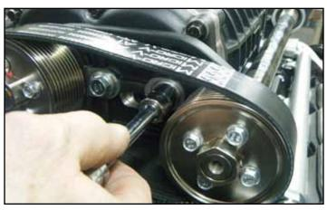
6. Remove the two (2) rear pulley bracket bolts using a 15mm socket.
