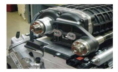
9. Remove the rear supercharger belt and pulleys.
