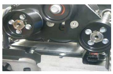
30. Using a 10mm socket the eight (8) bolts that were removed in step 7, we will now install the new 14-rib rear pulleys. Start all eight bolts, but only tighten the passenger-side pulley. Torque the bolts on the passenger-side pulley to 106 in-lbs.
