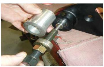
18. Using whatever method you choose, pull the end of the jackshaft through the bearing. Again, this operation should not take excessive force to complete. As illustrated in the following step, the end of the jackshaft should portrude out of the bearing by roughly 1.1 inches.
