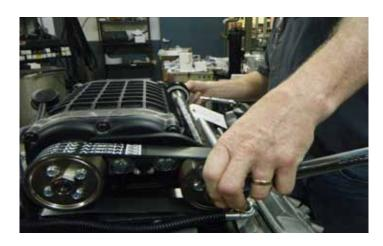
2. Using a 1" wrench and 1" socket, break the bolts loose that hold the jackshaft in place.
