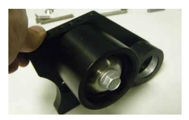
25. The adjacent illustration shows the tensioner pulley fastened to the tensioner bracket by the T-nut from the front.
