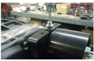
34. Using the supplied washer, nut, and a 4mm Allen socket, secure the set screw to the bracket.
