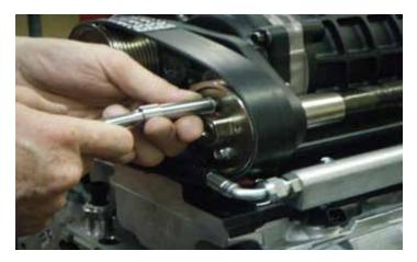
7. Using a 10mm socket, remove the bolts on both rear supercharger pulleys.
