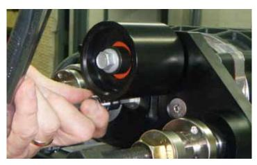
26. Using a 6mm allen socket and blue loctite, install the two (2) M10x1.5x30 flat head countersunk bolts (PN: KP82415) that fasten the tensioner bracket to the rear of the supercharger. Torque the bolts to 35 ft-lbs.
