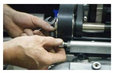
8. Using an 11/16" wrench, remove the rear fuel line hose from the passenger side fuel line.
