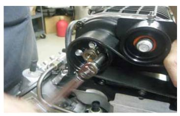
32. Using the belt to hold the pulley in place, tighten the bolts on the driver-side pulley. Torque the bolts to 106 in-lbs.
