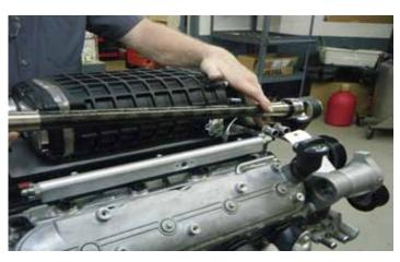
10. Gently pulling towards the rear of the supercharger, remove the supercharger jackshaft assembly from the forward jackshaft housing.
