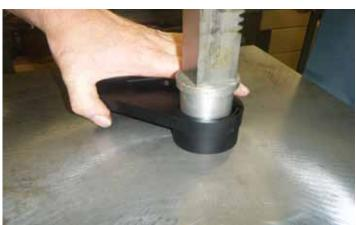
14. Using an arbor press or equivalent, press the new bearing into the new tensioner bracket until some resistance is felt. This operation should not take excessive force to complete.
