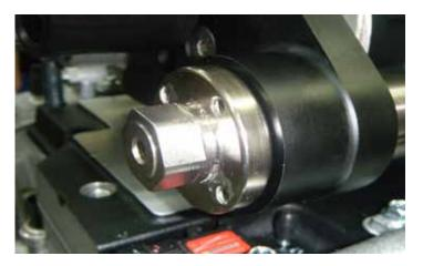
27. Tighten the pulley hub against the end of the jackshaft. The end of the jackshaft should be flush with the outside of the pulley hub, as shown in the picture.
