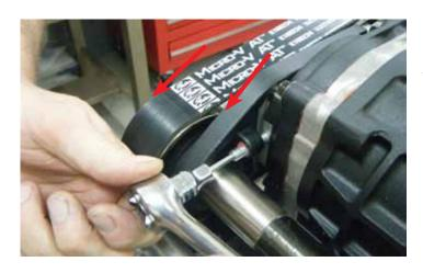
5. Loosen the rear tensioning screw on the passenger side of the supercharger with a 4mm Allen socket.
