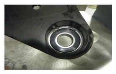
17. The adjacent illustration shows the snap ring installed into the bearing housing.
