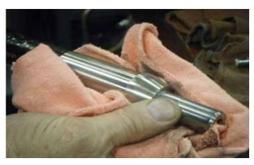
12. Wipe off the surface on the end of the jackshaft where the bearing will make contact to ensure that there are no particulates on the contact surface.
