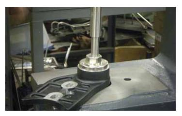
11. Using an arbor press or equivalent, press the jackshaft out of the pulley hub and bearing. Inspect the individual components after their separation is complete to confirm that no components have been damaged. If any component was damaged during the pressing process, it will need to be replaced.
