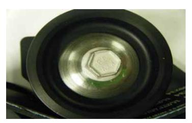
35. Tighten the idler pulley bolt until belt is secure.
