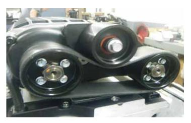
31. Install the belt onto the rear pulleys. This will help hold the driver-side pulley in place while being tightened. Work the belt onto the pulleys by running the belt back and forth over the pulleys.
