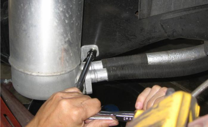
16. At this point in the installation it is recommended to have another person to help remove and place the oil tank. While one person is holding the top of the tank, remove the two (2) 15mm bolts on the mounting bracket on the bottom of the oil tank that secure the tank and bracket assembly to the vehicle.
