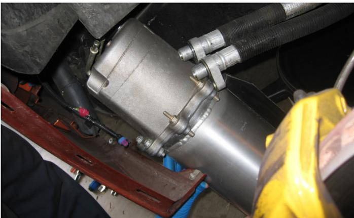
29. Place the tank inside of the passenger front fender with the tank's expanded oil volume section pointing towards the rear of the vehicle.
