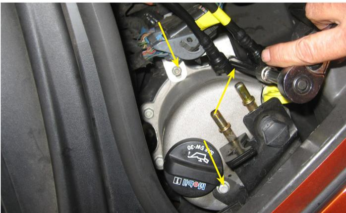
33. Using a 10 mm socket, install the three (3) bolts on top and torque each to 89 lb-in (10 Nm).
