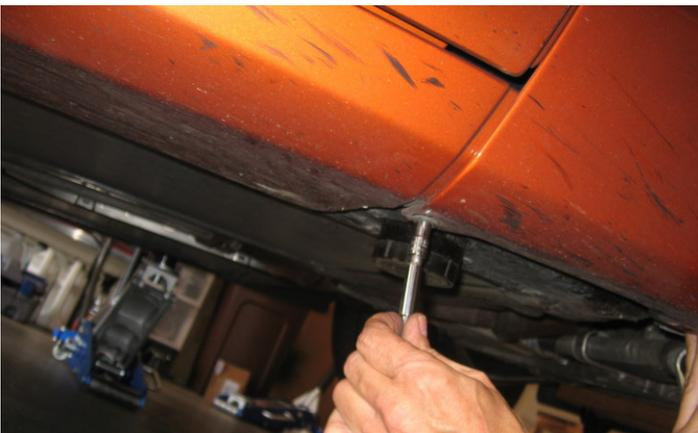
37. Position the fender back into place and, using a 7 mm socket, install the bolt that was taken off in step 9.
