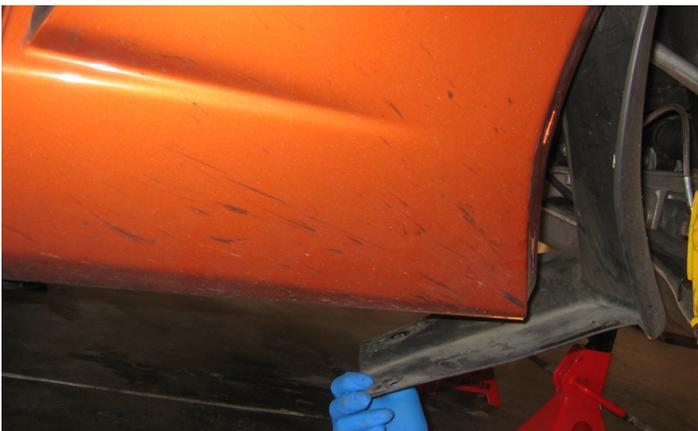
9. The liner is attached to the fender with metal push-clips. Start with the lower portion of the liner and pull the liner straight out of the fender.
