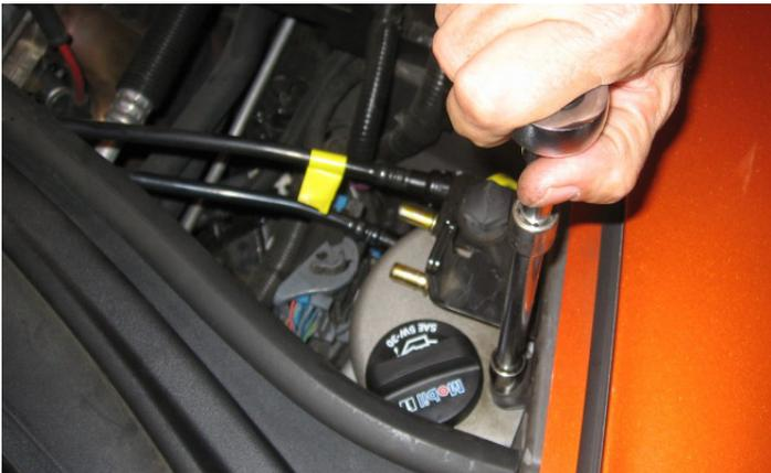
13. Using a 10 mm socket and extension, remove the bolt on the top of the tank located directly between the oil cap and the fender.
