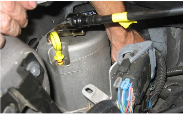
18. Remove the tank from the car by having one person pull the tank down through the bottom of the fender while the other person carefully moves the tank out of the way of the wiring harness as well as any other obstructions.
