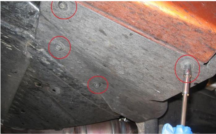
7. Using a 7mm socket for the outer bolts and a 10 mm socket for the inner bolts, remove the passenger front fender liner.
