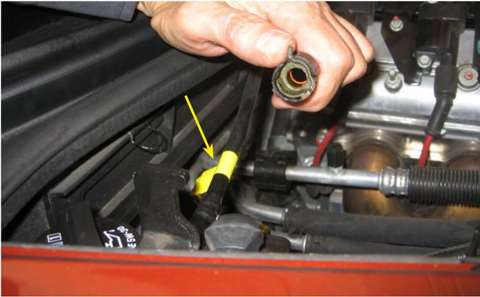
11. Mark one of the vapor lines as well as its respective port with a piece of tape (or equivalent) and remove the vapor lines from the top of the tank. This is done by pushing the small tabs on the ends of the lines clockwise and pulling outward.
