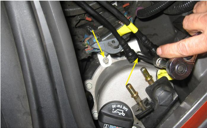
12. Using a 10 mm socket and extension, remove the two bolts from the bracket holding the middle of the tank. Be careful not to drop the two bolts once you remove them.
