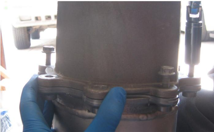
27. After aligning the tanks, using a 13 mm socket and extension, torque the eight (8) bolts to 18 lb-ft in an 8-bolt star pattern (25 Nm). Remember that you will need a deep well socket to torque the longer bolts. The tape used to mark the tank should be in between the two (2) longer bolts.
