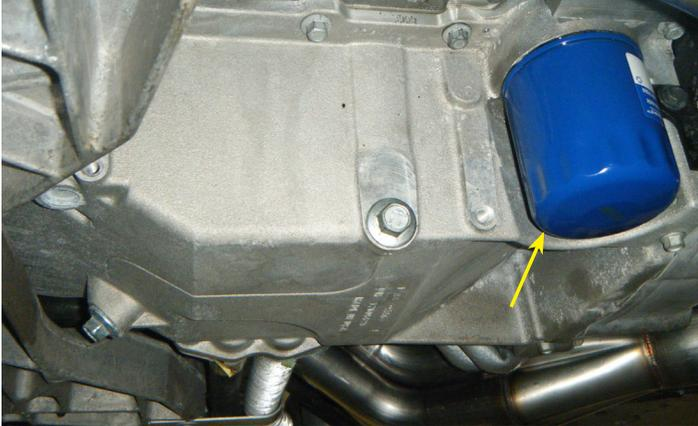
4. Allow all oil to drain out of the oil pan. Remove the oil filter by turning it counter clockwise by hand or using an oil filter wrench.
