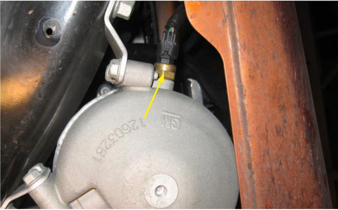
14. On the bottom of the tank remove the oil temperature sensor by first disconnecting the harness and then unscrewing the sensor using a 19 mm wrench. Inspect the sensor for damage as you will be using this sensor again.
