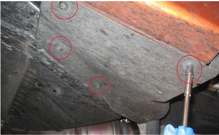
39. Using 7 mm and 10 mm sockets, replace the four (4) bolts that were removed from the fender liner.
