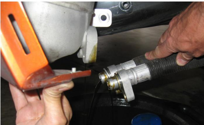
17. Move the bottom of the tank out of the way and remove the oil lines. Be sure to point the lines into the oil pan as residual oil will most likely drain out.
