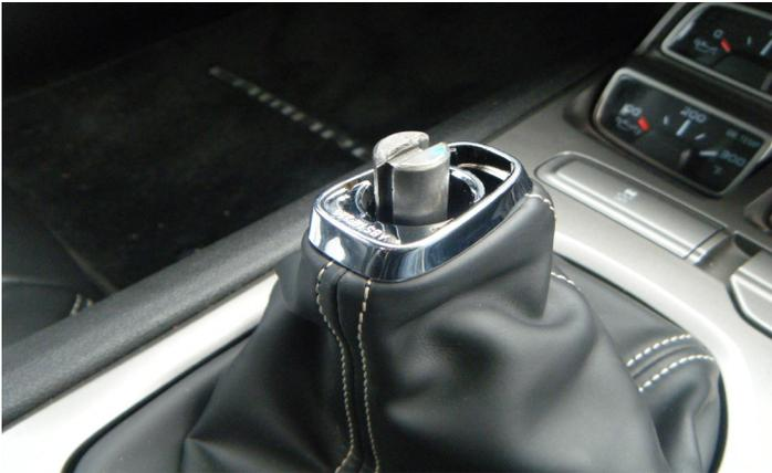
2. Gripping the shift knob above the chrome collar with both hands, pull upward to remove the shift knob.
