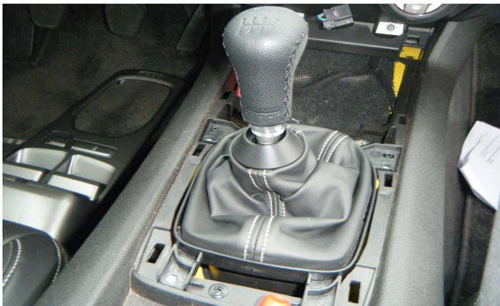
11. Place the LPE shift knob boot adapter onto the gear lever with the tapered end pointing up. Then push the shift knob onto the shift lever. The shift knob should bottom out on the shift lever when the shift knob is adequately pressed on.
