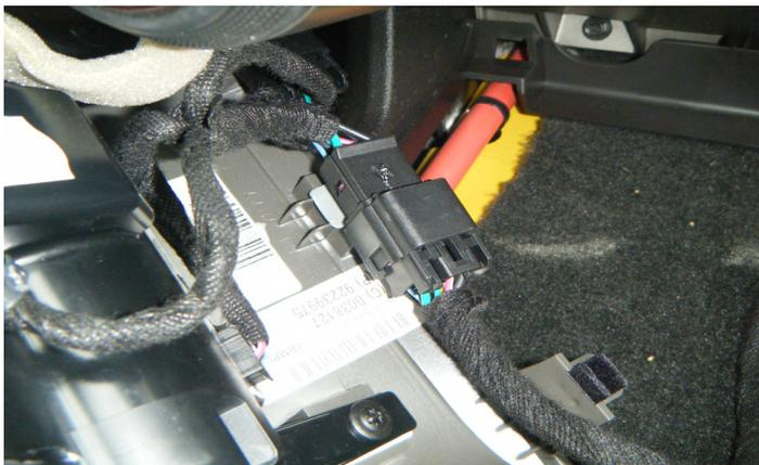
15. Reconnect the electrical connector on the back of the front floor console front cover.
