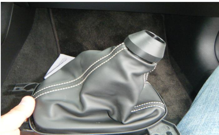
7. After flipping the shift boot back to its normal orientation, work the LPE shift boot collar into the shift boot as shown in the adjacent picture. The tapered end of the new collar should be pointing up.
