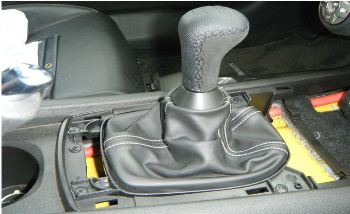
14. Orient the shift boot to its proper position. The shift boot can be rotated around the collar, even with the zip-tie already installed. Then using a Phillips head screwdriver, reinstall the four (4) shift boot mounting screws.
