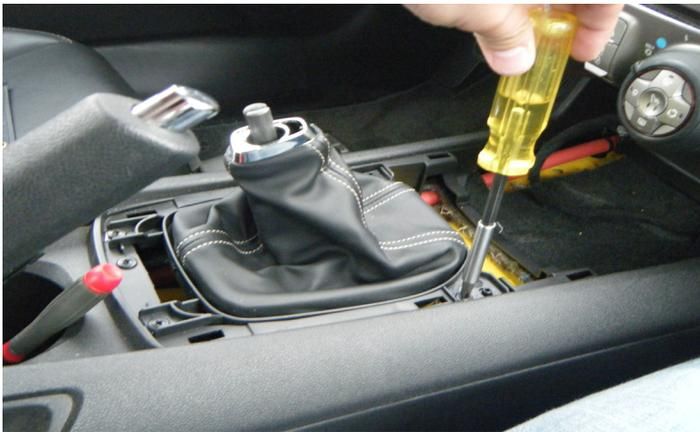
5. Using a #2 Phillips screwdriver, remove the four (4) shift boot mounting screws. The shift boot can now be removed.
