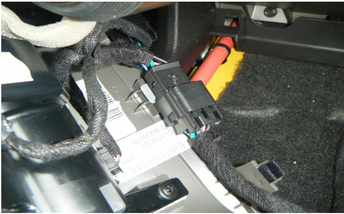
4. Disconnect the electrical connector on the back of the front cover. The front floor console front cover can now be removed and set aside.
