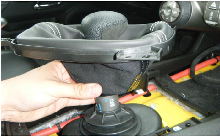
13. Screw the LPE shift knob boot adapter onto the shift knob. The tapered surface of the collar can be difficult to get ahold of, so it may be necessary to screw on the collar from the inside of the shift boot, as shown in the adjacent picture.
