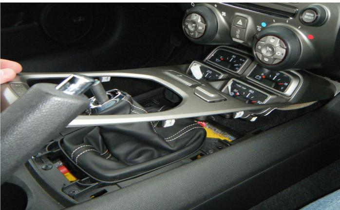
3. Using a small flathead screwdriver, plastic pry tool, or your fingers, gently pry up on the end of the front floor console front cover. Work your way around the front cover until the front cover completely separates from the floor console, taking care not to damage the plastic console or the retaining tabs that hold it down.
