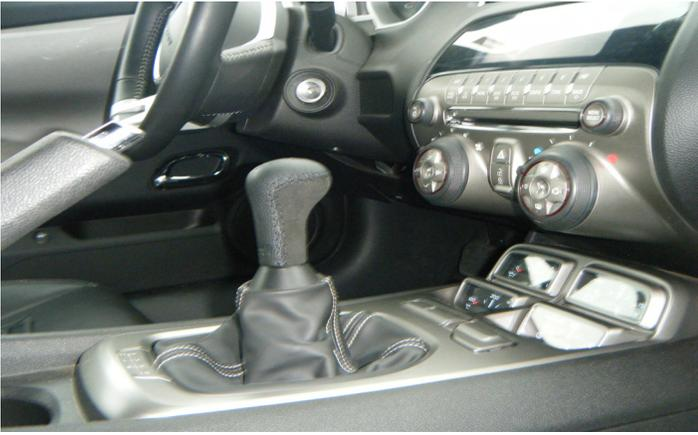
16. Reinstall the front floor console front cover by placing the end with the gauges in first. As you lower the other end of the front cover into place, gently press down on the front cover to re-engage the retainer tabs.
