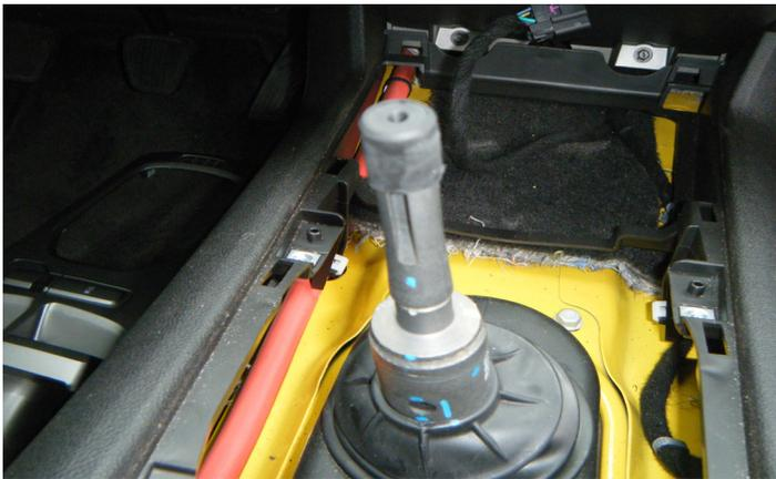
9. Select the rubber shift knob adapter with the largest inside diameter and install it onto the end of the shift lever.
