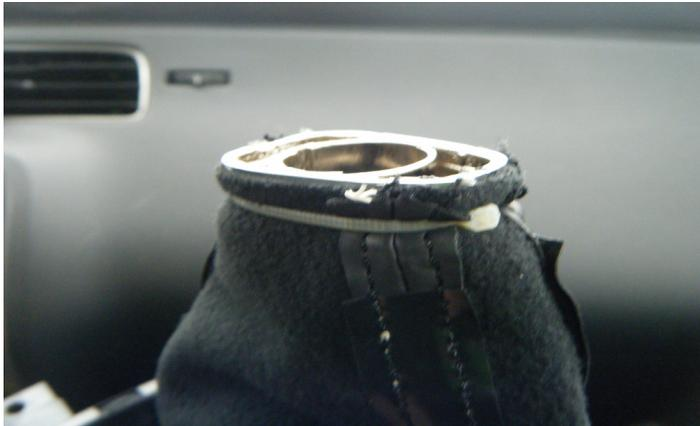
6. Flip the shift boot inside-out. You will see a zip-tie that holds the shift boot to the chrome collar. Using a knife or equivalent, remove the zip-tie, taking special care not to damage the shift boot.
