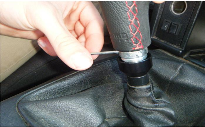
6. Push the shift knob onto the shift lever until it bottoms out. Applying constant downward pressure on the shift knob, tighten the three (3) set screws in a uniform manner to secure and center the shift knob onto the gear lever.
