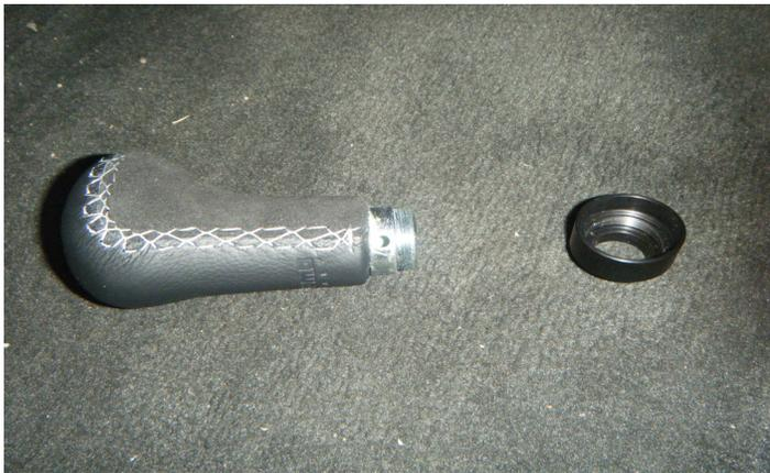
2. Remove the black threaded ring that is screwed onto the end of the LPE shift knob.
