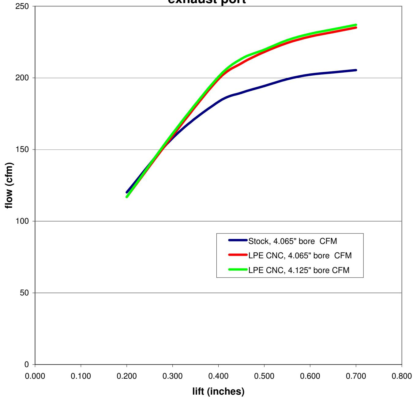
\*Flow differences are purely from the flow fixture bore size difference. The same CNC program/the same head/cylinder was tested on both bore sizes.
