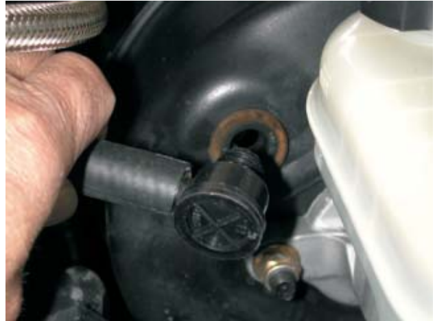
83. Disconnect the power brake booster vacuum line at the power brake booster by pulling the check valve out of the grommet.
