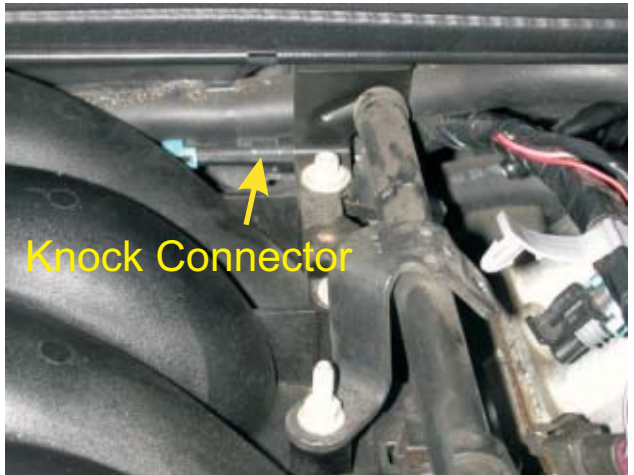
84. Remove the knock sensor wire harness connector from the (PCV) tube and unplug.
