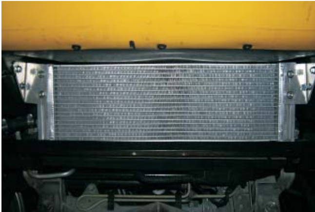
37. Here is the heat exchanger bolted in position with the hoses installed.
