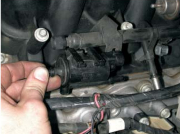
81. Remove the (EVAP) canister solenoid and mounting bracket.
