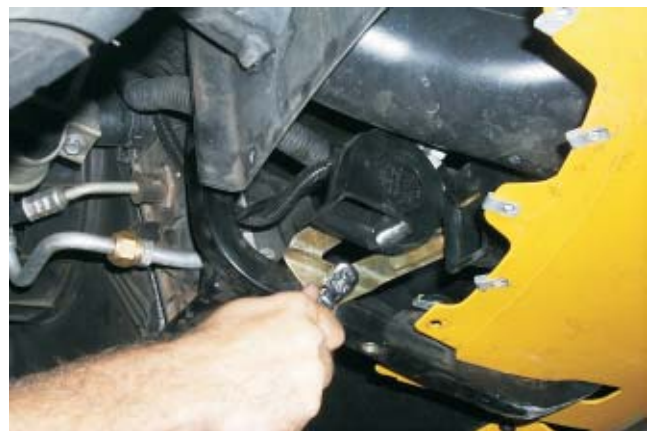
40. After removing the right hand splash panel, remove the horn assembly by unbolting it's mounting bracket with a ratchet and 13mm socket. Pull the assembly free then disconnect it's electrical connection.
