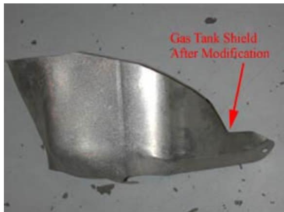
Mark the inner fender liner as shown; this will be your wire routing. Remove the gas tank shield and cut with tin snips. Use the supplied, pre-cut black piece of edge protector (part #30) on the shield, this must be installed to prevent cutting of the battery cable. Remove the inner fender liner and cut as marked. Install the gas tank shield but leave the fender liner out for now. For the LPE minitub kit, cut a notch of the same width and height in approximately the same location shown here.
