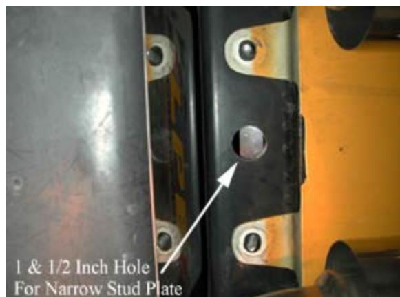
Find the black narrow stud plate that has two 5/16" bolts welded to it (part #8), insert it into the 1 ½ inch hole and drop the studs through the fascia mounting holes. (Needle nose pliers can make this easier.)
