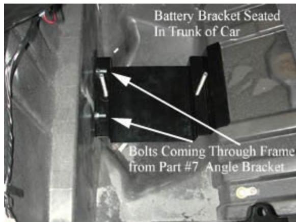
Drill 21/64 inches through the two holes on the bracket through the fiberglass; make sure carpet is out of the way. Place the black battery tray with 4" studs (part #4) in the fiberglass tub. It should be lined up with the holes you have drilled. From the exterior, install 5/16" x 3/4 serrated flange bolts and put nuts on battery tray side, then snug, but do not tighten the nuts.
