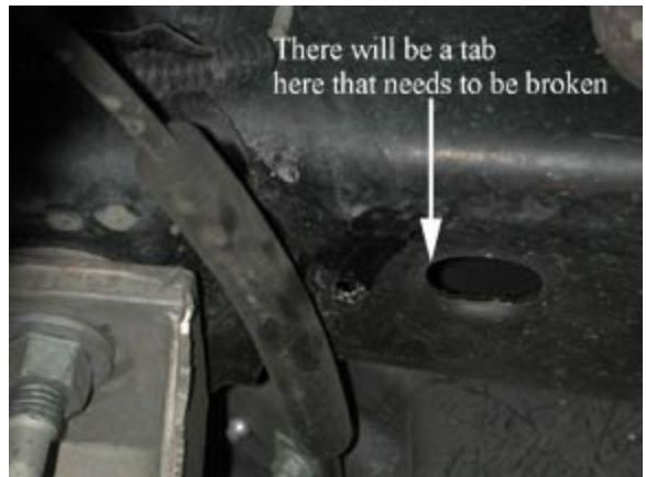
On the frame rails directly behind the hole you just drilled, you will see that the slotted hole still has the punched slug still attached to it. You will need a Phillips screwdriver to pry it over. Now go through your 21/64 inches hole with the Phillips screwdriver and push it the other way. Work it back and forth until it breaks off.
