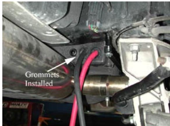
From outside of the car, route the round end of the positive (red) cable (part #3) through the 1" hole in the fiberglass panel that is located towards the front. Spray a large grommet (part #21) with WD40 and from inside the car, force it over the cable end and work it into place on the fiberglass. Repeat with the negative cable (part #4).
