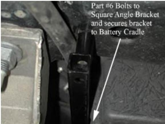
Center the battery tray in tub. Then drill 21/64 inches through the two holes in the front of the battery tray. Locate the black angle bracket with four slots (part #6). Using two 5/16"x18"x 3/4" (part #17) serrated flange bolts, install the bracket from underneath the car. The horizontal leg of the angle bracket should be to the bottom. Install 5/16 inch nuts (part #18) from inside the car, make these nuts snug, but do not tighten.
