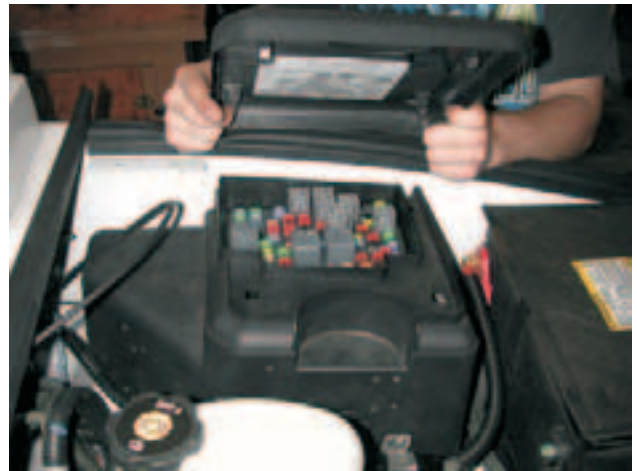
121. Reinstall the fuse / relay cover by aligning it up and pushing down on it.
