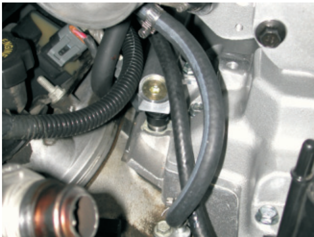
64. Connect throttle body to cylinder head manifold coolant hose.
