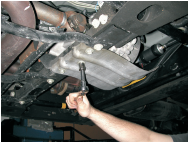
118. Using a 15mm socket wrench reinstall the rock / skid plate to the chassis.
