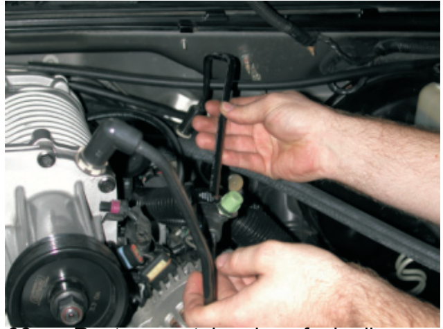
66. Route evap tube along fuel rail on drivers side. Re-connect to fitting on back of engine, route under supercharger nose.
