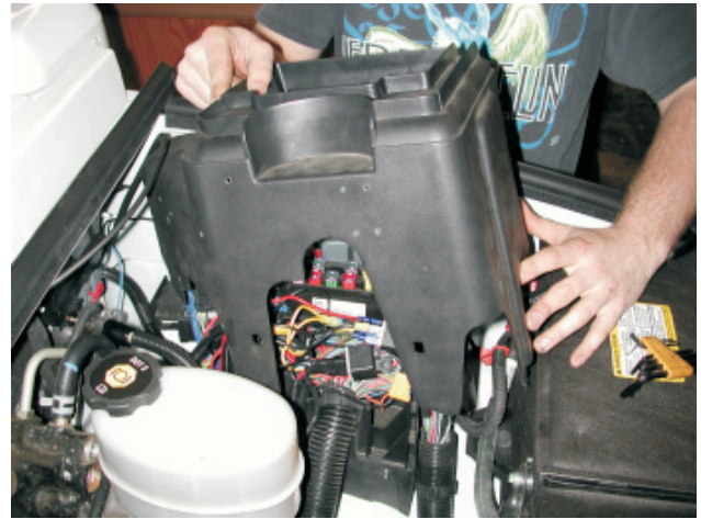
120. Reinstall the relay center cover. ( Be careful not to pinch any wires).
