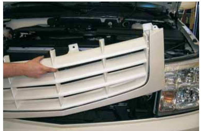
139. Remove the grille assembly.
