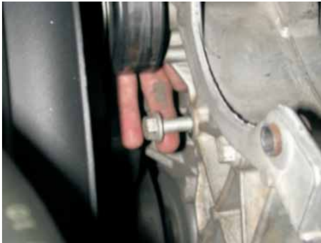
97. Remove the one bolt directly below the alternator and factory GM idler with a 15mm socket wrench.
