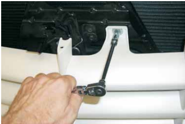
137. Remove the grille assembly by first removing the upper retaining bolt with a 10mm socket wrench.
