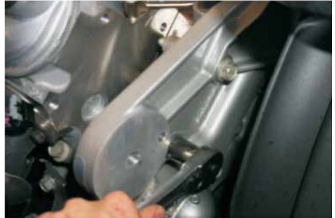
99. In the original tensioner location, install the new tensioner support bracket. Torque all mounting fasteners to 40 lb-ft.
