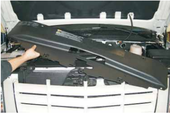
136. Remove the radiator cover.
