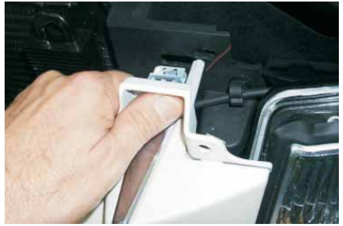
138. Pull out on the grille assembly at the corners to release the snap-in fasteners.
