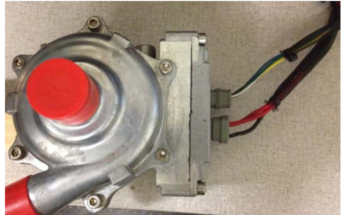
Wire routing provides a path for water to flow down into connector
