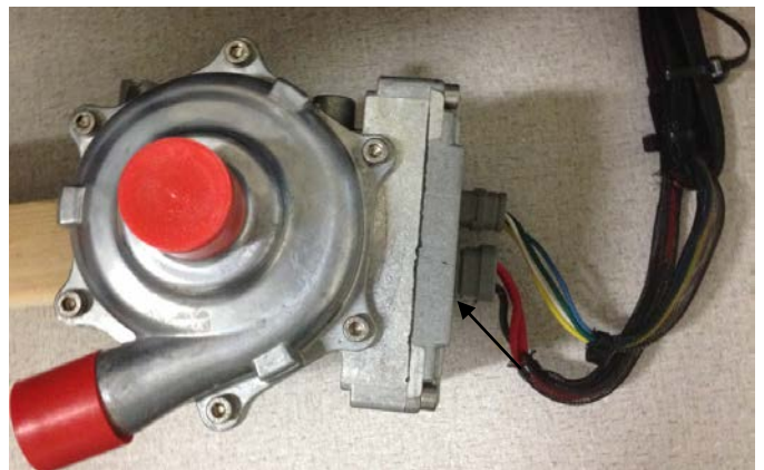
Drip loop collects water and sheds it away from connectors
