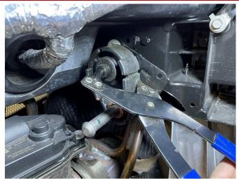
21. Remove both of the front exhaust grommets from the hanger on the chassis side of the connection using grommet pullers or similar device. The use of a soap and water solution will aid in the removal of the hangers from the factory grommets. The factory exhaust can now be lowered on the jack stand just enough to access the AFM valve actuator wiring connections.
