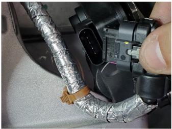
12. Reconnect the wiring connectors to both of the AFM valve actuators. Push in the grey locking tabs on the wiring connectors to secure the connections.
