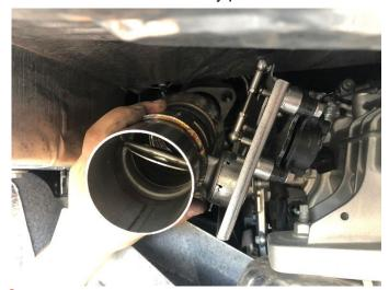
9. Locate the two M10 nuts set aside in Removal Step 19. Insert the driver side CORSA head pipe assembly onto the studs from the catalyst as shown, then hand tighten the M10 nuts to hold the head pipe in place, leaving the nuts loose enough that the head pipe can still pivot and rotate.
