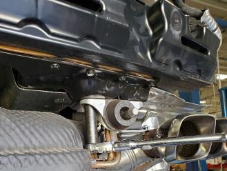
**18.** Support the factory exhaust with a jack stand. Remove the four bolts that secure both of the rear exhaust grommets to the chassis using a 13mm socket and 3/8" ratchet. Set aside the fasteners in a protected location.
