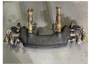
**23.** CAREFULLY slide the factory exhaust down and rearward to free it from the vehicle.
