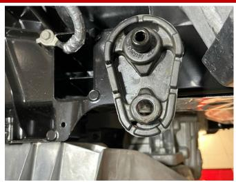
**18.** (ALL VERSIONS) Locate both front grommets set aside in Removal Step 24. Reinstall both of the front exhaust grommets onto the hangers on the chassis side of the connections. Make sure the larger sides of the grommets face upward as shown.
