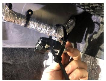
29. (FOR MUFFLER DELETE ONLY) Tuck the NPP valve wiring connectors up into the chassis, and secure with a zip tie.
