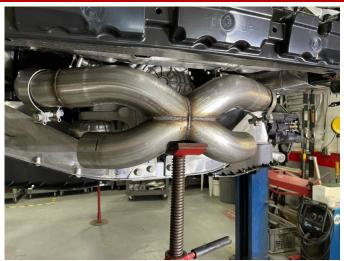
**15.** Adjust the rotation and overlap of the X-pipe assembly onto both of the head pipes until the X-pipe outlets are even both vertically and front to back in the vehicle. The X-pipe should be centered on the midline of the vehicle behind the rear differential.
