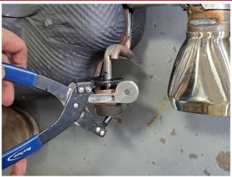
25. Remove both of the rear exhaust grommets from the exhaust hangers using grommet pullers or similar device. Note the orientation of the grommets for the installation of the CORSA exhaust system.
