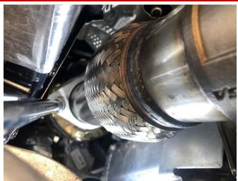
11. Next, secure the driver side cat back mounting flange to the factory catalyst using a 15mm socket, a 3/8" ratchet, and a 24" long extension. Torque to 32 FT-LBS.
