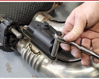
**26.** Remove the six bolts (3 per side) that secure both of the factory NPP valve actuators using a 10mm socket and a ¼" ratchet. Set aside the NPP actuators in a protected location. The NPP actuators will be reused on the versions of the CORSA exhaust that utilize a valved rear muffler configuration.
