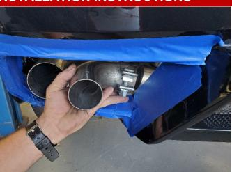
**33.** Locate one of the CORSA inner tip elbow pipes, and a 2.5" clamp from the hardware kit. Position the clamp on the elbow pipe inlet so the clamp bolt is facing towards the bend and the clamp nut is facing downwards. Insert the inlet of the elbow pipe onto the non-valved outlet of the driver side muffler with approximately 1.375" of overlap.
