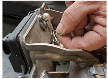
**27.** Remove four locking pins from both of the AFM valve actuator linkages.
