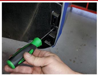
9. The inner fender liners are secured by eleven T15 TORX screws, four push clips, and three 7mm bolts per side. Starting on the driver side, remove the push clips first using a removal tool or flathead screwdriver, followed by the T15 TORX screws, and then the bolts using a 7mm socket and ¼" ratchet. This will free the inner fender liner from the vehicle.
