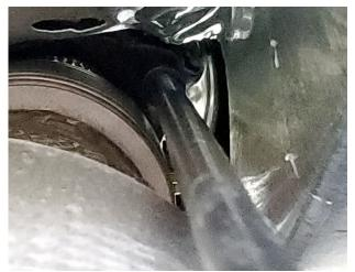
**20.** Remove the three M8 nuts that secure the passenger side cat back mounting flange to the factory catalyst using a 13mm socket, a 3/8" ratchet, and a 24" long extension. Set aside the fasteners in a protected location.
