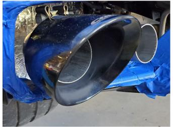
**35.** Locate one of the CORSA outer tip assemblies, and a 3" clamp from the hardware kit. Position the clamp on the tip inlet so the clamp bolt is on top of the tip and the clamp nut is facing inwards. Insert the inlet of the outer tip assembly onto the elbow pipe with approximately 1.5" of overlap.
