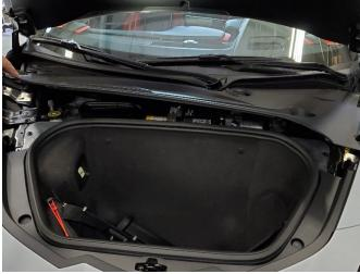
Unclip the front trunk battery cover panel and remove from the vehicle. Set aside the panel in a protected location.
