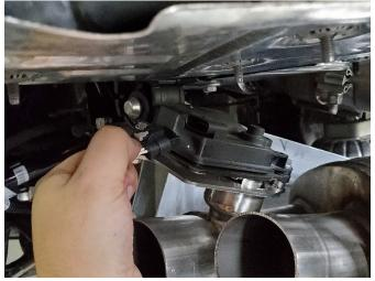
27. (FOR NPP VALVED MUFFLER ONLY) Connect the opposite end of the wiring extensions to the NPP valve actuator on both sides of the vehicle. Push in the grey locking tabs on the wiring connectors to secure the connections.
