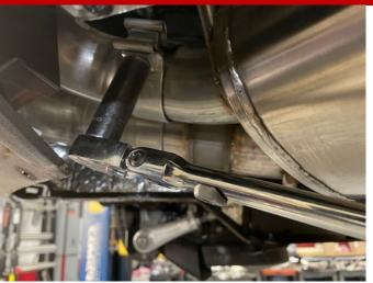
**34.** Rotate the CORSA inner tip elbow pipe until it is centered in the rear valence, then tighten the exhaust clamp at the elbow pipe inlet using a 15mm socket and 3/8" ratchet.
