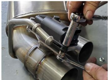
17. (FOR NPP VALVED MUFFLER ONLY) Locate the two CORSA NPP Compatible Muffler assemblies, and the two stock NPP valve actuators set aside in Removal Step 26, along with the remaining six supplied M6 bolts and M6 nuts from the hardware kit. Align and secure both of the factory NPP valve actuators to the CORSA NPP valve assemblies using a 10mm socket, a ¼" ratchet, and a 10mm wrench. Torque to 89 IN-LBS.
