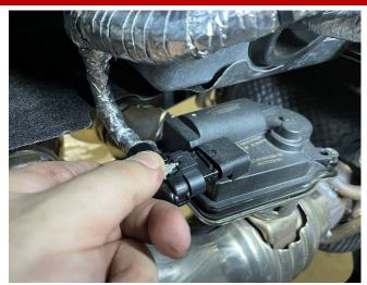
17. Disconnect the wiring connectors to both of the NPP valve actuators; these are located on the pipes leading to the outer exhaust tips. Note that the grey locking tab on the wiring connectors must be slid outwards before disconnecting the wires from the actuators.
