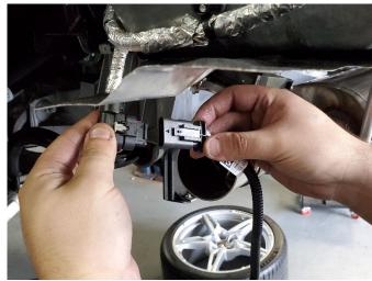
**26.** (FOR NPP VALVED MUFFLER ONLY) Locate both NPP valve wiring extensions from the hardware kit. Connect both wiring extensions to the chassis side of the NPP valve wiring connectors. Push in the grey locking tabs on the wiring connectors to secure the connections.
