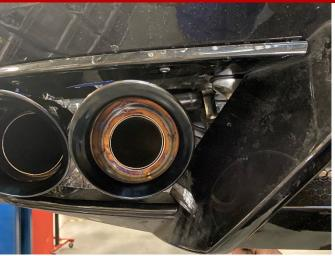
**38.** Adjust the rotation of the CORSA inner tip assembly until the CORSA logo is centered on the top of the tip, then tighten the exhaust clamp at the tip inlet using a 15mm socket and 3/8" ratchet.
