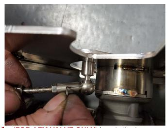
(FOR AFM VALVE ONLY) Locate the two CORSA AFM valved head pipe assemblies, and the two stock AFM valve actuator linkages and four locking pins set aside in Removal Steps 27 & 28. Connect both of the AFM valve actuator linkages to the CORSA AFM valve assemblies. Secure the connections with the locking pins.
