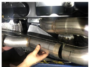
20. Position the clamp on the CORSA driver muffler (or muffler delete) inlet so the clamp bolt is in front of the expansion and the clamp nut is facing downwards. Insert the inlet of the driver muffler/muffler delete assembly on to the driver side outlet of the X-pipe with approximately 1.75" of overlap.
