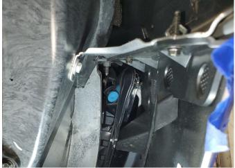
11. The sides of the rear bumper cover are secured to the fender by a 10mm nut and two 7mm bolts on each side. Starting on the driver side, remove the nut first using a 10mm socket and 3/8" ratchet, followed by the two bolts using a 7mm socket and ½" ratchet.
