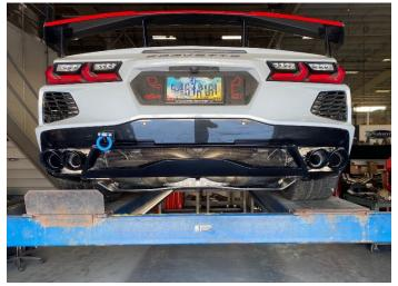
**40.** At this time, adjust the tip tube and tip positions until all tips are centered within the cutouts in the rear valence, and there is approximately ½" reveal at the CORSA logo of each tip. Torque all exhaust clamp bolts to 45 FT-LBS.
