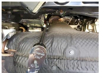
**19.** Remove the two M10 nuts that secure the driver side cat back mounting flange to the factory catalyst using a 15mm socket, a 3/8" ratchet, and a 24" long extension. Set aside the fasteners in a protected location.
