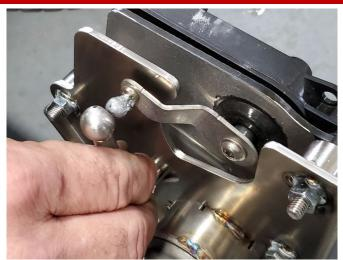
**3.** (FOR AFM VALVE ONLY) Connect both of the AFM valve actuator linkages to the factory AFM valve actuators. Secure the connections with the remaining locking pins.
