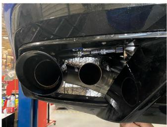
**36.** Adjust the rotation of the CORSA outer tip assembly until the CORSA logo is centered on the top of the tip, then tighten the exhaust clamp at the tip inlet using a 15mm socket and 3/8" ratchet.
