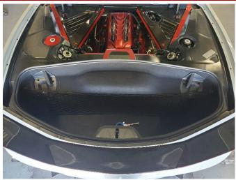
13. Remove the sixteen T15 TORX screws that secure the top of the factory rear bumper cover to the chassis. Start with the fourteen screws that run along the top edge of the bumper.
