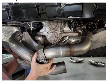
13. Locate the CORSA X-pipe assembly, and two 3" clamps from the hardware kit. Position the clamps on the X-pipe inlet, so the clamp bolts are on the outside of the expansion and the clamp nuts are facing downwards. Insert the inlet of the CORSA X-pipe assembly on to the outlet of both head pipe assemblies with approximately 1.75" of overlap.
