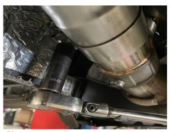
**32.** Rotate the CORSA outer tip elbow pipe until it is centered in the rear valence, then tighten the exhaust clamp at the elbow pipe inlet using a 15mm socket and 3/8" ratchet.
