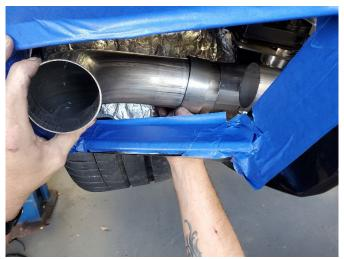
**31.** (ALL VERSIONS) Locate one of the CORSA outer tip elbow pipes, and a 3" clamp from the hardware kit. Position the clamp on the elbow pipe inlet so the clamp bolt is facing away from the bend and the clamp nut is facing downwards. Insert the inlet of the elbow pipe onto the valved outlet of the driver side muffler with approximately 1.75" of overlap.
