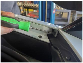
14. Remove the last two T15 TORX screws that are facing rearward and tucked into the corner of the fender on each side. This will allow the bumper cover to move independently from the vehicle. Set aside the fasteners in a protected location.
