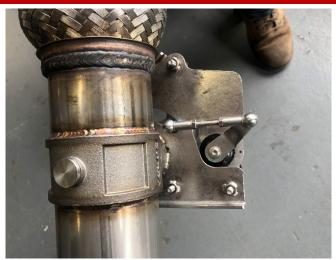
4. (FOR AFM VALVE ONLY) The AFM valve actuators should now be connected to the CORSA AFM valve assemblies as shown.
