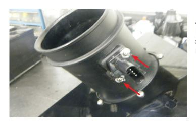
10. Using the two (2) supplied #14 screws and a phillips head screwdriver, secure the stock MAF sensor to the MAF housing. The screws should be tightened until the washers touch the metal surface on the MAF sensor.
