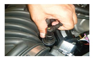
6. By pressing the retaining tab, disconnect the breather tube that connects the air intake tube to the driver-side valve cover.
