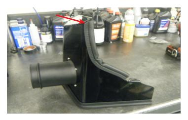
12. Firmly push the supplied shorter edge seal with the angle cut on one end onto the bottom of the airbox. The angle cut in the edge seal should be pointed down when the airbox gets installed into the vehicle, as shown by the arrow.
