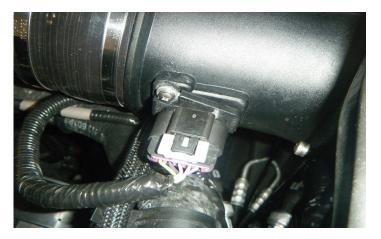
20. Connect the MAF sensor harness connector to the MAF sensor housing. You should hear a click when the connector is fully engaged. Slide the grey tab to lock the MAF sensor connector in place.
