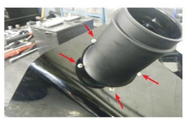
9. Using a phillips head screwdriver, insert the supplied MAF housing through the hole in the supplied airbox. Using the five (5) 10-32 screws, secure the MAF housing to the airbox. The screws should be tightened in a star pattern with the screw behind the MAF sensor being the first to be tightened.
