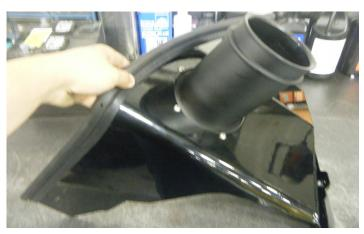
11. Firmly push the supplied longer edge seal onto the top of the airbox.
