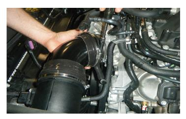
18. Rotate the inlet elbow clockwise until it can be connected to the throttle body. Connect the hump hose to the throttle body. Disengage all four (4) of the worm clamps and place the clamps over the narrow parts of the hump hoses. Using an 8mm socket, secure the hump hoses. Do not overtighten.
