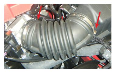
4. Loosen the hose clamps holding the air intake tube to the throttle body and airbox using an 8mm socket.
