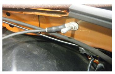
21. Using a 10mm socket, remove the ground stud located on the front driver-side corner of the engine compartment.
