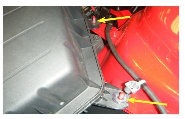
5. Remove the two (2) nuts that hold the airbox in place using a 10mm deep socket.
