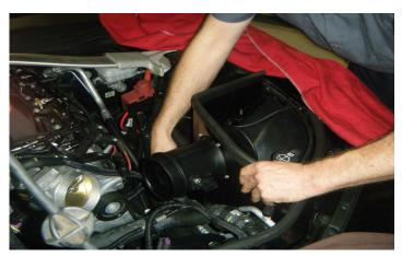
13. Lower the airbox assembly into lowering the airbox onto the bottom grommet and the upper stud as shown the illustration. Firmly push down on the airbox to verify that the airbox is fully seated onto the grommet.
