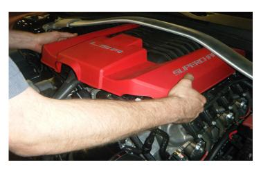
2. Remove the engine cover by pulling the front of of the cover up and away from the engine.
