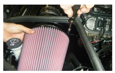
23. Carefully install the supplied air filter onto the MAF housing inside the airbox. If the airbox flange nut was left loosened, you can move the airbox slightly towards the passenger side of the vehicle to make installation of the air filter easier. Secure the air filter to the MAF housing using the large supplied worm clamp and an 8mm socket. Do not overtighten.
