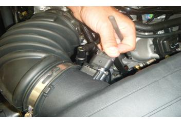
3. Unplug the Mass Air Flow (MAF) connector, which is located on the side of the airbox inlet, by first sliding the grey tab to unlock the connector. Then, press on the center tab and pull the connector away from the airbox inlet.
