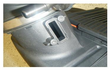
8. Using a 7mm socket, remove the two (2) screws that secure the MAF sensor to the airbox. Make sure to keep the stock MAF sensor as it will be re-used for the new air intake installation.
