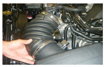
7. Remove the air inlet tube from the throttle body and pull up on the airbox to remove the air inlet tube and airbox.
