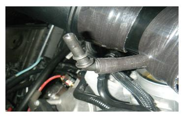
17. Insert the supplied 45 degree breather hose adapter into the supplied hump hose with built-in breather. Clock the adapter so that it points straight up, as shown in the picture.
