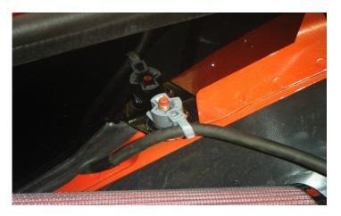
24. Tighten the airbox flange nut and then attach the ground wire guide back onto the upper stud as well.
