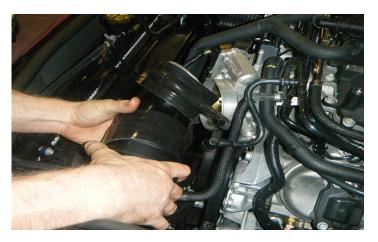
16. Work both hump hoses onto the inlet elbow. The hump hose with the built-in breather will connect the inlet elbow to the throttle body while the other hump hose will connect the inlet elbow to the MAF sensor housing. To make installation easier, connect the inlet elbow to the MAF sensor housing and point the other end of the elbow upward, as shown in the picture. If necessary, silicon lubricant can be applied to the inside of the hump hoses to make the assembly easier to adjust.
