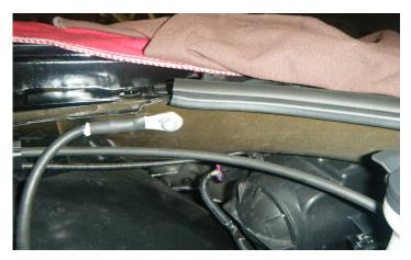
22. Using a 10mm socket, install the supplied ground bolt allowing additional clearance for the air filter. Torque the bolt to 89 in-lbs.
