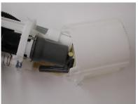
4) Using a small pocket screwdriver, carefully pry the fuel sock (fuel pump inlet filter) from the center pin on the bottom of the fuel pump. Save the fuel sock. You will be reusing the fuel sock when you reassemble the module.
