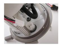
3) Carefully remove the outer "bucket" from the fuel pump module assembly.
