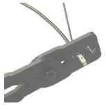
19) Using a pin tool, remove the original wires from the white connector that attaches to the bulkhead connector on the top of the module. Note which wire is in which cavity (red should be closest to the latch).
