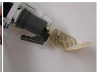
5) Using wire cutters, clip the small ground wire as close to the fuel pump terminal as possible.
