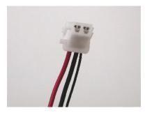
22) Reconnect the white bulkhead connector to the mating connector on the top of the fuel pump module.
