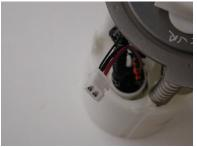
23) Follow the GM service instructions to reinstall the fuel pump module, using the supplied replacement fuel sender module O-ring (GM part # 22682111).
