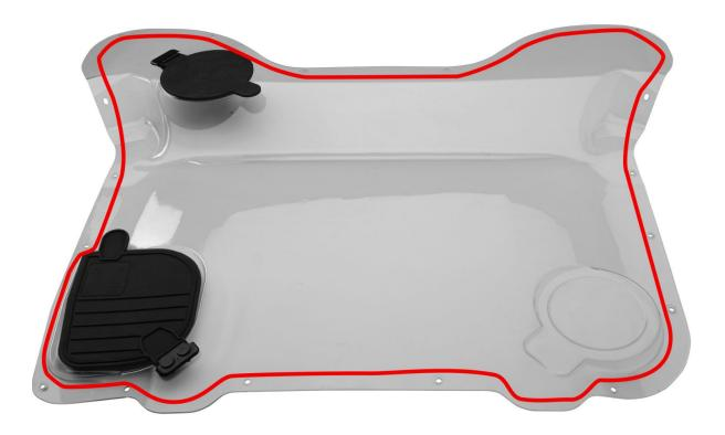
Place the 14 double sided grommets into the the mounting holes where the OEM cover was on the car. (For this step, these are placed on the car, not the clear cover)
