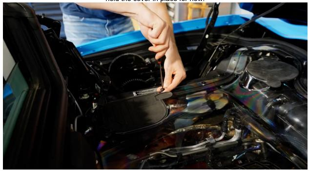
Install the 4 single sided grommets. These can be a little tricky. Gently lift the corners of the clear cover on the upper backside and slide the single sided grommets under the cover into position one by one. The flat portion of the grommet will rest on the car and the top will rest inside the hole of the cover. As you place them, lightly thread the OEM hardware into each, only a few threads, just enough to secure the grommets from slipping out of place. Refer to the diagram below.
