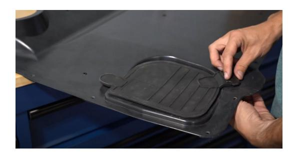
Install the access flaps onto the Clear Engine Cover
