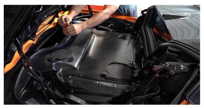
Using a 10mm socket, remove the access flaps from the OEM Engine Cover
