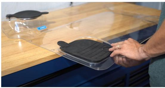
Apply the adhesive seal around the Clear Engine Cover. Follow around the mounting holes with the seal on the inside of them.
