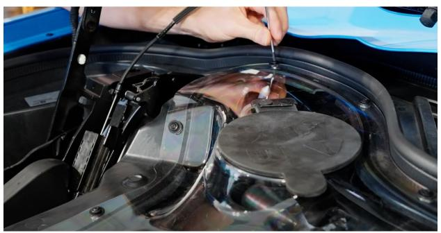
Once all 4 of the single sided grommets are in place go back around the perimeter of the cover and fasten all 18 bolts to secure the cover in place. Do not use power tools as over-torquing the bolts may cause damage to the cover. Once you have ensured that all 18 bolts are secure installation is complete.
