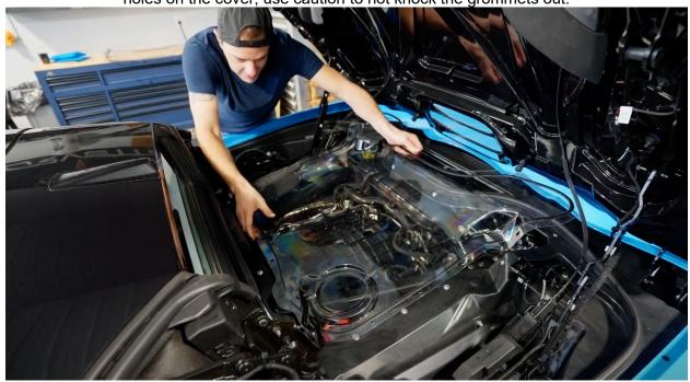
Lightly fasten a few of the bolts utilizing the OEM hardware removed from the stock cover. Just tight enough to hold the cover in place for now.
