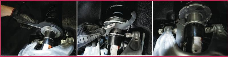
The Lingenfelter Spanner Wrench is precisely designed for use on C8 Corvettes and is a must for performance enthusiasts to optimize handling for track days. With its precisely engineered size and ergonomic shape, the C8 Spanner Wrench offers a comfortable grip, maximum leverage and clearance for adjusting the shock spanners to desired rideheight. The tool has also been designed to store neatly in the recess located in the glovebox under the owners manual.
