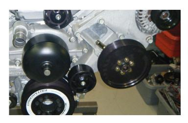
3. Install the supplied power steering and alternator pulleys on the vehicle. Also install the new water pump and damper on the vehicle using the factory GM torque specifications. DO NOT RE-INSTALL THE IDLER AT THIS TIME.
