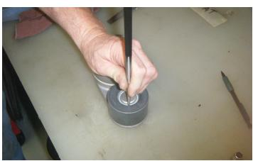
9. Using a hammer and a punch, remove the dust cap from the idler.
