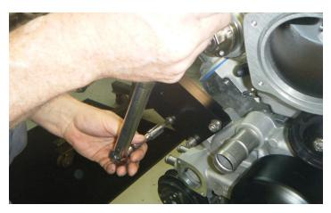
7. Torque the support bolt to 35 ft-lbs.
