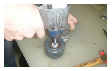
10. Using an impact gun, remove the idler bolt from the front of the pulley and remove the pulley. The stock pulley and dust shield will not be reused.
