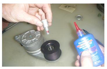
13. Place the pulley on the tensioner. Apply a small amount of Loctite on the tensioner pulley bolt.
