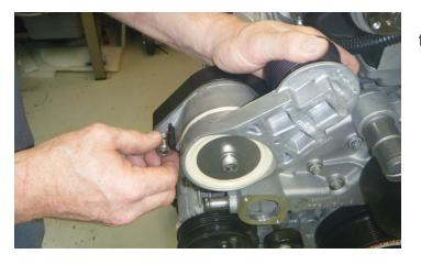
15. Install the two (2) tensioner bolts into the tensioner bracket.
