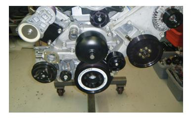
18. Top idler pulley (on front jackshaft bracket) uses M10x1.5x70 stainless socket head cap screw and 0.450" pulley locator behind the 90 mm idler pulley. The lower idler pulley (on the alternator bracket) uses the M10x1.5x60 stainless socket head cap screw and the 0.350" pulley locator.
