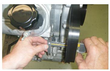
5. Using a set of calipers, measure the air gap between the head and the bracket. If the space between them is larger than 2.395" then you may need to used the supplied shims to make up the difference. If the gap is smaller than 2.395" you may need to take material off of the spacer. DO NOT TIGHTEN THE BOLT TO MAKE UP FOR THE GAP.
