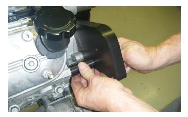
6. Using the supplied M10x1.5x90mm bolt, install the bracket support between the head and the tensioner bracket.
