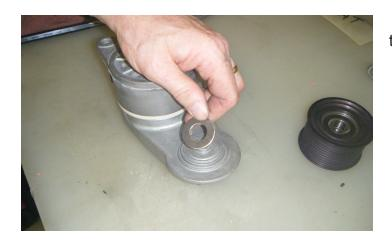
12. Install the supplied 10mm washer onto the tensioner in the position shown.
