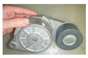
8. You will now need to remove the factory idler pulley and install a ribbed pulley.
