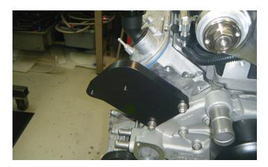
4. Install the LPE supplied 10 rib bracket onto the water pump. Torque the bolts to factory torque specifications.
