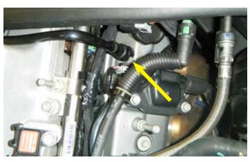
18. Disconnect the PCV fresh air hose line from the left side valve cover (at the rear of the engine).
