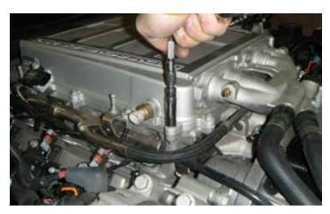
36. Starting with the back 6 bolts, remove the seventeen (17) 10 mm bolts on the supercharger cover with a socket and extension.
