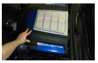
132. Re-install the engine sight shield (engine cover) by pushing down on the cover to secure it to the mounting posts.
