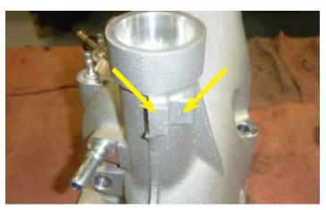
68. If you are using a 2.55" or smaller pulley, you will need to partially remove the fixturing tabs on the casting of the front cover shown to the left.
