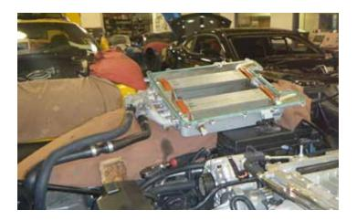
39. With the intercooler fluid lines still connected to the cover, put the cover off to one side of the engine compartment and cover with a plastic bag or rags to prevent dust and debris from getting into the cover.
