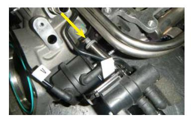
57. Remove all vacuum hoses from the bypass valve actuator and boost control solenoid. Using a 10 mm wrench, remove the two (2) bolts securing the bracket as shown.
