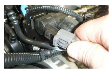
13. Disconnect the electrical connector from the boost control solenoid at the left front of the supercharger.
