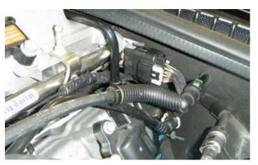
16. Disconnect the fuel injector and ignition coil harness connector from the driver side of the engine.
