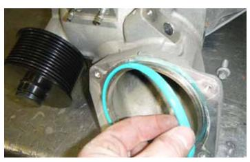
80. Re-install the throttle body gasket that you removed from the front cover.
