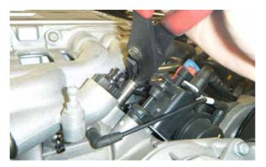
123. Connect the brake boost vacuum line to the supercharger front cover.
