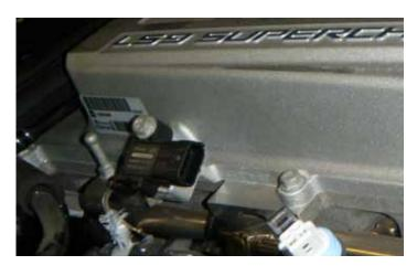
21. Disconnect the barometric (BARO) pressure sensor electrical connector on the right side (passenger side) of the intercooler.
