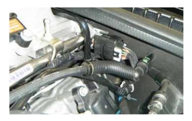
121. Connect the fuel injector and ignition coil harness connector on the driver side.
