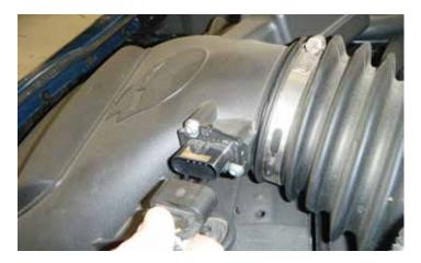
131. Connect the mass air flow sensor connector.
