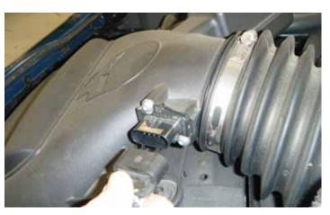
4. Disconnect the mass air flow (MAF) sensor electrical connector located at the air inlet duct.
