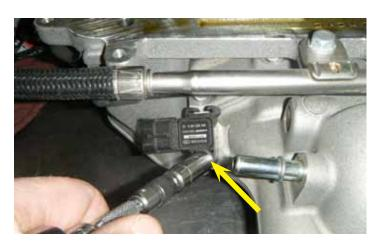
55. Using a 10 mm socket, remove the bolt to the inlet air pressure sensor from the supercharger front cover.
