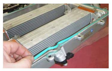
40. Inspect the supercharger cover seal. Replace if damaged. [GM PART #12613457].
