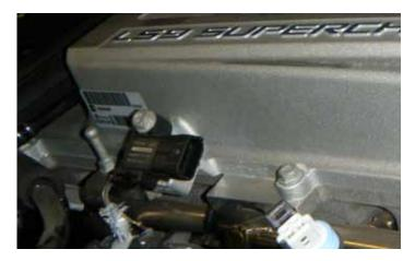
119. Connect the barometric pressure sensor electrical connector.
