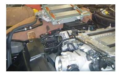
97. With the help of an assistant, place the supercharger assembly back in place on the engine. Align the dowel pin at the right front of the supercharger to the cylinder head.
