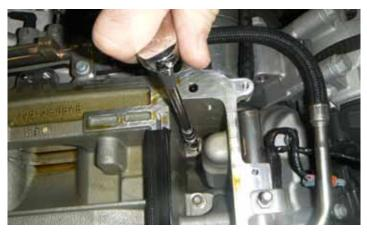
98. Torque down the ten (10) supercharger bolts, refer to the next step for the torque pattern and specifications.
