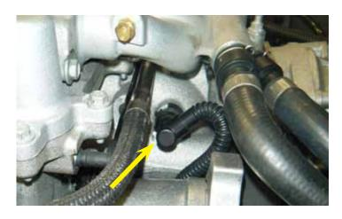
101. Connect the PCV dirty air hose line to the passenger side of the supercharger front cover.
