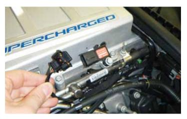
120. Connect the boost pressure sensor connector.
