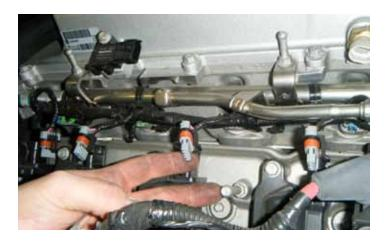
113. Connect the ignition coil electrical connectors to the ignition coils on both sides (8 coils).
