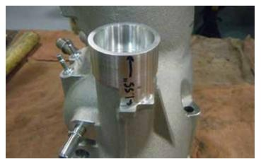
70. Using a runout gage, locate your end mill to be concentric with the inside of the jackshaft housing (you may also use the jackshaft itself to center the endmill). You can complete the machining with the jackshaft installed if your boring gage allows it, otherwise you will need to remove the jackshaft. If you remove the jackshaft, you must replace the bearings. See the next step for the dimensions of the machined part.
