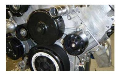
93. Place the supplied idler locating spacer on the back side of the idler. Place the supplied dust shield/cover on the front of the idler pulley. Put the supplied bolt through the idler and install the assembly on the engine.
