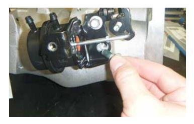
81. Using a 10 mm socket, torque the two (2) bypass actuator bolts to 18 lb-ft (25 Nm). If your front cover has been hand ported by LPE or someone else, the lower bolt hole may now be open to the inside of the cover and require thread sealant ( Loctite 567 thread sealant or equivalent) on the actuator bolts.
