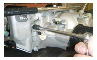
59. Using a 10 mm socket and extension, remove the six (6) bolts that secure the front cover to the supercharger assembly.
