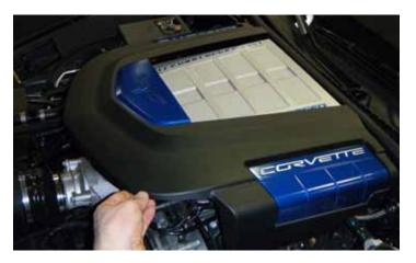
3. Remove the engine sight shield (engine cover) by pulling up on the cover to remove it from the three (3) mounting posts.
