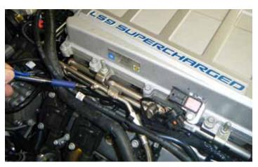
44. Bleed the fuel system pressure to 0 psi at the service test port on the driver side fuel rail.
