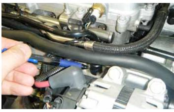
22. Disconnect the PCV fresh air hose line from the right valve cover (at the front of the engine).
