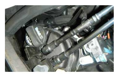
115. Connect the PCV fresh air hose assembly to the left and right valve covers and the dry sump tank.
