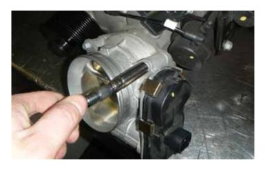
89. Install the throttle body on the supercharger front cover. Using a 10 mm socket, torque the four (4) bolts to 10 Nm (89 lb-in).
