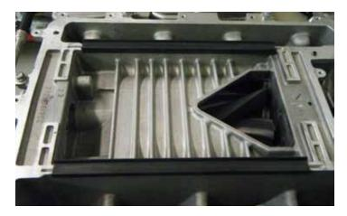
103. Install insulator seals on the supercharger assembly.
