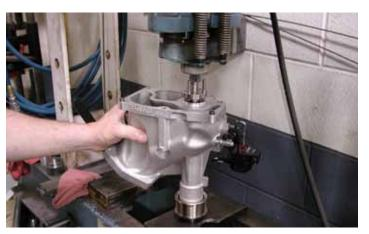
72. Place the LPE pulley on the bearing shaft, then use a machine press to press the new pulley on to the supercharger front cover until it is flush with the bearing shaft.
