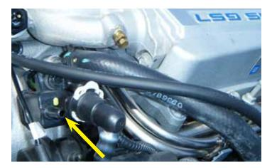
31. Disconnect the purge line from the purge solenoid on the driver side of the supercharger front cover.
