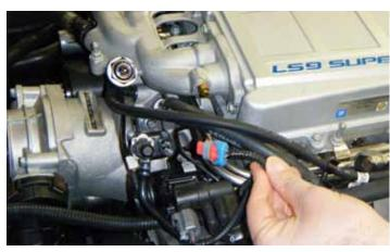
126. Connect the electrical connector to the EVAP purge solenoid.
