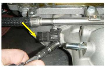
54. Disconnect the engine inlet air pressure sensor electrical harness.
