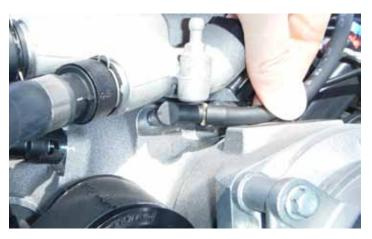
124. Connect the active exhaust vacuum hose to the supercharger front cover.
