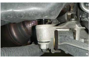
110. Using a 21 mm socket, tighten the four engine cradle stud nuts (two on each side) and torque to 110 Nm (81 lb-ft). You can now remove the jack from under the engine.
