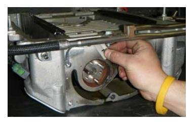
63. Inspect the cover mounting surface on the supercharger assembly. Clean off any remaining adhesive with a razor blade.
