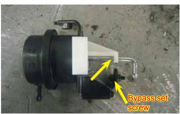
82. Use the set tool to set the actuator position [tool part # ETN86063]. Place the actuator set tool so that the actuator arm teeth are located in the position shown. Note the bypass set screw position.
