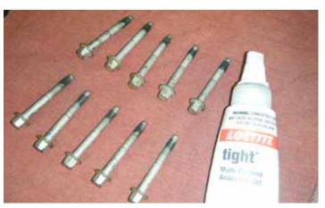
96. Apply a 5 mm (0.2 inch) band of threadlocker (Loctite Blue, GM PN 12345382 or equivalent) to the threads of the 10 supercharger bolts. Place the ten bolts into the supercharger.
