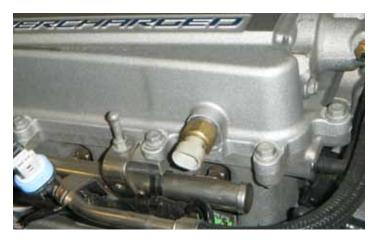
20. Disconnect the supercharger outlet air temperature sensor (IAT2) electrical connector from the sensor on the right side of the intercooler.
