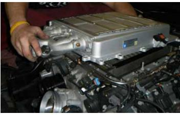
38. Remove the supercharger cover from the engine.
