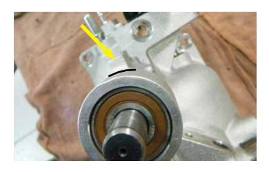
69. Start by marking both of the tabs with a black marker. Make sure that the you do not go below your mark in the machining process. LPE suggests using an adjustable boring head or a die grinder to remove material. Remove the tabs 1.55" down as illustrated in the next step.
