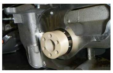
64. Install the supplied plastic isolator coupling on the pins on the shaft in the supercharger assembly. The holes are evenly spaced so it doesn't matter what set of holes you use. The new isolator coupling will be a tight fit on the pins.
