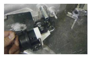
85. Tighten the set screw so that it barely touches the stop plate on the front cover. After the initial contact, tighten the set screw 1/8 to 1/4 turn *more* to set the bypass valve blade into position. The set screw should now be touching the stop plate on the front cover. This will prevent the bypass valve blade from getting stuck on the front cover casting. Remove the bypass actuator set tool.
