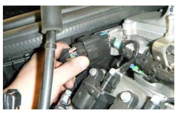
122. Connect the fuel injector and ignition coil harness connector on the passenger side.
