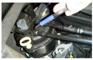
8. Disconnect the PCV lines from the dry sump oil tank.
