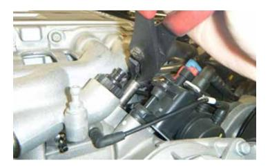
15. Disconnect the brake boost vacuum hose that routes from the left side of the engine compartment to the front of the supercharger.
