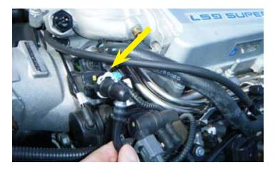
127. Connect the EVAP purge line to the purge solenoid.
