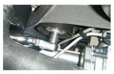
92. Due to the low clearance in the front of the engine compartment, it is recommended to use a flex-head ratchet for this part of the installation.
