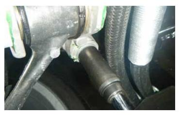
35. Loosen the engine cradle nuts and lower the engine assembly and cradle assembly approximately 1 inch down. You should still have several turns of engagement on the threads on each nut. Do not remove the nuts from the studs.
