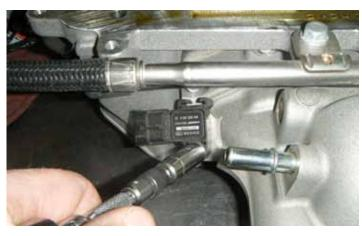
102. Connect the engine inlet air pressure sensor electrical harness.
