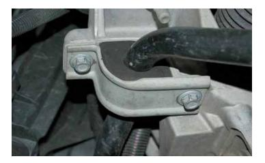
111. Using a 13 mm socket and the 6" extension, install the sway-bar bushing to cradle brackets and bolts on both the left and right side. Torque to 58 Nm (43 lb-ft).
