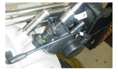
87. Install the purge solenoid onto the front cover. Using a 10 mm socket, torque the fastener to 10 Nm (89 lb-in).
