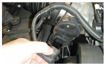
130. Connect the throttle actuator electrical connector.
