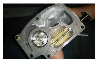
77. Apply a thin film of the supplied Permatex Ultra Black Gasket Maker to the LS9 cover flange surface.
