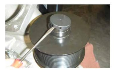
66. Remove the cap on the pulley by using a small flat head screwdriver and prying up.
