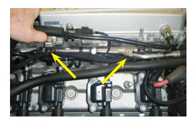
117. Re-attach the two (2) wiring harness fastener clips on the passenger side of the vehicle.
