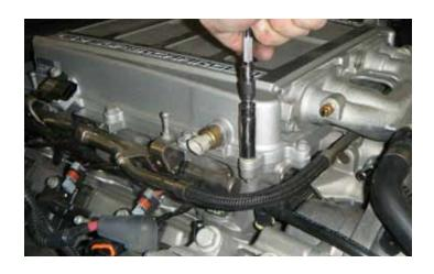
105. Install the seventeen (17) supercharger cover bolts and the supercharger cover.
