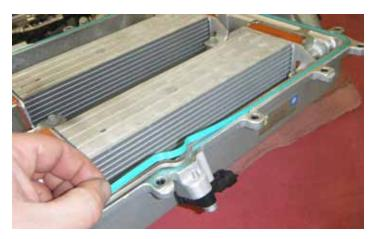
104. If you removed or are replacing the supercharger cover seal, install the supercharger cover seal.
