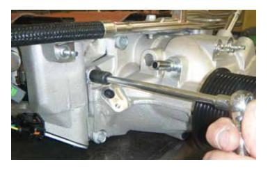
79. Install the six (6) cover bolts with a 10 mm socket and extension. Torque to 27 Nm (20 lb ft). The torque sequence is not critical on this component. With the plastic cover removed from the end of the shaft, tap the end of the shaft with a rubber mallet to seat the plastic shaft coupler. Check to make sure the supercharger assembly turns smoothly. If it doesn't turn freely, tap the end of the shaft again to fully seat the plastic coupler.
