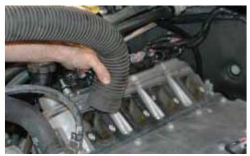
94. Make sure the cylinder head and engine area are free of loose debris.
