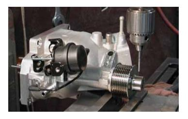
73. Using a drill press, secure the supercharger pulley so that it is clamped evenly and drill a 3/16" hole, 1.05" deep in the center of the end of the pulley. Next, using a 1/8" drill bit, drill a hole completely through the pulley and shaft in the same position. This will allow you to remove the pin if you are ever replacing or removing the pulley.
