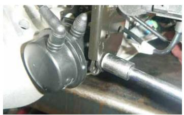
86. Install the boost control solenoid bracket assembly onto the front cover. Using a 10 mm socket, torque the fastener to 10 Nm (89 lb-in). Replace all vacuum hoses.
