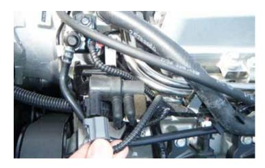
125. Connect the electrical connector to the supercharger boost control solenoid and connect evap hose to solenoid.
