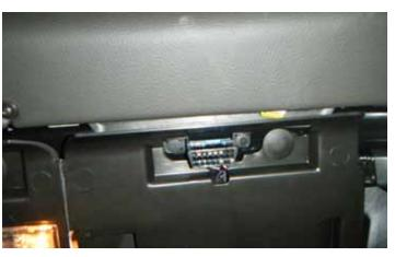
136. Install the supplied diagnostic port (DLC port) cover onto the DLC port in the driver foot well. Secure the strap that retains the DLC cover to the vehicle.
