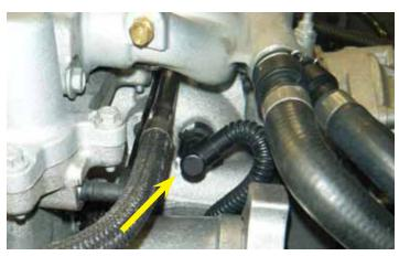
42. Remove the PCV dirty air hose line from the passenger side of the supercharger.
