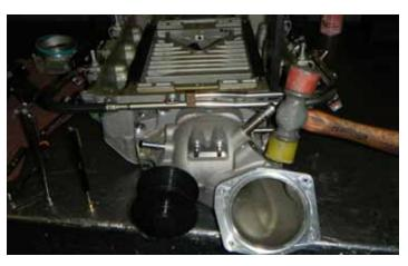
60. Using a rubber mallet and prybar, carefully knock the front cover loose from the supercharger assembly. It is located in place by two dowels and the pins in the supercharger shaft coupler so you are just using the mallet to loosen the adhesive between the cover flange and the supercharger housing. Use the prybar to pry the front cover away from the supercharger. The front cover will be sealed very tightly to the supercharger and will require a heavy duty pry tool to remove.
