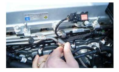
107. Reconnect the fuel line and safety clip on the passenger side of the vehicle.
