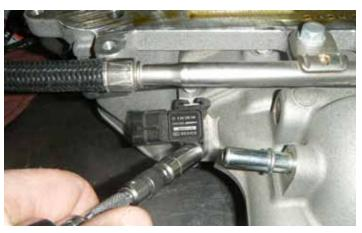
88. Install the inlet air pressure sensor onto the front cover. Using a 10 mm socket, torque the fastener to 10 Nm (89 lb-in). Plug the electrical connector back into inlet air pressure sensor.
