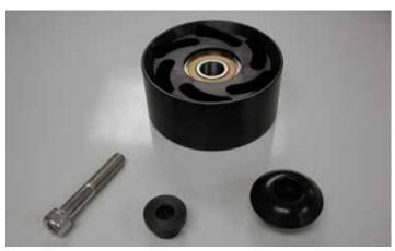
90. The idler to be replaced is the factory 90 mm idler found on the driver side of the vehicle (not the 76 mm idler found near the water pump and tensioner).
