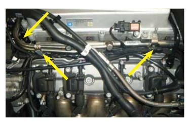
116. Re-attach the three (3) wiring harness fastener clips on the driver side of the vehicle.
