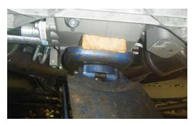
109. Using the jack raise the engine back up into position. Use a wooden block to avoid damage to the oil pan.
