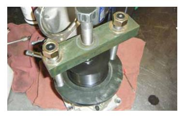
67. Using a pulley removal tool, remove the factory pulley from the supercharger front cover.
