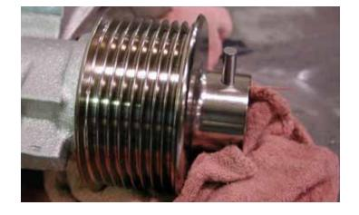
76. Secure the front cover and supercharger pulley. Using a hammer and punch, hit the two surfaces around the pin shown to the left. This will keep the dowel pin securely in place.
