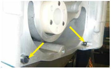
65. Remove the old dowell sleeves from the front cover/housing. Install the supplied dowel sleeves into the LS9 supercharger housing. Install the sleeves in the bottom left and bottom right hand corner of the supercharger housing. DO NOT install sleeves on the front cover.
