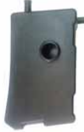
(1x) Intercooler fluid reservoir PN: XX04468-0015
