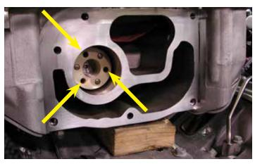
50. Notice the unoccupied holes on the coupler. The drive pins on the supercharger cover shaft will go into these holes.
