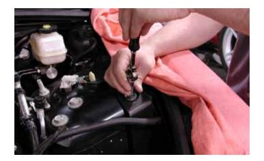
15. Using a 10 mm socket, remove the air filter housing bracket bolt located on the driver side strut tower.
