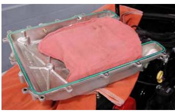
37. Cover the supercharger cover with rags or plastic to prevent debris from entering the cover.
