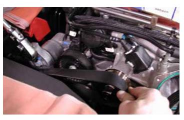
65. Using a breaker bar, release the tension on the tensioner by turning it counter-clockwise. While the tension is released install the LPE supplied belt (part # 8PK1655). See Table 1 on page 29 for recommended belt and idler sizes for the different supercharger pulley and damper diameter combinations.
