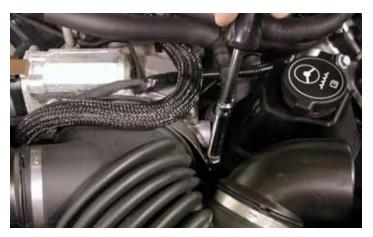
8. Loosen the band clamp on the intake duct that connects to the throttle body.
