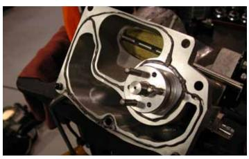
52. Apply a thin film of the supplied Permatex Ultra Black Gasket maker to the mounting surface of the front cover.
