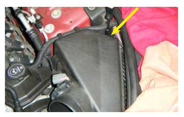
12. The location of the second bolt is located in between the fender and the strut tower.
