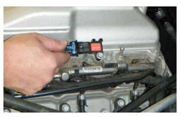
24. Disconnect the manifold absolute pressure (MAP) sensor electrical connector from the left rear of the intercooler.
