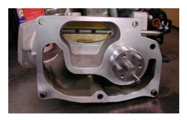
51. Using a razor blade and Scotch pads, scrape and clean the mounting surface of the supercharger front cover.
