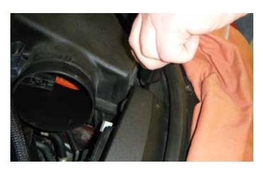
13. The location of the third bolt is directly behind the driver front headlight assembly.
