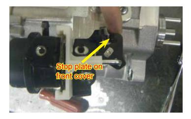
70. Hold the bypass stop plate back so that the bypass valve blade is in the closed position. The stop plate should not be touching the set screw on the bypass actuator. The set screw can be adjusted using a 3/32" Allen wrench.
