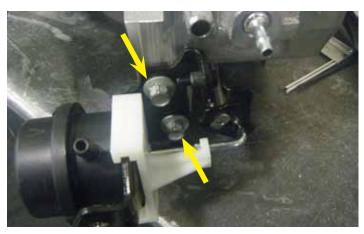
71. Install the two (2) 10 mm bolts and torque them to 21 lb-ft (28.5 Nm).
