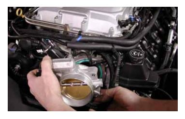
21. Carefully remove the throttle body. Do not allow dirt or debris to enter the throttle body or front cover during the installation.
