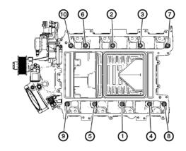
56. Tighten the bolts down in the order shown, using an 8 mm socket make a first pass of 44 lb-in (4 Nm). Then make a final pass in sequence to 89 lb-in (10 Nm).
