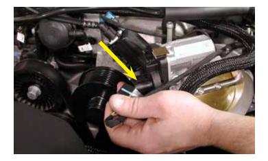
19. Disconnect the throttle actuator electrical connector from the throttle body.
