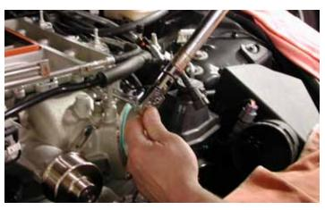
54. Carefully place the supercharger front cover on the supercharger housing. Make sure the pins insert into the empty isolator coupler holes. Using a 10 mm ratchet, torque down the six bolts to 20 lb-ft (27 Nm). As the front cover is being pulled to the supercharger, slight tapping with a rubber mallet on the pulley will help seat the isolator and allow it to spin freely.
