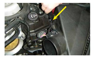
11. Using a T-25 Torx tool, remove the three (3) Torx bolts from the top portion of the air filter housing. The location of the first bolt is next to the power steering reservoir.
