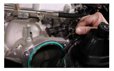
76. Replace the inlet air pressure electrical connector.
