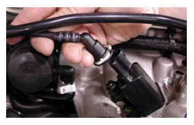
27. Disconnect the evap line from the purge solenoid on the left side of the supercharger front cover.
