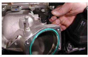
75. Using a 10 mm socket, replace the inlet air pressure sensor and torque down to 89 lb-in (10 Nm).
