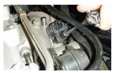
77. Install the purge solenoid onto the front cover. Using a 10 mm socket, torque the fastener to 10 Nm (89 lb-in).
