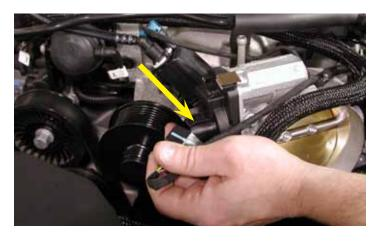
85. Replace the throttle actuator electrical connector to the throttle body.
