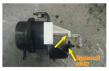
69. Use the set tool to set the actuator position [tool part # ETN86063]. Place the vacuum bypass positioning tool so that the actuator arm teeth are located in the position shown. Note the bypass set screw position.
