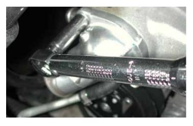
62. Using a 10 mm socket and torque wrench, torque the inlet bolts to 89 lb-in.
