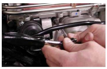
42. Using a 10 mm socket, remove the (6) bolts on the front supercharger cover.
