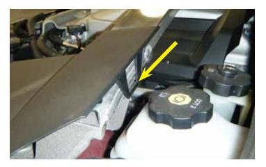
3. Remove the plastic covers on both sides of the motor by un-clipping the covers on the strut tower brace.
