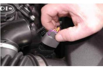
6. Remove the connector from the mass air flow/intake air temperature (MAF/IAT) sensor located on the end of the intake duct on the air filter box.
