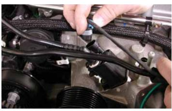
79. Replace the electrical connector to the purge solenoid.
