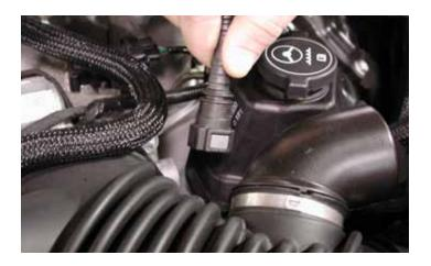
7. Remove the fresh air inlet positive crankcase ventilation (PCV) connector from the middle of the intake duct.
