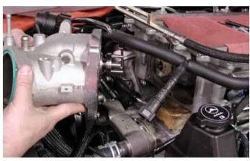
44. Carefully remove the supercharger front cover from the assembly.
