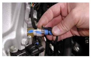
81. Replace the electrical connector to the IAT2 sensor.
