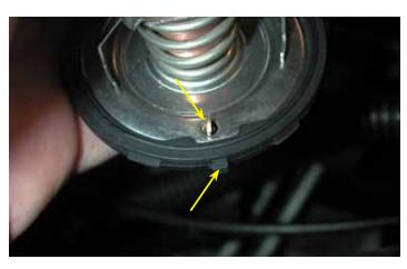
60. On the new thermostat, make sure that the small square tab is lined up with the check valve on the engine side of the thermostat.
