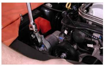
18. Using a 1/2" breaker bar, release the tension in the supercharger belt tensioner located on the passenger side by turning the tensioner counter-clockwise. Grab the belt in an open location and remove from the pulleys
