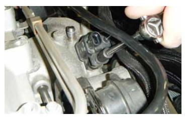
28. Unbolt the purge solenoid using a 10 mm ratchet and extension and carefully remove the purge solenoid.
