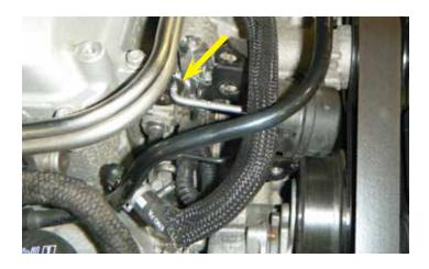
68. Insert the bypass actuator arm into the supercharger front cover bracket. Replace the PCV hose and correct vacuum hose as shown.
