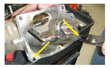
45. Remove dowel sleeves from supercharger front cover (they may also still be in the supercharger) by squeezing with a pair of pliers while twisting and pulling the sleeves out of the cover. You will be replacing these sleeves with new ones.
