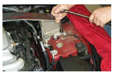
4. Using an 18 mm socket with an extension, remove the strut tower bar by unbolting the two bolts on each strut tower and carefully lifting the strut tower brace out.
