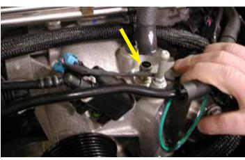
83. Re-connect the brake booster hose on the top of the supercharger front cover.
