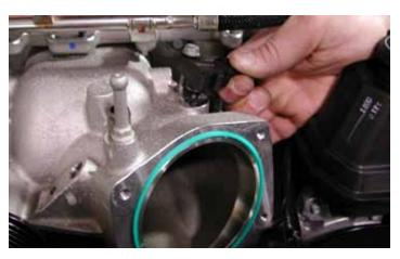
39. Using a 10 mm socket, remove the inlet air pressure sensor. Handle the sensor and O-ring with care.
