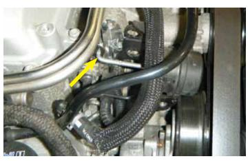
34. Remove the bypass actuator by tilting it upward and removing the metal bar from the bypass shaft linkage.
