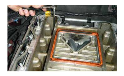
40. Using an 8 mm socket, remove the ten (10) bolts from the supercharger. Refer to the bolt locations below.
