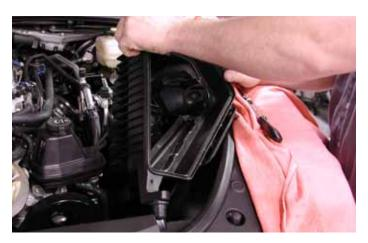
16. Carefully remove the bottom portion of the air filter housing by pulling up and away from the fender from the location shown.
