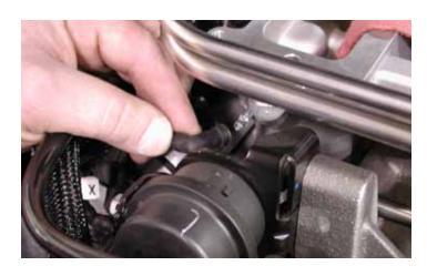
74. Reconnect the vacuum hose from the bypass valve actuator to the supercharger.
