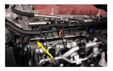
41. Carefully lift up on the front of the supercharger and place a wooden block or equivalent underneath to wedge the front of the supercharger up 1" to 2". Make certain your wedging device is clean and clear of debris
