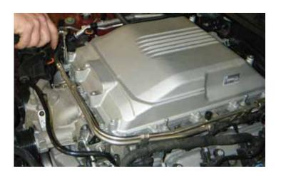
66. Replace the intercooler cover. Using a 10 mm socket torque each bolt down on the first pass to 44 **lb in** (5 Nm) then on a final pass of 89 lb in (10 Nm). Make certain to use the order shown below.
