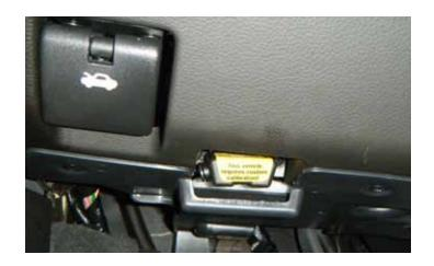
90. Install the supplied diagnostic port (DLC port) cover onto the DLC port in the driver foot well. Secure the strap that retains the DLC cover to the vehicle.
