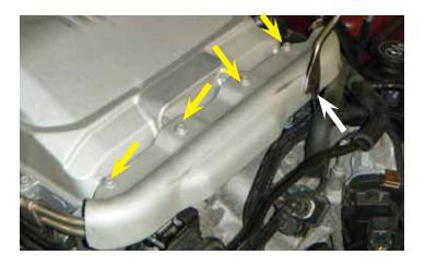
17. Using a fork type pry tool, pry the plastic push pin out at the location shown by the white arrow. Then using a 10 mm socket, remove four (4) bolts on the front fuel line protective cover located on the front of the intercooler shown by the yellow arrows.
