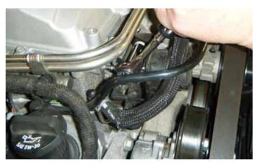
32. Using a 10 mm socket, remove the two bolts on the bypass actuator bracket.
