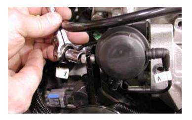
31. Using a 10 mm socket, remove the boost solenoid bracket from the bypass actuator. Make sure any vacuum lines that are connected from the solenoid are disconnected.
