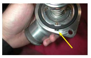
61. Insert the thermostat assembly in the inlet with the square tab aligned with the notched out portion of the inlet. Make sure to press down firmly to properly seat the thermostat and gasket in the housing.
