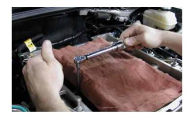
55. Lift up on the front of the supercharger and remove the wood block or wedge that was inserted earlier. Line up the supercharger bolt holes with the corresponding holes in the cylinder heads and insert the ten (10) bolts that secure it.
