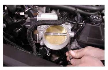
20. Using a 10 mm socket, remove the four (4) bolts that secure the throttle body to the supercharger assembly.
