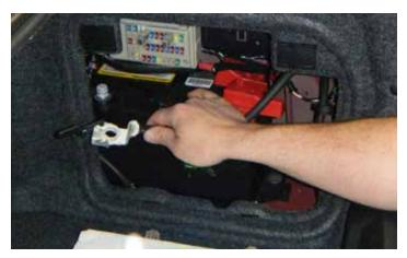
2. Disconnect the battery located in the trunk by releasing the latch and disconnecting the negative (black) from the battery terminal.
