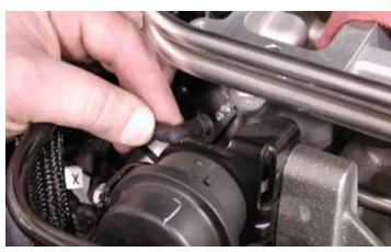
30. Remove the two (2) vacuum lines from the bypass actuator to the intercooler and boost solenoid.
