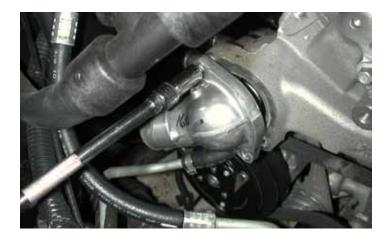
58. Using a 10 mm socket and extension, remove the two (2) bolts that hold the engine coolant inlet.
