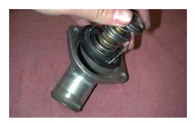
59. Remove the old thermostat from the inlet.
