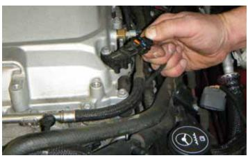
22. Remove the barometric pressure (BARO) sensor electrical connector from the left front of the intercooler.
