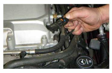
82. Replace the electrical connector to the BARO sensor.
