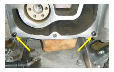
53. Insert the LPE provided dowel sleeves (part # SPIR-69427) into the two (2) locations shown on the supercharger housing by squeezing and twisting them in with pliers.
