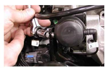
73. Install the boost solenoid bracket onto the bypass valve actuator. Torque the bolt down to 89 lb-in (10Nm).
