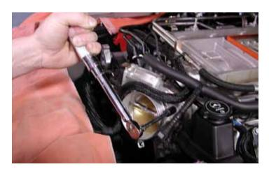
84. Place the throttle body on the end of the supercharger front cover. Using a 10 mm socket, torque down the four (4) bolts to 89 lb-in (10 Nm).
