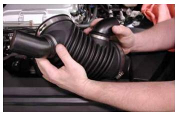
10. Carefully remove the intake duct.
