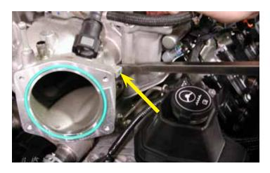
43. Using a pry bar, carefully pry the front cover in the location shown. Make certain any wires or lines are not in the way. This step may require a rubber mallet. Gently tap on the front of the supercharger cover to loosen and continue prying.
