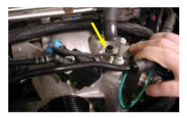
25. Disconnect the brake booster hose from the top of the supercharger front cover.
