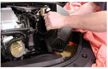
14. Carefully remove the top of the air filter housing.
