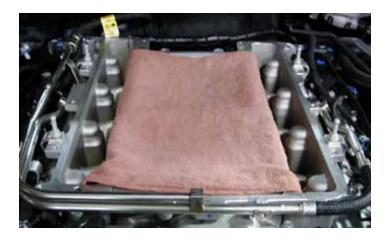
38. Cover the supercharger inlet with rags or plastic to prevent debris from entering the supercharger.
