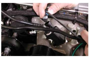
26. Disconnect the purge solenoid electrical connector from the top of the supercharger front cover.
