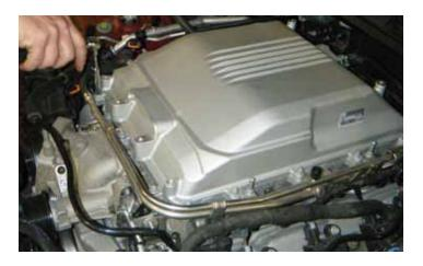
35. Using an 10 mm socket, start with the back six (6) bolts and remove the sixteen (16) bolts from the supercharger cover. Refer to the bolt locations below.
