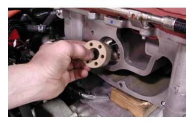
49. Replace the factory isolator coupling with the supplied LPE solid supercharger isolator coupling (LPE part # L960130709).
