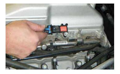
80. Replace the electrical connector to the MAP sensor.
