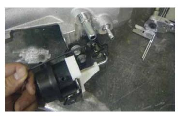
72. Tighten the set screw so that it barely touches the stop plate on the front cover. After the initial contact, tighten the set screw 1/8 to 1/4 turn *more* to set the bypass valve blade into position. The set screw should now be touching the stop plate on the front cover. This will prevent the bypass valve blade from getting stuck on the front cover casting. Remove the bypass actuator set tool.
