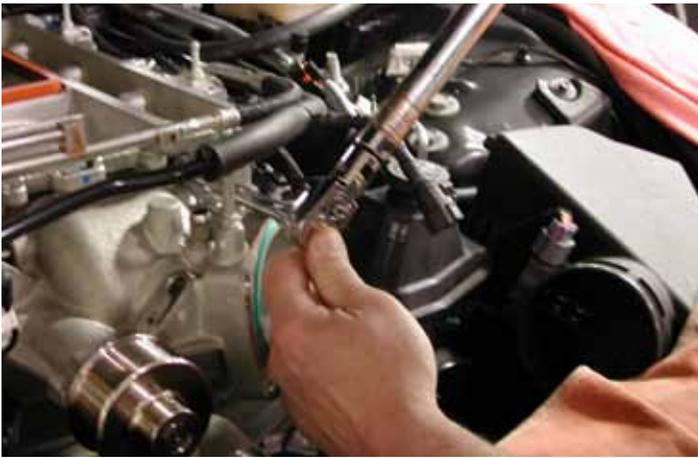
55. Carefully place the supercharger front cover on the supercharger housing. Make sure the pins insert into the empty isolator coupler holes. Using a 10 mm ratchet, torque down the six bolts to 20 lb-ft (27 Nm). As the front cover is being pulled to the supercharger, slight tapping with a rubber mallet on the pulley will help seat the isolator and allow it to spin freely.
