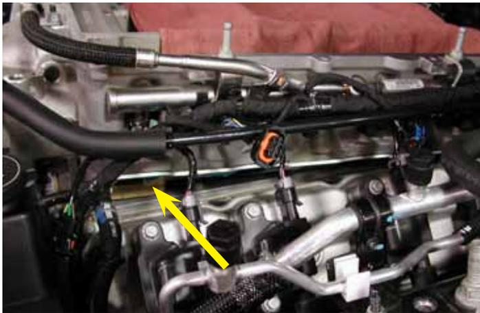
36. Carefully lift up on the front of the supercharger and place a wooden block or equivalent underneath to wedge the front of the supercharger up 1" to 2". Make certain your wedging device is clean and clear of debris
