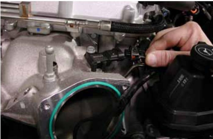
67. Replace the inlet air pressure electrical connector.
