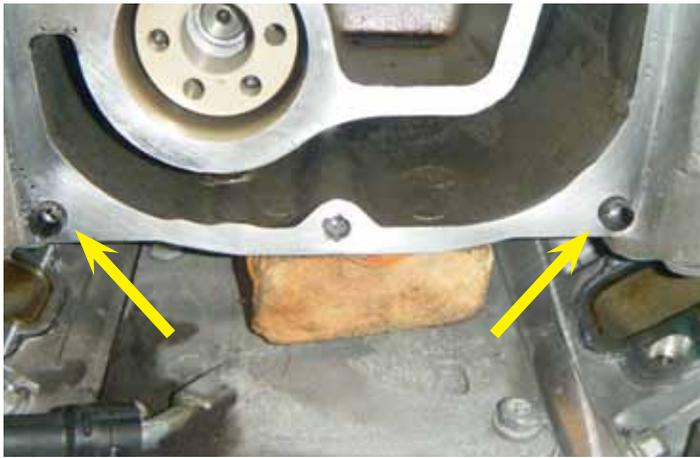
47. Insert the LPE provided dowel sleeves (part # SPIR-69427) into the two (2) locations shown on the supercharger housing by squeezing and twisting them in with pliers.
