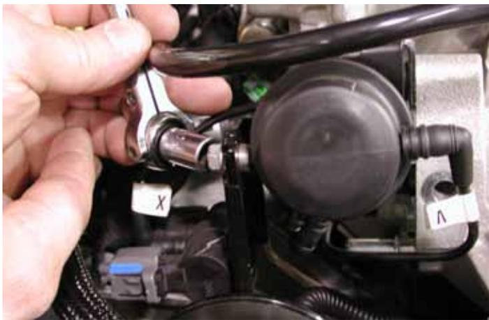
64. Install the boost solenoid bracket onto the bypass valve actuator. Torque the bolt down to 89 lb-in (10Nm).
