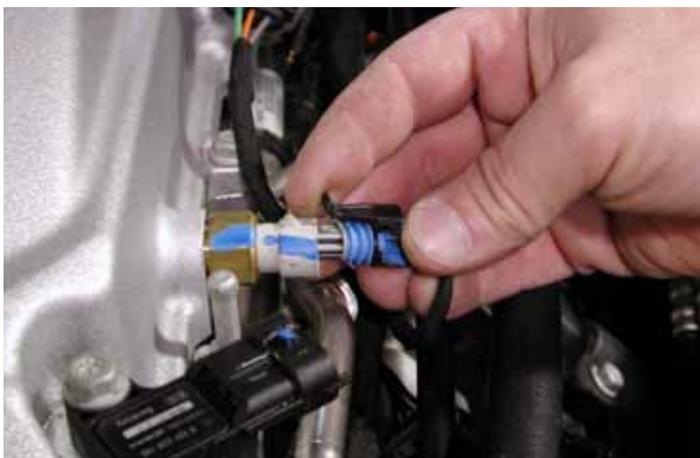
73. Replace the electrical connector to the IAT2 sensor.
