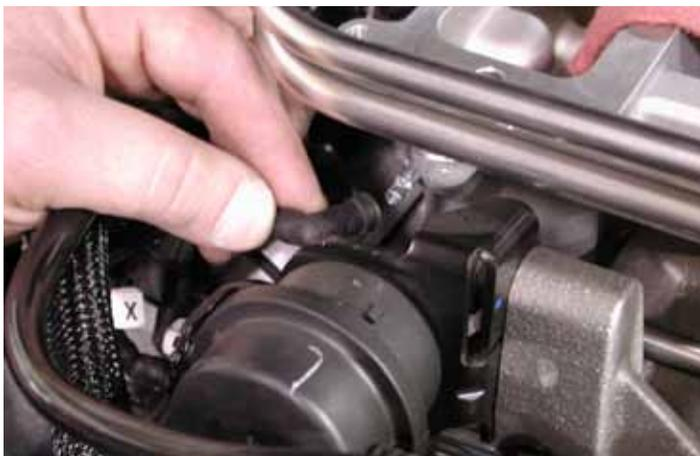
65. Reconnect the vacuum hose from the bypass valve actuator to the supercharger.
