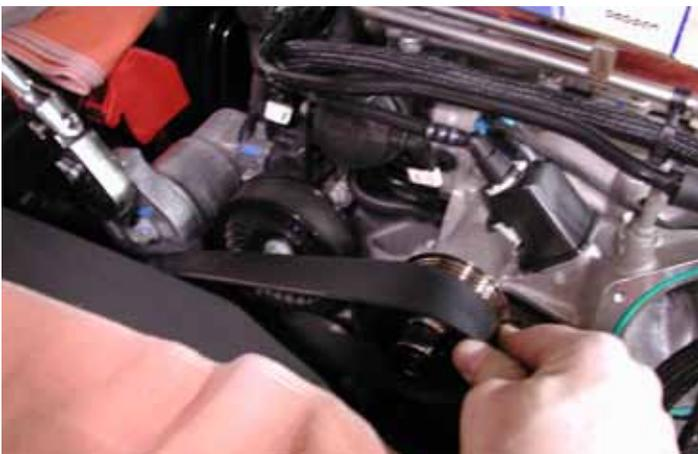
77. Using a breaker bar, release the tension on the tensioner by turning it counter-clockwise. While the tension is released install the LPE supplied belt (part # 8PK1655). See Table 1 on page 33 for recommended belt and idler sizes for the different supercharger pulley and damper diameter combinations.
