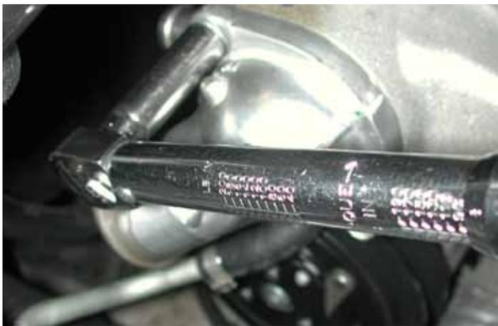
53. Using a 10 mm socket and torque wrench, torque the inlet bolts to 89 lb-in.
