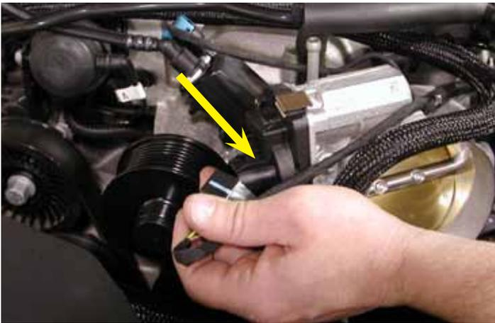
14. Disconnect the throttle actuator electrical connector from the throttle body.
