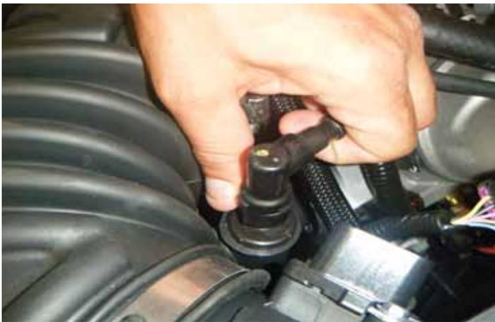
11. The positive crankcase ventilation (PCV) tube goes from the driver-side valve cover to the rubber air inlet tube. Disconnect the PCV tube from the air inlet tube by pressing the retaining tab on the fitting and pulling up on the tube.
