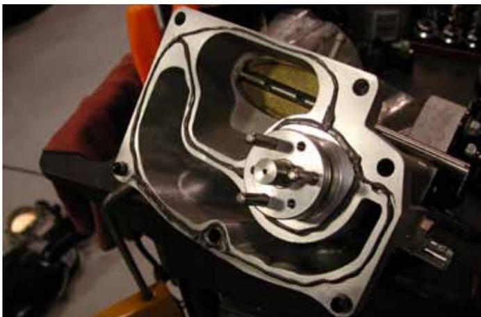
54. Apply a thin bead of the supplied Permatex Ultra Black Gasket maker to the mounting surface of the front cover as shown.
