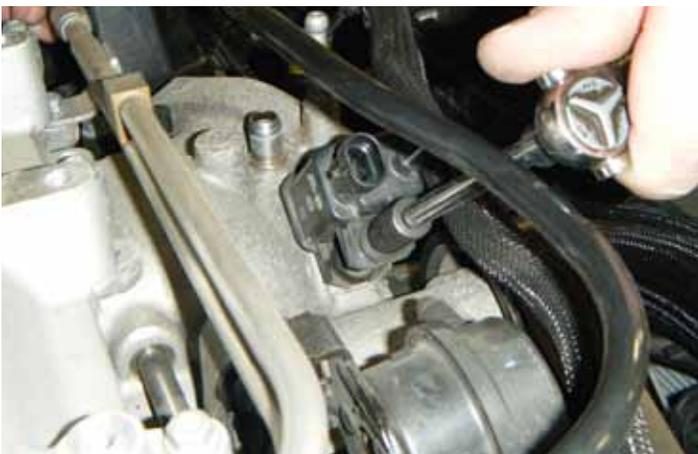
69. Install the purge solenoid onto the front cover. Using a 10 mm socket, torque the fastener to 10 Nm (89 lb-in).
