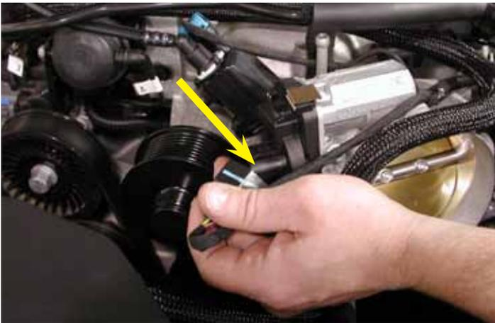
79. Replace the throttle actuator electrical connector to the throttle body.
