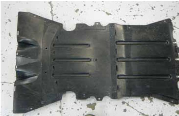
2. If you need to lift the vehicle using a floor jack, remove the belly pan from the underside of the vehicle by removing the fourteen bolts using a 10 mm socket.
