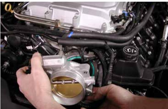
16. Carefully remove the throttle body. Do not allow dirt or debris to enter the throttle body or front cover during the installation.
