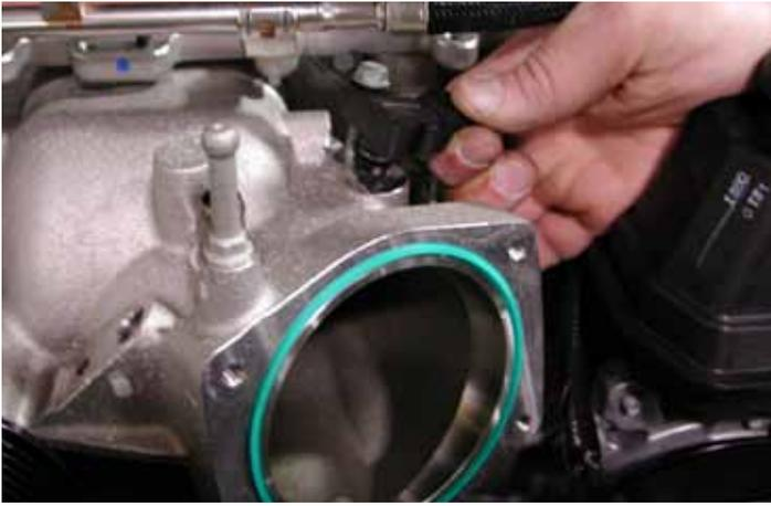
66. Using a 10 mm socket, replace the inlet air pressure sensor and torque down to 89 lb-in (10 Nm).
