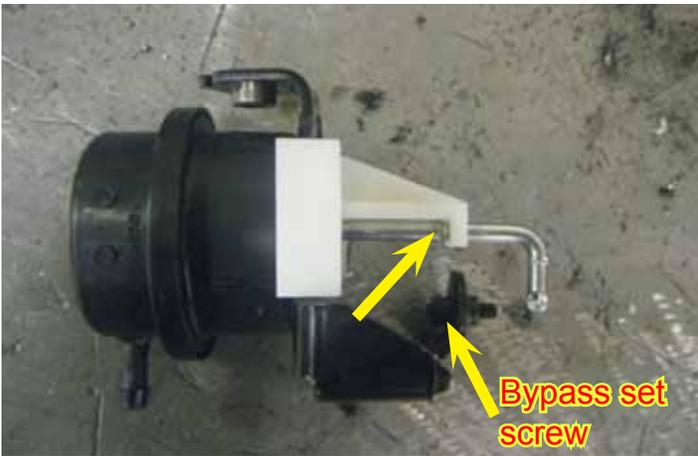
60. Use the set tool to set the actuator position [tool part # ETN86063]. Place the vacuum bypass positioning tool so that the actuator arm teeth are located in the position shown. Note the bypass set screw position.
