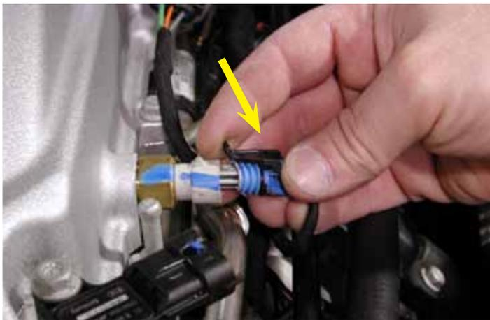
18. Remove the supercharger inlet air temperature sensor (IAT2) electrical connector from the sensor on the left side of the intercooler.
