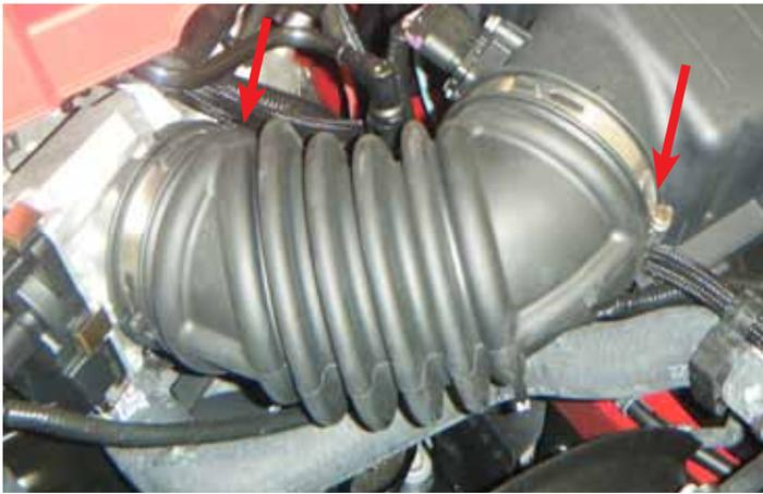
9. Loosen the hose clamps securing the rubber air inlet tube to the throttle body using an 8mm socket.
