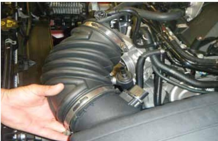
12. Remove the air inlet tube from the throttle body and pull up on the airbox to remove the air inlet tube and airbox assembly.
