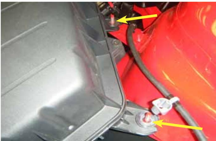
10. Remove the two (2) nuts that hold the airbox in place using a 10mm deep socket.
