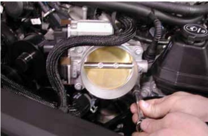
15. Using a 10 mm socket, remove the four (4) bolts that secure the throttle body to the supercharger assembly.
