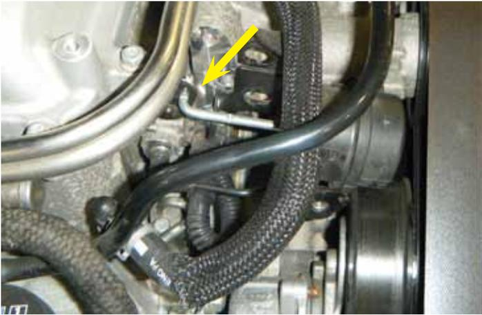
59. Insert the bypass actuator arm into the supercharger front cover bracket. Replace the PCV hose and correct vacuum hose as shown.
