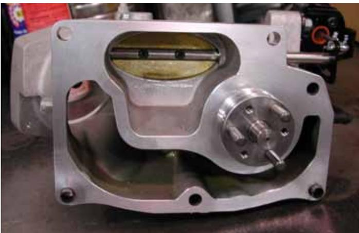
46. Using a razor blade and Scotch pads, scrape and clean the mounting surface of the supercharger front cover.
