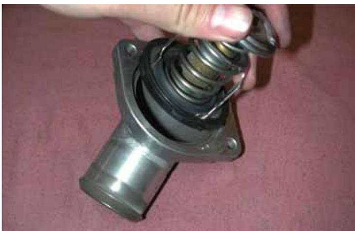
50. Remove the old thermostat from the inlet.
