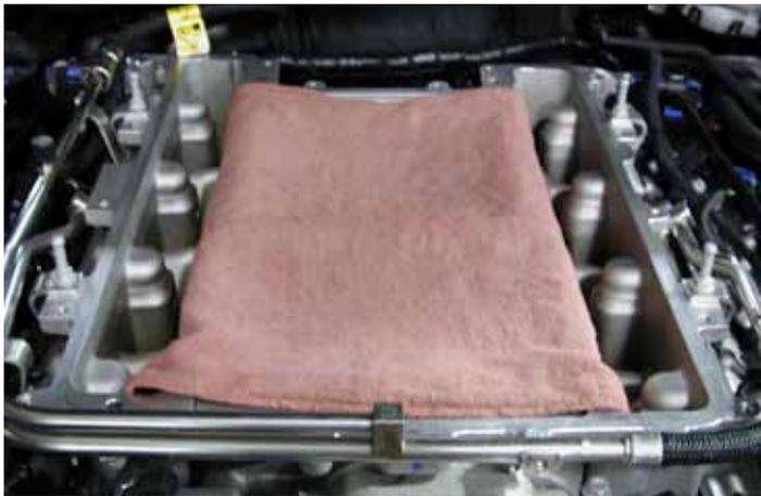
33. Cover the supercharger inlet with rags or plastic to prevent debris from entering the supercharger.
