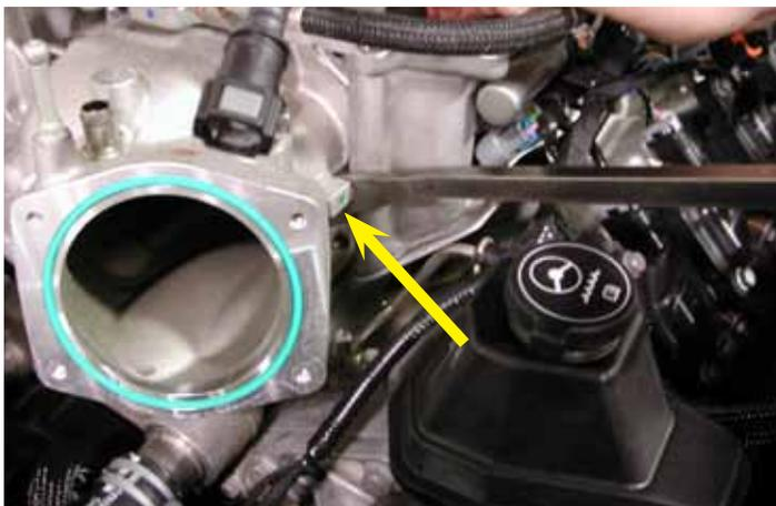
38. Using a pry bar, carefully pry the front cover in the location shown. Make certain any wires or lines are not in the way. This step may require a rubber mallet. Gently tap on the front of the supercharger cover to loosen and continue prying.
