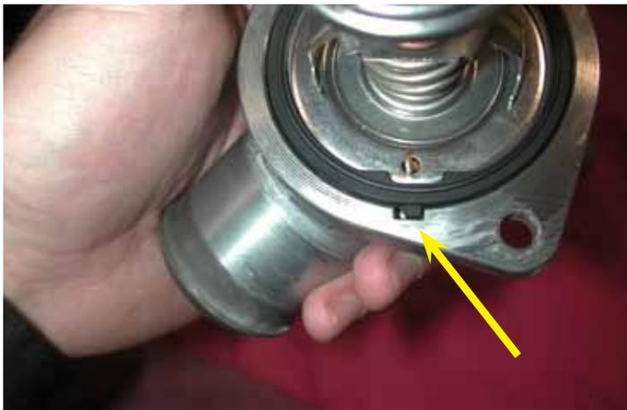
52. Insert the thermostat assembly in the inlet with the square tab aligned with the notched out portion of the inlet. Make sure to press down firmly to properly seat the thermostat and gasket in the housing.
