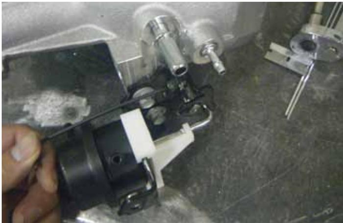
63. Tighten the set screw so that it barely touches the stop plate on the front cover. After the initial contact, tighten the set screw 1/8 to 1/4 turn **more** to set the bypass valve blade into position. The set screw should now be touching the stop plate on the front cover. This will prevent the bypass valve blade from getting stuck on the front cover casting. Remove the bypass actuator set tool.
