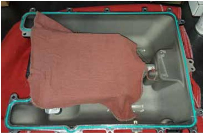
32. Carefully remove the supercharger cover and lay it upside down on the passenger inner fender. Cover the supercharger cover with rags or plastic to prevent debris from entering the cover.
