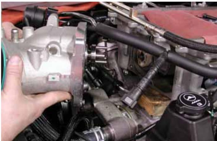
39. Carefully remove the supercharger front cover from the assembly.
