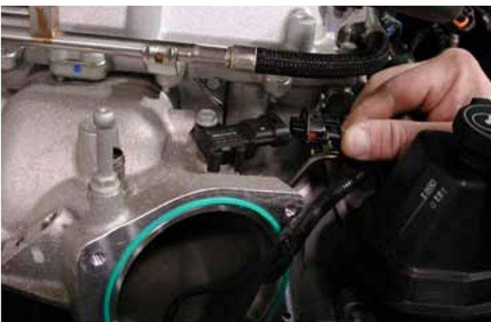
24. Disconnect the electrical connector to the inlet air pressure sensor from the supercharger front cover.
