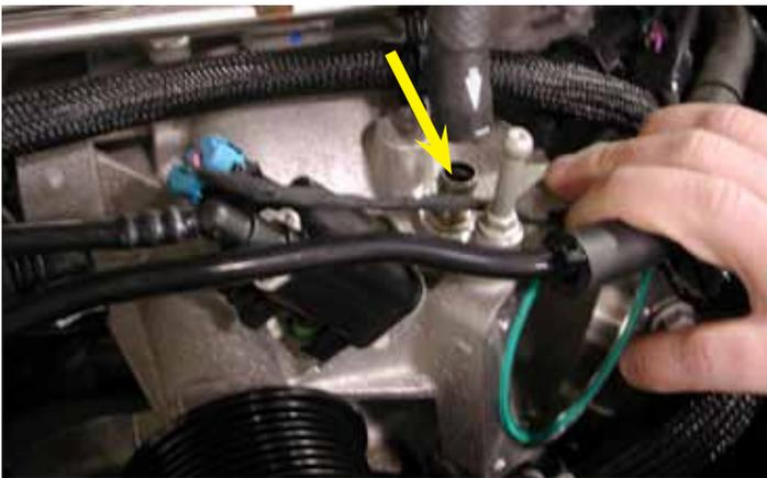
75. Re-connect the brake booster hose on the top of the supercharger front cover.
