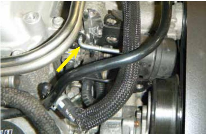
30. Remove the bypass actuator by tilting it upward and removing the metal bar from the bypass shaft linkage.
