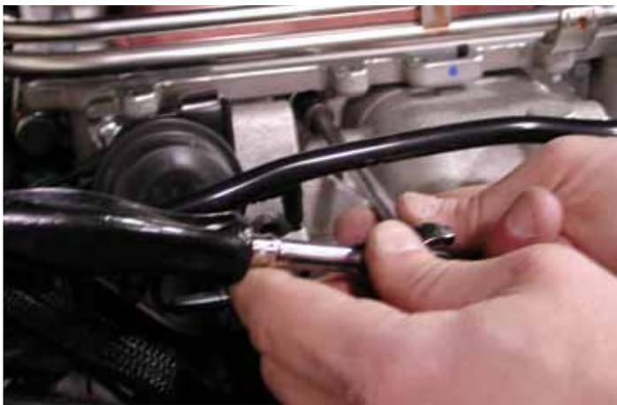
37. Using a 10 mm socket, remove the (6) bolts on the front supercharger cover.
