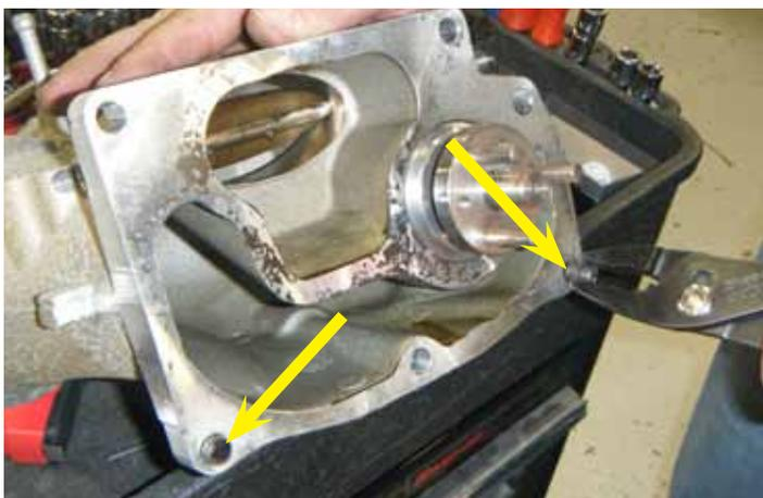
40. Remove dowel sleeves from supercharger front cover (they may also still be in the supercharger) by squeezing with a pair of pliers while twisting and pulling the sleeves out of the cover. You will be replacing these sleeves with new ones.
