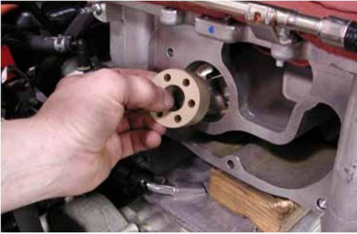
43. Clean the mounting surface of the supercharger housing with a razor blade and Scotch pads.
