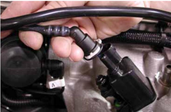
22. Disconnect the evap line from the purge solenoid on the left side of the supercharger front cover.
