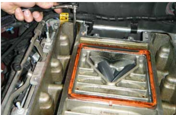
35. Using an 8 mm socket, remove the ten (10) bolts from the supercharger. Refer to the bolt locations below.
