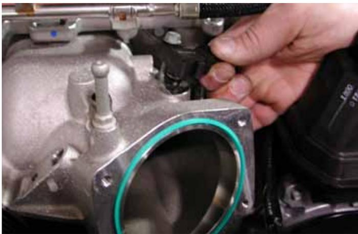
34. Using a 10 mm wrench, remove the inlet air pressure sensor. Handle the sensor and O-ring with care.
