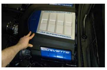
121. Re-install the engine sight shield (engine cover) by pushing down on the cover to secure it to the mounting posts.
