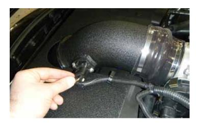
120. Connect the mass air flow sensor connector.
