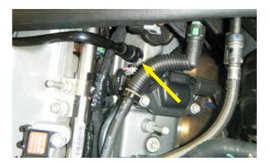
18. Disconnect the PCV fresh air hose line from the left side valve cover (at the rear of the engine).
