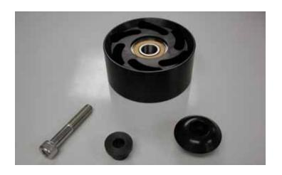
80. If you are using a pulley combination that requires a different idler, replace the factory idler at this time. Follow steps 79 to 81 for installing the new idler. See table 1 on page 37 for information on what size idler is needed for different pulley combinations.
