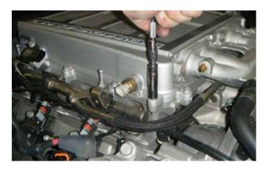
94. Install the seventeen (17) supercharger cover bolts and the supercharger cover.
