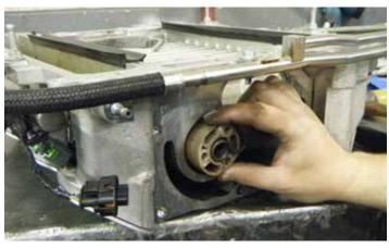
61. Remove the spring loaded isolator coupling from the supercharger assembly (it may be on the front cover assembly).
