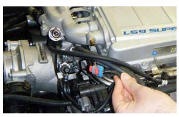
115. Connect the electrical connector to the EVAP purge solenoid.
