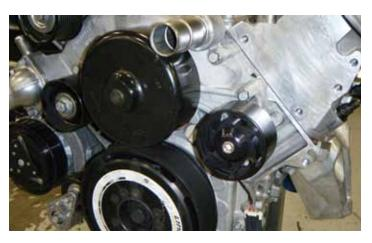
83. Place the supplied idler locating spacer on the back side of the idler. Place the supplied dust shield/cover on the front of the idler pulley. Put the supplied bolt through the idler and install the assembly on the engine.
