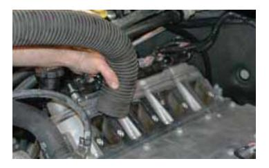
50. Wipe the heads clean of oil using a solvent dampened rag and then vacuum the area of dust and debris. It is very important to maintain a clean work environment.
