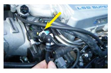
116. Connect the EVAP purge line to the purge solenoid.
