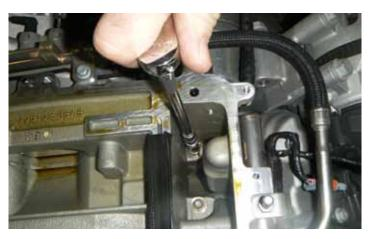
87. Torque down the ten (10) supercharger bolts, refer to the next step for the torque pattern and specifications.
