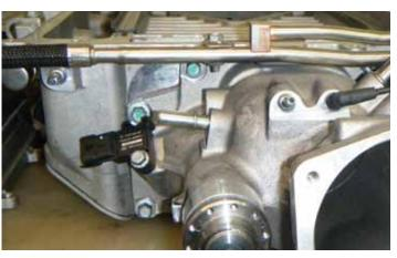
67. Install the six (6) cover bolts with a 10 mm socket and extension. Torque to 27 Nm (20 lb ft). The torque sequence is not critical on this component. With the plastic cover removed from the end of the shaft, tap the end of the shaft with a rubber mallet to seat the plastic shaft coupler. Check to make sure the supercharger assembly turns smoothly. If it doesn't turn freely, tap the end of the shaft again to fully seat the plastic coupler.
