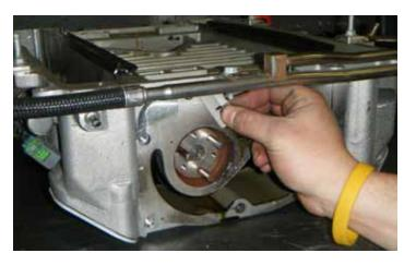
62. Inspect the cover mounting surface on the supercharger assembly. Clean off any remaining adhesive with a razor blade.
