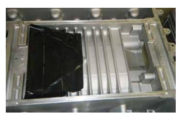
49. Cover the inlet area of the supercharger to prevent dirt or debris contamination on the rotors.
