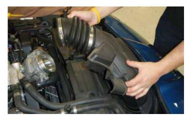
11. Remove the air inlet duct and air filter housing by pulling straight up on the air inlet duct assembly to detach the rubber grommets from the mounting pegs.
