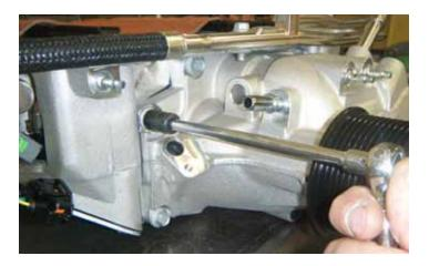
58. Using a 10 mm socket and extension, remove the six (6) bolts that secure the front cover to the supercharger assembly.
