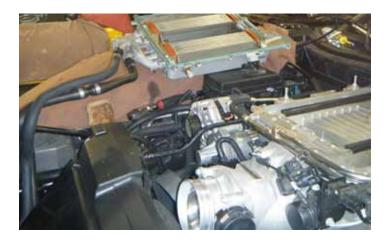
86. With the help of an assistant, place the supercharger assembly back in place on the engine. Align the dowel pin at the right front of the supercharger to the cylinder head.
