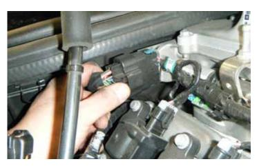
19. Disconnect the fuel injector and ignition coil harness connector from the passenger side of the engine.
