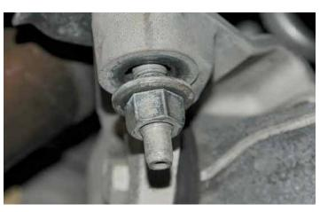
35. Loosen the engine cradle nuts such that you have roughly a 1 inch (25 mm) gap between the nut and the subframe. You should still have several turns of engagement on the threads on each nut. Do not remove the nuts from the studs.
