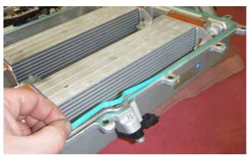
93. If you removed or are replacing the supercharger cover seal, install the supercharger cover seal.
