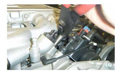
112. Connect the brake boost vacuum line to the supercharger front cover.
