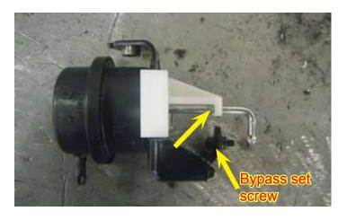
72. Use the set tool to set the actuator position [tool part # ETN86063]. Place the actuator set tool so that the actuator arm teeth are located in the position shown. Note the bypass set screw position.
