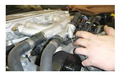
14. Disconnect the active exhaust vacuum hose that routes from the left side of the engine compartment to the front of the supercharger.
