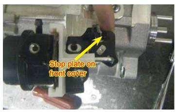
73. Hold the bypass stop plate back so that the bypass valve blade is in the closed position. The stop plate should not be touching the set screw on the bypass actuator. The set screw can be adjusted using a 3/32" Allen wrench.
