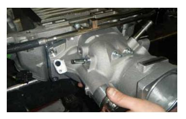
66. Install the new cover onto the supercharger assembly. The three pins sticking out of the supercharger drive shaft in the front cover go into the three holes in the plastic coupler that are not occupied by the pins from the supercharger assembly.
