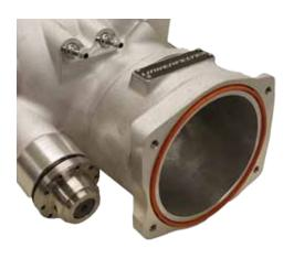
68. Install the supplied O-ring onto the throttle body.
