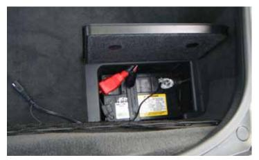
2. Open the rear hatch and open the battery compartment cover. Using a 10 mm socket wrench, disconnect the negative (-) battery cable from the terminal on the battery. Cover the cable end with electrical tape so accidental connection to the battery does not occur.
