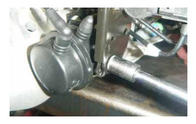
76. Install the boost control solenoid bracket assembly onto the front cover. Using a 10 mm socket, torque the fastener to 10 Nm (89 lb-in). Replace all vacuum hoses.
