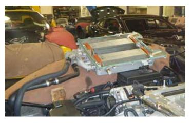
39. With the intercooler fluid lines still connected to the cover, put the cover off to one side of the engine compartment and cover with a plastic bag or rags to prevent dust and debris from getting into the cover.
