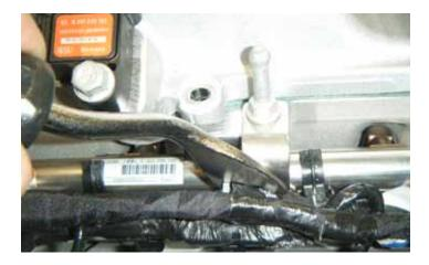
26. Using a fork type pry tool, carefully pry the wiring harness fastener clip located on the rear of the driver's side fuel rail.
