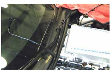
23. Move the PCV air house assembly out of the way by rotating it up and over.
