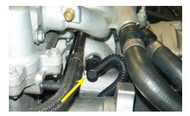
90. Connect the PCV dirty air hose line to the passenger side of the supercharger front cover.
