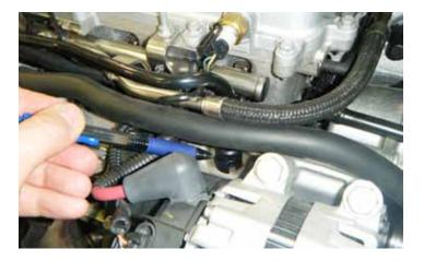
22. Disconnect the PCV fresh air hose line from the right valve cover (at the front of the engine).
