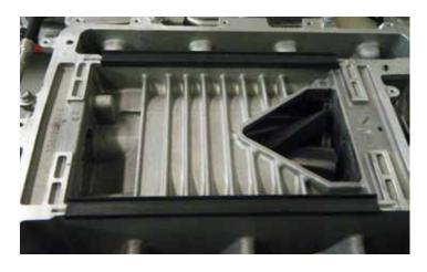
92. Install insulator seals on the supercharger assembly.
