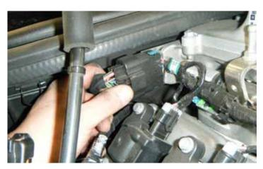
111. Connect the fuel injector and ignition coil harness connector on the passenger side.
