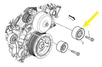
81. The idler to be replaced is the factory 90 mm idler found on the driver side of the vehicle (not the 76 mm idler found near the water pump and tensioner).
