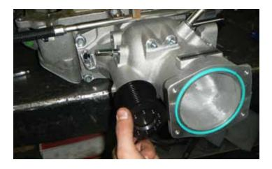
69. Install the supercharger pulley onto the hub on the supercharger shaft.
