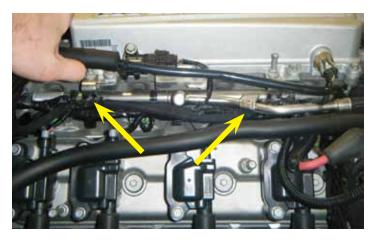
106. Re-attach the two (2) wiring harness fastener clips on the passenger side of the vehicle.
