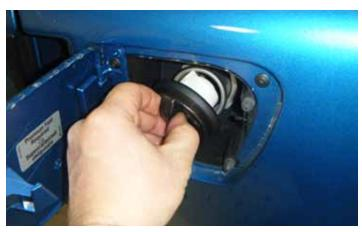
101. Lower the vehicle back down onto the ground and re-install gas cap
