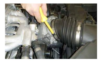
10. Using a 5/16" nut driver or socket, loosen the clamp on the throttle body
