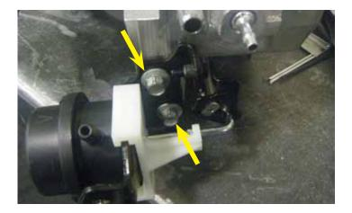
74. Install the two (2) 10 mm bolts and torque them to 21 lb-ft (28.5 Nm).
