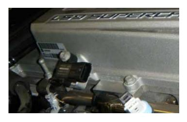
108. Connect the barometric pressure sensor electrical connector.
