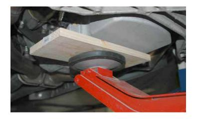
98. Using the jack, raise the engine back up into position.
