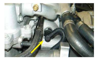
42. Remove the PCV dirty air hose line from the passenger side of the supercharger.
