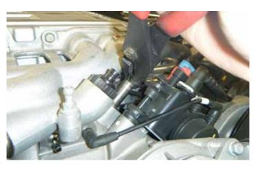
15. Disconnect the brake boost vacuum hose that routes from the left side of the engine compartment to the front of the supercharger.
