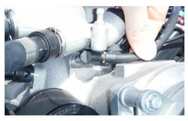
113. Connect the active exhaust vacuum hose to the supercharger front cover.
