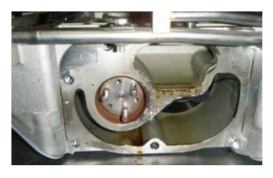
60. Remove the front cover from the supercharger assembly.
