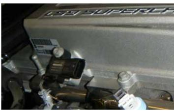
21. Disconnect the barometric pressure sensor electrical connector on the right side (passenger side) of the intercooler.
