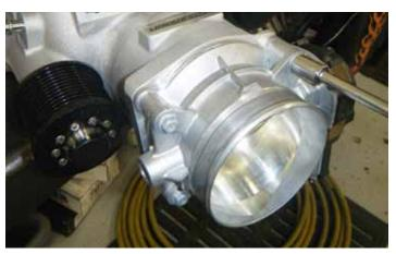
79. Install the throttle body on the supercharger front cover. Using a 10 mm socket, torque the four (4) bolts to 10 Nm (89 lb-in).
