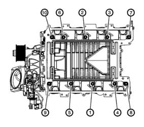
88. Tighten the bolts a first pass in sequence to 5 Nm (44 lb-in).
