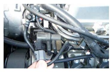
114. Connect the electrical connector to the supercharger boost control solenoid and connect EVAP hose to solenoid.
