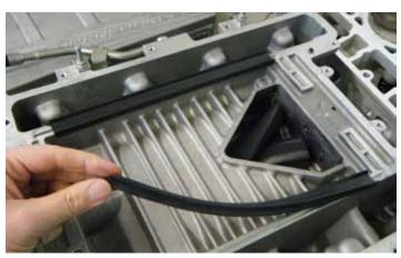
41. Inspect the supercharger insulator seals. Replace if damaged [GM part # 12609472].
