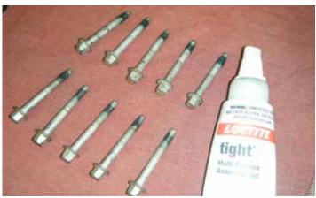
85. Apply a 5 mm (0.2 inch) band of threadlocker (Loctite Blue, GM PN 12345382 or equivalent) to the threads of the 10 supercharger bolts. Place the ten bolts into the supercharger.
