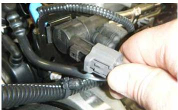
13. Disconnect the electrical connector from the supercharger actuator solenoid at the left front of the supercharger.
