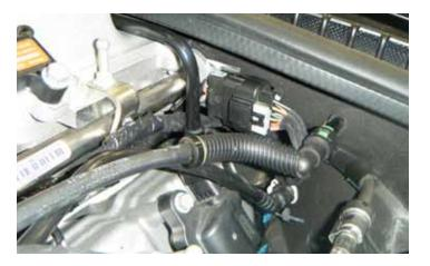
110. Connect the fuel injector and ignition coil harness connector on the driver side.
