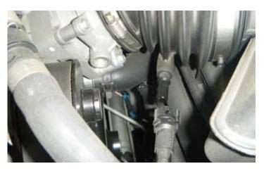
7. Disconnect the positive crankcase ventilation (PCV) fresh air tube from the passenger side of the air inlet duct. Remove the PCV inlet tube from the air filter bellows by pushing up on the release lever. Next pull the tube free from the air duct barb. This same removal method will be used with the other similar PCV connections.
