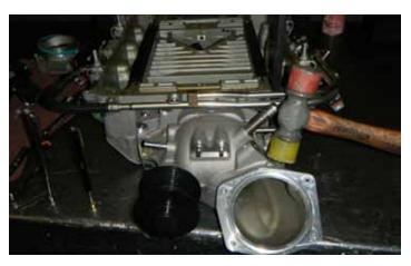
59. Using a mallet (or pry bar) gently knock the front cover loose from the supercharger assembly. The front cover is held in place by two dowels and the pins in the supercharger shaft coupler. Use the mallet to loosen the adhesive between the cover flange and the supercharger housing.
