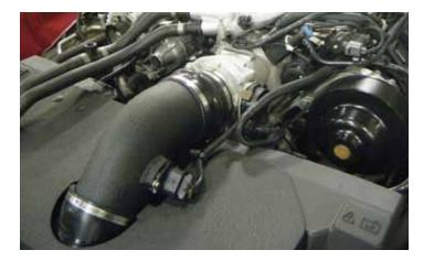
118. Install the air intake system.
