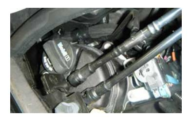
104. Connect the PCV fresh air hose assembly to the left and right valve covers and the dry sump tank.
