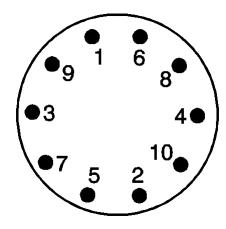
70. Apply a small amount of Loctite Blue to the supplied M4x0.7x12 socket head cap screws and, using a 3 mm Allen wrench or socket, secure the pulley to the hub with these screws. Use the pattern to the left to tighten the screws. Torque to 2.3 Nm (20.7 lb-in). For instructions on supercharger pulley removal, refer to page 34.
