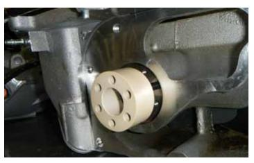
63. Install the supplied plastic isolator coupling on the pins on the shaft in the supercharger assembly. The holes are evenly spaced so it does not matter what set of holes you use. The new isolator coupling will be a tight fit on the pins.
