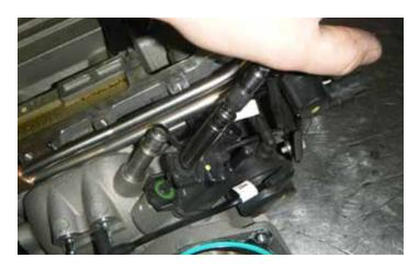
56. Using a 10 mm socket, remove the bolt to the purge solenoid from the supercharger front cover.
