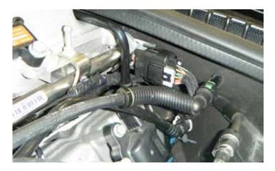
16. Disconnect the fuel injector and ignition coil harness connector from the driver side of the engine.
