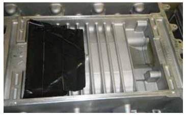
89. Remove the tape or other covering material from the supercharger housing.
