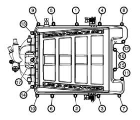
95. Tighten the bolts a first pass in sequence to 5 Nm (44 lb-in).
