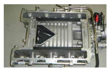
48. With the help of an assistant, remove the supercharger assembly. The supercharger, throttle body, fuel injection rail and fuel injectors may be removed as an assembly. Use caredo not reposition or bend the intercooler cover dowel pins. Do not lift the supercharger assembly from the black plastic vacuum actuator as you risk damaging the actuator.
