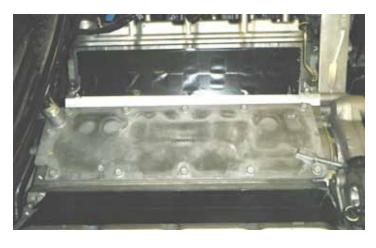
84. Make sure the cylinder head and engine area are free of loose debris. Remove the tape from the cylinder head intake ports.
