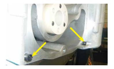
64. Remove the old dowel sleeves from the front cover/housing. Install the supplied dowel sleeves into the LS9 supercharger housing. Install the sleeves in the bottom left and bottom right hand corner of the supercharger housing. DO NOT install sleeves on the front cover.
