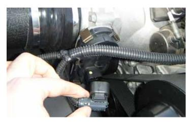
119. Connect the throttle actuator electrical connector.
