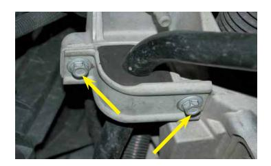
33. Using a 13 mm socket and the 6" extension, remove the sway-bar bushing to cradle bracket bolts (2 per side) and then remove the brackets from both sides. Allow the sway bar to swivel down but do not remove the sway bar.
