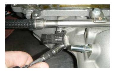
78. Install the inlet air pressure sensor onto the front cover. Using a 10 mm socket, torque the fastener to 10 Nm (89 lb-in). Plug connector back into inlet air pressure sensor.
