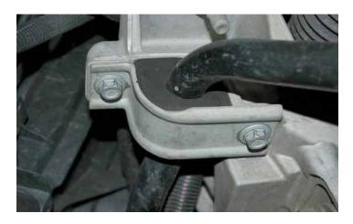
100. Using a 13 mm socket and the 6" extension, install the sway bar bushing to cradle brackets and bolts on both the left and right side. Torque to 58 Nm (43 lb-ft).
