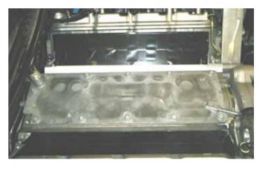
51. Cover the intake ports on the engine with tape or rags to make sure nothing enters the engine.
