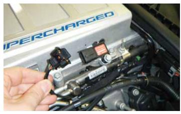
109. Connect the boost pressure sensor connector.
