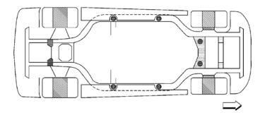
32. Raise the vehicle with a vehicle hoist or a jack and jackstands. Be careful to follow the GM lifting procedures on the ZR1 Corvette due to the carbon fiber aerodynamic components being easily damaged and the low ride height of the vehicle.
