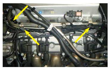
105. Re-attach the three (3) wiring harness fastener clips on the driver side of the vehicle.
