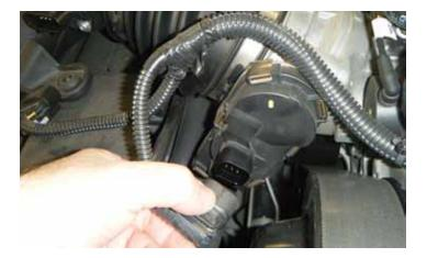
6. Disconnect the throttle actuator electrical connector from the throttle body.
