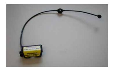
125. Install the supplied diagnostic port (DLC port) cover onto the DLC port in the driver foot well. Secure the strap that retains the DLC cover to the vehicle.
