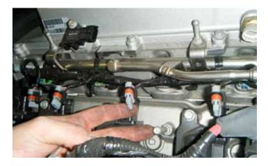
102. Connect the ignition coil electrical connectors to the ignition coils on both sides (8 coils).
