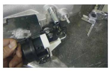
75. Tighten the set screw so that it barely touches the stop plate on the front cover. After the initial contact, tighten the set screw 1/8 to 1/4 turn *more* to set the bypass valve blade into position. The set screw should now be touching the stop plate on the front cover. This will prevent the bypass valve blade from becoming stuck on the front cover casting. Remove the bypass actuator set tool.
