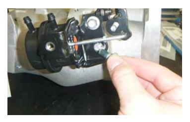
71. Using a 10 mm socket, torque the two (2) bypass actuator bolts to 18 lb-ft (25 Nm). In the new casting the bottom bolt hole is machined all the way through to the inside of the front cover so the bolt going into this hole needs thread sealant applied to the threads [Loctite 567 thread sealant or equivalent].
