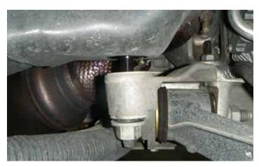
99. Using a 21 mm socket, tighten the four engine cradle stud nuts (two on each side) and torque to 110 Nm (81 lb-ft). You can now remove the jack from under the engine.
