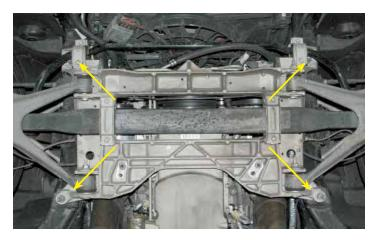
34. Using a 21 mm socket, loosen the four engine cradle retaining nuts on both sides.
