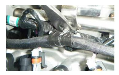
28. Using a fork type pry tool, carefully pry the wiring harness fastener clip located on the rear of the passenger side fuel rail.
