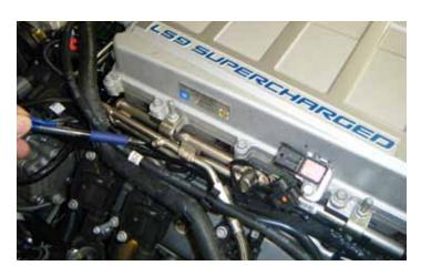
44. Bleed the fuel system pressure to 0 psi at the service test port on the driver side fuel rail.
