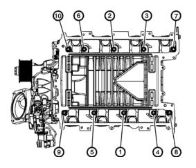
47. Remove the ten (10) 8 mm socket head bolts that retain the supercharger assembly.
