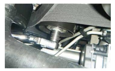
82. Using a 15 mm socket, remove the bolt that secures the factory 90 mm idler.
