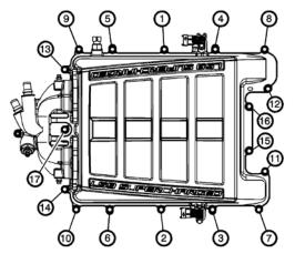
37. Remove the seventeen (17) 10 mm head bolts that secure the supercharger cover to the supercharger assembly.
