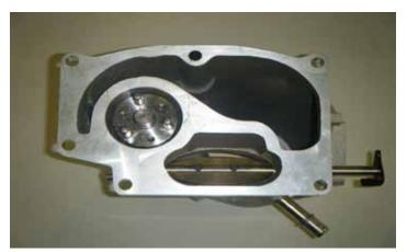
65. Apply a thin film of the supplied Permatex Ultra Black Gasket Maker to the Lingenfelter LS9 cover flange surface.
