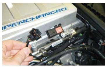
17. Disconnect the air outlet pressure sensor (boost pressure) harness connector from the sensor on the driver side of the vehicle.
