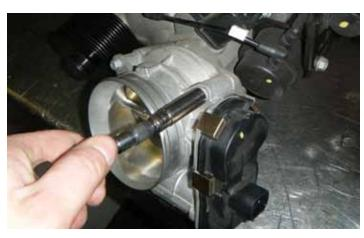
53. Using a 10 mm socket, remove the four (4) bolts that secure the throttle body to the supercharger assembly. Remove the throttle body.
