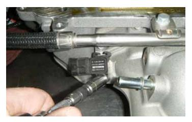
91. Connect the engine inlet air pressure sensor electrical harness.
