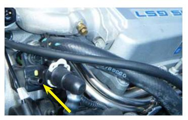
31. Disconnect the purge line from the purge solenoid on the left side of the supercharger front cover.
