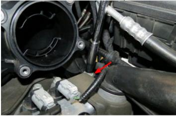
43. Once the manifold is removed, cover the intake ports to ensure nothing falls down into the ports.
