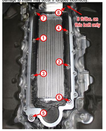
56. It is recommended to use copper sealant spray (or similar) on the bottom of the supercharger gasket to help keep it in place while positioning the supercharger.
