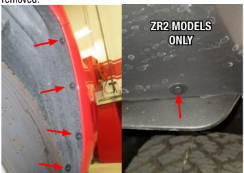
16. Fold back the inner fenderwell. Using a 7mm ratchet, remove the 3 screws holding the fender to the bumper cover. Do this for each side.
