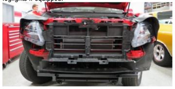
20. Remove the grill seal from the shutter assembly by removing the plastic fasteners (green arrows) and then reach inside the housing, through the shutters, and pressing the 6 tabs (red arrows) until it is free. TIP: A short flat-head screwdriver helps in disengaging the tabs. **NOTE:** Some models may not be equipped with shutters.
