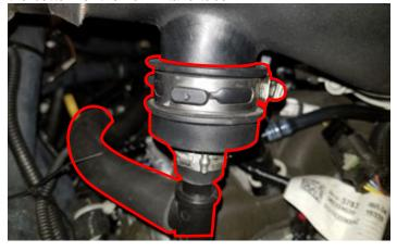
71. Connect the PCV line to the fitting on the intake tube.
