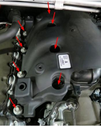
41. Behind the intake manifold, there are two bolts attaching the intake to a steel bracket. Using a 10mm, remove these two bolts.
