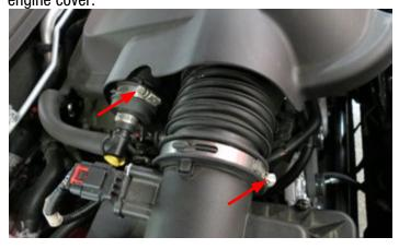
33. Using a 10mm socket and a long extension, remove the 2 bolts holding the engine cover to the engine.
