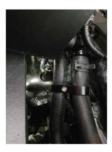
**Step 9:** install the hose separator that's supplied in your intercooler tank kit.
