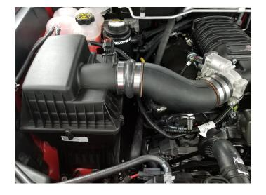
**Step 11:** Reinstall upper air box, air inlet tube and all connectors.
