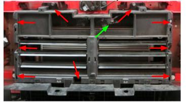
22. Carefully remove the plastic cowl on the passenger (right) side of the vehicle.
