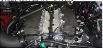
44. Using a 13mm socket, remove the front engine cover bracket. Renstall the original bolt in the passenger side.
