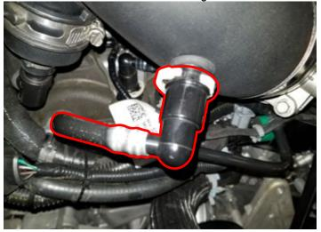
72. Unplug the MAF connector & attach the TMAP harness to the MAF. Reconnect the MAF sensor plug into the TMAP harness. Then connect the last plug into the TMAP extension located on the intake that was installed earlier.
