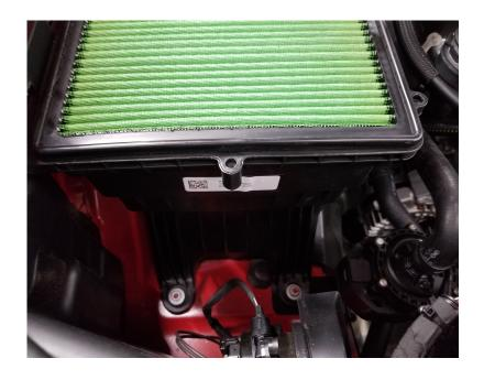
**Step 3:** Remove the two 10mm nuts at the bottom of the air box, then remove air box.
