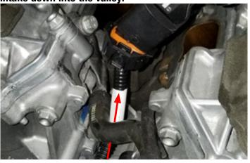
55. From bag #3, use the (7) M8 x 65mm bolts, and the (1) M8 x 30mm intake bolt in the back. Apply Blue Loctite to all. Use the following sequence to torque bolts 1 through 7 to 18 ft/lbs. Torque the #8 bolt (the short bolt) to 8 ft/lbs. Damage to intake may occur if torqued incorrectly.
