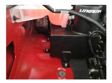
**Step 4:** Slide your new intercooler tank under the factory coolant reservoir.
