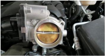
38. Using a T25 screwdriver, remove the MAP sensor and disconnect the cable. Set the MAP sensor aside. It will be reinstalled on the supercharger.
