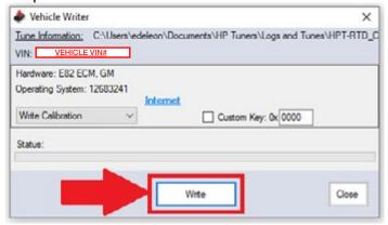
12. Once the flash is completed, click CLOSE, turn the ignition OFF and disconnect the RTD from your OBDII port. The engine is now ready to start once the supercharger installation is complete!
