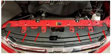
15. Remove the T15 screws (6 on each side) that attach the inner fender to the bumper cover. Do this for each side. **NOTE:** ZR2 models will need an additional T15 removed.
