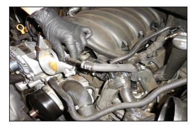
56. Release the blue locking tab, shown at the yellow arrow, on the MAP sensor electrical connection and unplug it.
