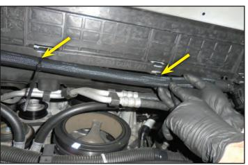
151. Here is a photo of the completed routing of hoses and cable ties.
