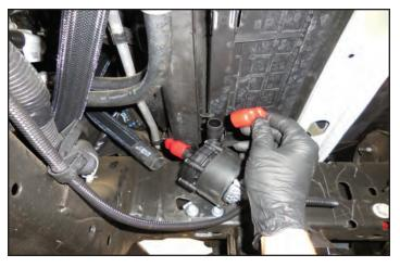
147. Attach the hose from the reservoir at the intercooler pump inlet yellow arrow location and secure with a provided spring clamp. Attach the hose that comes from the lower LTR inlet pipe to the output of the intercooler pump at the red arrow and secure with a provided spring clamp.
