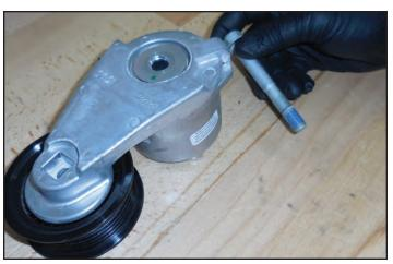
103. Once you have installed the bolt from the last step you will see the boss at the back of the tensioner shown with the arrow.
