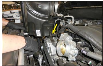
53. Acquire a belt removal tool like the one shown. Alternatively you could cut the belt out.
