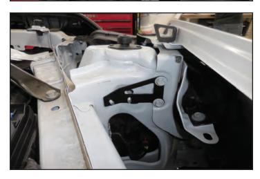
122. Run the gray plug from the intercooler pump harness through the opening shown with an arrow.
