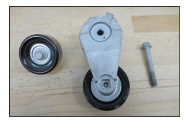
100. **Apply Blue Loctite 242** to the threads of the pre-installed bolt on the idler.
