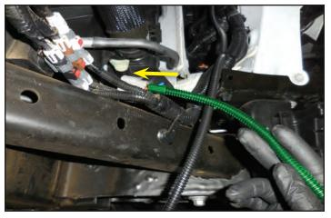
143. Route the gray connector over to the intercooler pump. Look at the next step to see how to attach a cable tie to the wire loom.
