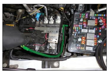
130. Place the ground wire eyelet from the intercooler harness on top of the OEM ground and reinstall the bolt from two steps ago.
