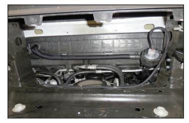
152. Use two cable ties (highlighted in green) to secure the slack of the wire harness that goes to the intercooler pump in the passenger fender well, behind the headlight bucket.
