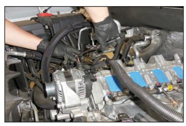
90. Remove the alternator positive cable terminal.
