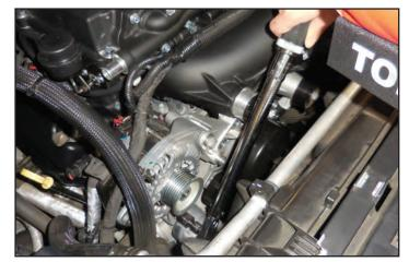
193. Rotate the alternator into the new idler bracket and insert the stock bolt.
