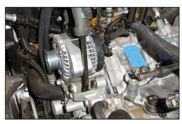
94. Remove the bolt at the water pump. The smaller photo below shows the location better with an arrow.
