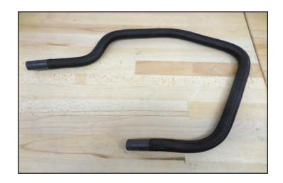
263. Route the hose from the last step as shown here. This hose will go around the air box.
