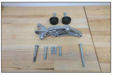
172. Lift the front of the supercharger to place the idler bracket from the last step into position. You will have to align the bracket down in the pocket the alternator used to sit in. Gently lower the supercharger back down and verify that the bracket moves freely.
