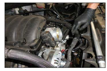
64. Remove the cable tie fasteners from the arrow locations. Repeat this process on the opposite side of the intake manifold.
