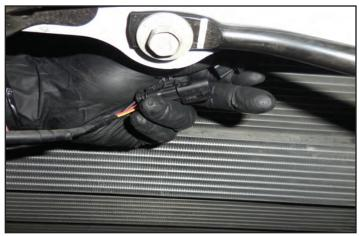
12. Trace around the bracket with a pencil to aid in re-alignment later. Remove the two bolts holding the hood latch assembly with a 13mm socket wrench.
