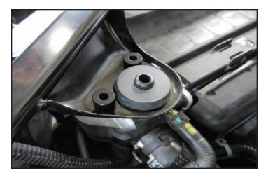
108. Place the bracket on top of the spacers, and install the two M6x25mm bolts from two steps ago through the top and secure them with the M6 serrated flange nuts from below. Use a 10mm socket wrench on top and a 10mm open end wrench on the bottom.
