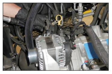
91. Remove the alternator bolt shown at the arrow using a 15mm socket wrench.
