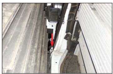
16. Once loosened, pivot the brace inward and down until it touches the back of the shutters. Here you can see the passenger side long diagonal brace moved out of the way. Repeat this process on the driver side long diagonal brace. This will give the necessary room to install the Low Temperature Radiator (LTR) for the intercooler system.
