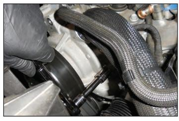
95. Use the provided bolt shown below to press out the bushing at the arrow.
