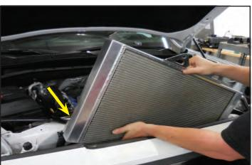
41. Here you can see the LTR hose installed through the radiator panel hole.
