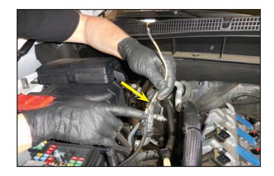
136. Route the yellow trigger wire though the hole that was made in the fuse box cover. Make sure the grommet is fully seated on both sides.
