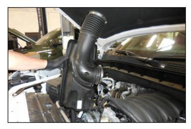
52. Pull the air intake plenum to the passenger side to remove it from the vehicle. This will not be reused.
