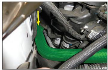
256. After the hose passes through the rubber shield it will be seen through the front like this.
