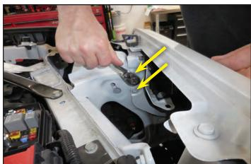
121. Place the intercooler electrical harness bracket in the location from the last step using the two OEM bolts that were just removed.
