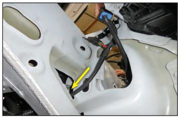
125. Secure the relay and fuse holder to the bracket with the provided serrated flange nuts.
