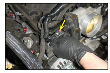
60. Unplug the alternator electrical connection shown with the arrow.
