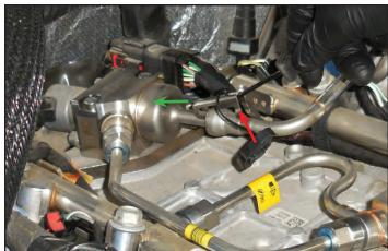
163. Remove the plastic tether from the securing clip. This will not be reused.
