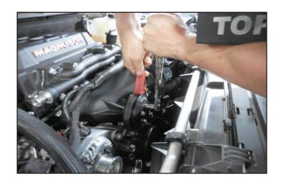
199. Install the belt following the diagram at the back of this manual. Connect a belt tensioner wrench or 1/2" breaker bar at the tensioner and rotate it counter-clockwise. The last pulley to place the belt over should be the smooth pulley that was installed on the right side three steps ago.
