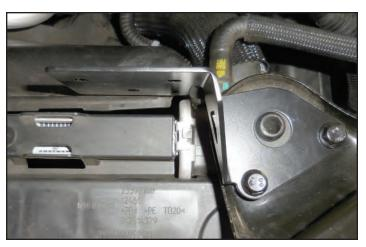
110. Torque the two M6x25mm bolts to 108 in-lbs.
