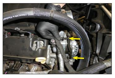
63. Pull the electrical wiring away from the throttle body to give room for intake manifold removal clearance.
