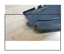
33. Use the template provided at the back of this manual to determine the location for the 1.75" diameter hole. Line up the template as shown here on the smooth underside of the passenger side. Use a center punch to transfer the hole location.
