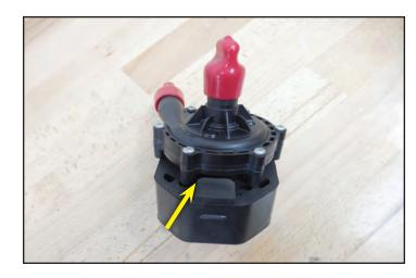
48. Install the rubber insulator on the bracket as shown. Ensure that it is fully engaged in the bracket.
