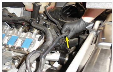
77. Remove the fastener holding the upper radiator hose at the arrow location. Try not to damage this plastic tie because it will be reused.
