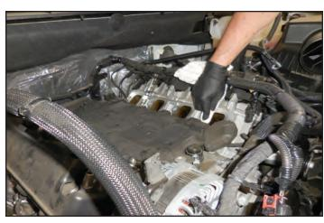
70. Seal the intake ports with tape (Shown here in blue).
