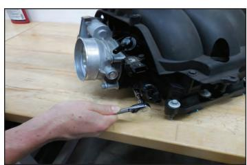
213. Remove the four bolts holding the throttle body to the OEM manifold. You may be using your OEM throttle body depending on how your calibration is being handled. These bolts will not be reused. If you have a 5.3L engine you will need to purchase a throttle body (GM Part# 12678223) Or Lingenfelter Ported LT5 95 mm Throttle Body | GM Gen V V8 Applications (LPE # L270046914)
