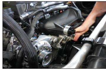
174. Gather the 8 provided M6x35mm bolts and apply Loctite Blue 242 to the ends as shown and apply blue Loctite 242 to the ends as shown. Gather the provided swivel socket shown below.
