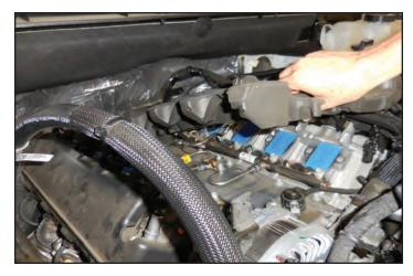
72. Remove the two plastic coil covers on the valve covers.
