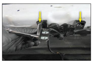
13. Disconnect the release cable from the hood latch.
