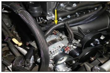
231. Re wrap the junction with electrical tape as shown.
