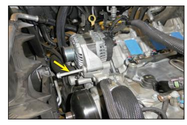
92. Loosen but do not remove the alternator mounting bolt on the opposite side with a 15mm socket wrench.
