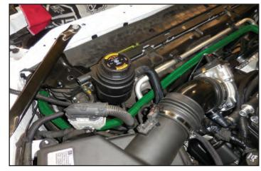
255. Here you can see the hose assembly from the last step being passed by the rubber shield.
