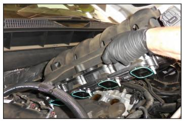
69. Clean the sealing surfaces on the heads using a cleaner like Simple Green.
