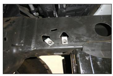
46. Mount the bracket with the two bolts as shown.
