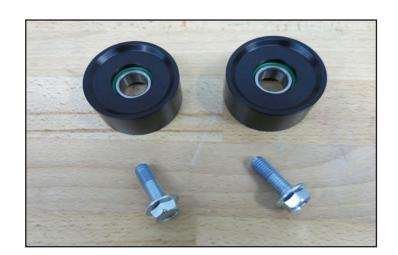
196. **Torque these two bolts to 25 ft- Ibs** after installing the idlers at the arrow locations.
