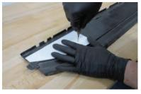
34. Use an electric drill with a hole saw to drill out the 1.75" diameter hole. Debur the hole after drilling.
