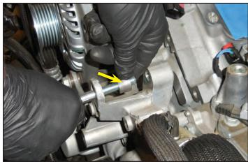
97. Gather the OE alternator bolt shown below along with the bushing that was removed in the last step. Insert the bushing into the provided bracket and tighten it in place with the bolt. See the next step for the bushing depth.
