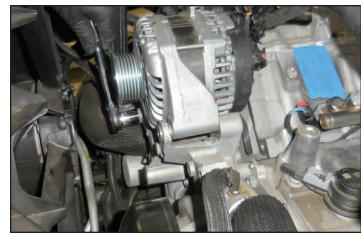
93. Use a prybar to lever the alternator up as shown.
