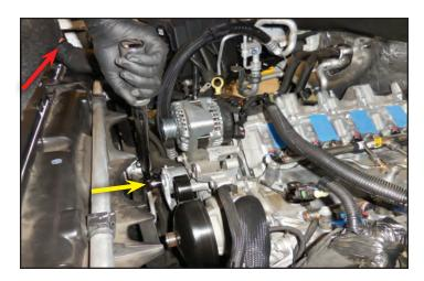
106. Gather the provided reservoir bracket, M6x25mm bolts, spacers, and M6 serrated flange nuts shown. If you don't have a top side creeper this could be done after Step 265 to avoid having to lean over the reservoir.
