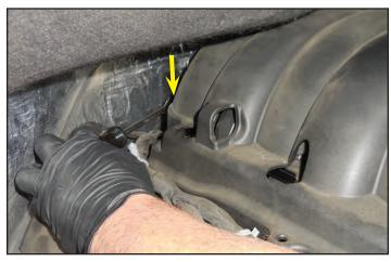
67. This image shows the location of the four tree connectors on the back of the intake manifold.
