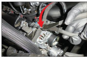
229. Unwrap the tape at the electrical harness junction shown.
