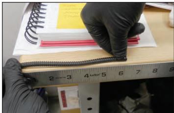
119. Peel back the yellow trigger wire through the OEM slit loom until it reaches the next tape junction. Cover the yellow wire with the wire loom from the last step and tape it in place at both ends. Continue the tape roughly 1" along the yellow wire.
