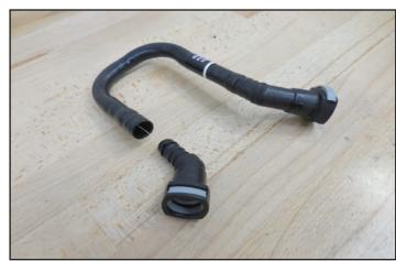
244. Gather the hose assembly, fittings and and Oetiker clamps shown. The fitting on the left was removed earlier from the OEM PCV hose. The other items are provided.
