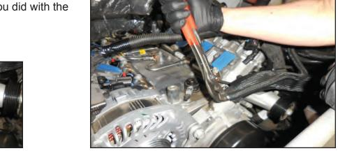
86. Gather the provided cable tie and clip shown. Remove the two tabs inside the clip.
