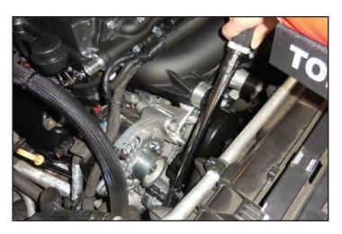
195. Gather thee two provided idler pulleys shown along with the two M10x30 mm bolts. Apply Loctite Blue 242 to the bolts Ensure that the side with the bearing surface and clip shown below is facing towards the engine when installed.
