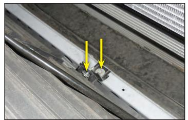
18. Remove the two bolts shown from the center bracket at the bottom of the grill.
