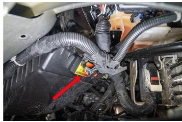
185. Zip tie the harness to the SCM-001 Module to the vehicle harness and trim the ends as shown.
