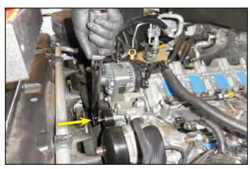
102. Apply Blue Loctite 242 to the M10x80mm bolt and install it into the provided tensioner.
