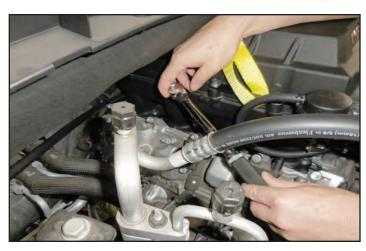
179. Ensure that the idler bracket sits flush with front of the supercharger at the arrow location
