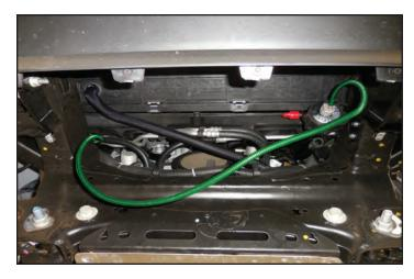
144. Ensure that there is enough slack to connect the cable from the previous step to the intercooler pump as you attach a provided cable tie with a tree connector on it (highlighted in green) at the location shown with the arrow here. This will provide a stress relief at the cable connection.
