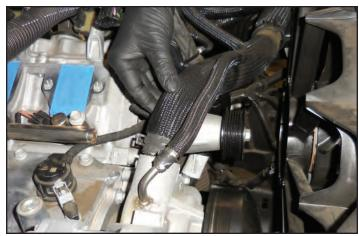
85. Rotate the clamp for the smaller hose so that the tabs face to the rear as you did with the other clamp.
