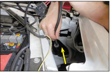
123. Continue to feed the gray plug and associated wiring through the hole in the last step until you have it near the headlight as shown.
