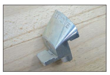
54. If using the tool shown in the last step you can rotate the crank with a 1/2 breaker bar and socket to allow the belt to ride up the ramp and derail itself.
