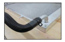
40. Insert the LTR in front of the radiator with the lower inlet pipe facing down and to the passenger side as shown with the arrow. At the same time have someone help you run the hose from the last step through the hole you made in the lower radiator panel earlier.
