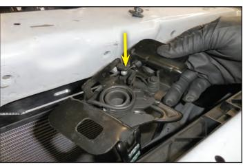
273. Plug in the electrical connector for the hood latch shown that is on the underside of the cross support for the radiator.
