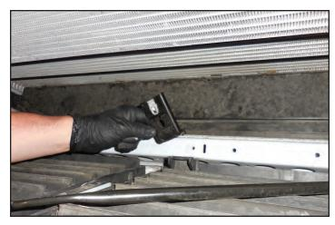
20. Clean the lower cross brace shown here in white with a cleaning product like Simple Green followed by rubbing alcohol to prepare it for the provided lower LTR bracket.
