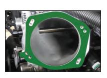
225. This photo shows the 95mm LT5 throttle body installed. **Apply Loctite Blue 242 to the ends of the provided M6x40 mm bolts as shown below.**
