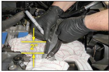
81. Release the clamp at the hose connection and pull the hose off .
