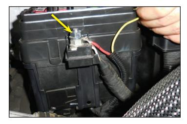
128. Remove the grounding bolt at the arrow location.
