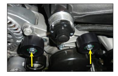
197. Gather the pulley and bolts shown. Apply Loctite Blue 242 to the four bolts as shown.
