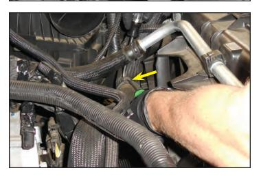
78. Cut the cable tie shown at the arrow. This will be replaced with a new one.
