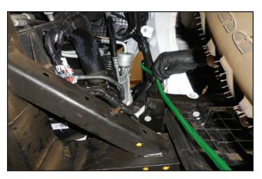
142. Route the end of the cable with the gray connector above the electrical harness shown at the arrow.
