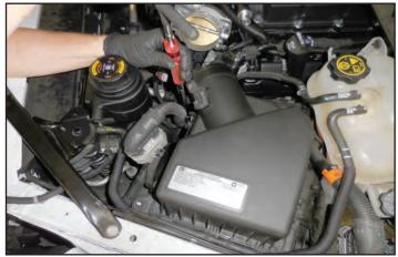
239. Gather the provided air inlet duct and the two hose clamps shown attached at the ends.
