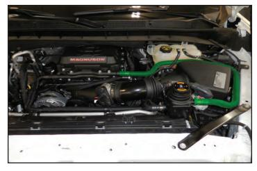
266. Secure the opposite end of the hose to the reservoir with a worm gear clamp. A worm gear clamp is necessary for proper sealing at the reservoir.
