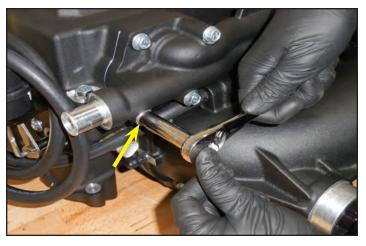
155. Apply some provided Loctite Blue 242 to the stud from two steps ago the stud from two steps ago as shown and install it at the location where the bolt was removed in the last step. It should thread in and bottom out by hand.
