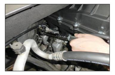
203. Reconnect the spark plug wires to the coils.
