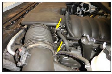
51. Rotate the air intake plenum as shown to reveal the fi nal mounting location.
