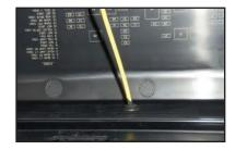
137. Remove the 10Amp fuse labeled as "#47 TCM IGN" at the location shown with the arrow.
