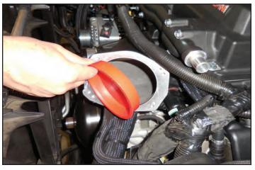
223. Remove the rubber adaptor from the end of the provided inlet duct.
