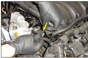
57. Press the release button on the EVAP hose connector and unplug it from the EVAP solenoid.
