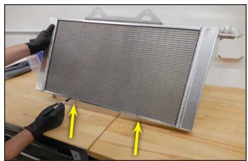
39. Install the hose assembly from the last step at the lower LTR inlet pipe and secure with the clamp from the last step.
