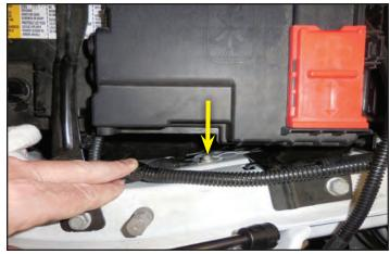
129. Route the ground wire for the intercooler pump harness as shown highlighted in green towards the bolt location from the last step.
