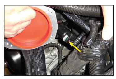
222. Remove the red cap at the supercharger inlet.
