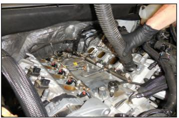
167. Use Simple Green or some other equivalent cleaner to wipe away any left over adhesive or debris. Apply some Tri-Flow or equivalent lubricant to a clean rag and wipe down the sealing surfaces.
