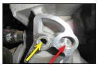
105. **Torque the tensioner to 25ft-lbs.** Make sure the boss stays properly aligned and tensioner is sitting flatbeforetorquing.
