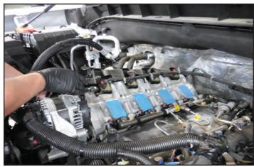
73. Remove the cable ties that are on the electrical harnesses. Several of these cable ties are shown below.
