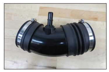
240. Install the air inlet duct between the throttle body and the airbox lid. Secure in place with the two hose clamps. Install first on the airbox lid and then lower the lid/duct assembly down, sliding the duct onto the throttle body. Secure upper air box lid to the lower air box lid.
