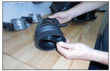
224. Install the provided gasket oriented as shown below highlighted in green.
