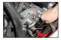
194. Torque the two alternator bolts shown in the last step with arrows to 25 ft-lbs.
