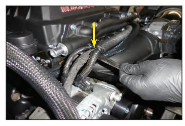
230. Cut 10 inches of 3/4" slit loom and install it at the arrow location.
