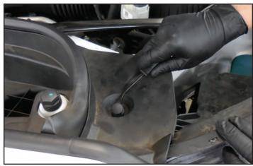
8. Remove the two T15 Torx bolts that hold the hood lever, and remove the lever.
