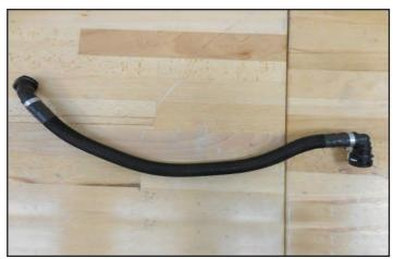
249. Install the hose assembly from the last step at the two arrow locations on the passenger valve cover and the air inlet duct. Ensure that the connections engage fully with a click. Gently pull on the connections to verify they are locked.
