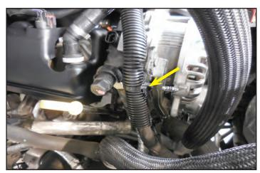
234. Plug in the electrical connection for the alternator and engage the lock.
