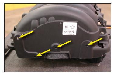
68. Carefully remove the intake manifold from the engine bay. Be careful not to drag the bolts across the sealing surfaces.
