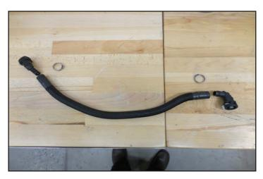
245. Install the provided 90 degree fi tting oriented on the hose as shown and secure with Oetiker pliers.
