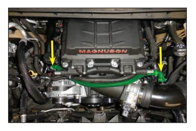
250. Secure the electrical harness to the PCV hose with a cable tie at the arrow location.
