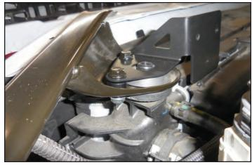
109. Ensure that the bracket is lined up with the radiator as shown.
