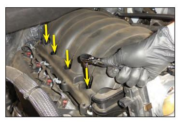
66. Be careful when pulling the manifold forward because the bolts can scratch the cylinder heads. Pull the intake manifold forward a bit to gain access to the wiring harness "tree" anchors that hold the harness to the back of the intake manifold. Use a screwdriver or tree clamp remover to unplug these trees from the OEM intake manifold.
