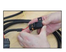
117. Remove the tape from the positive terminal side and remove one inch of the slit loom as shown.
