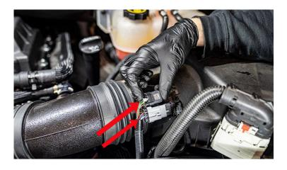
189. Secure the SCM-001 Module harness to the vehicle harness using zip ties.
