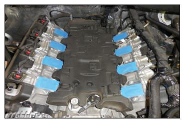
71. Remove the insulation pad from the engine valley. This will not be reused.
