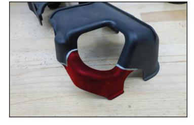
210. Trim the driver's side coil cover at the lines that were made in the last step.
