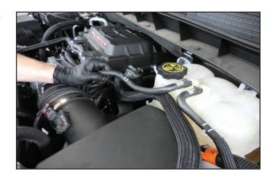
264. Install the hose from the last step at the supercharger charge air cooler outlet pipe with a provided hose clamp at the arrow location.
