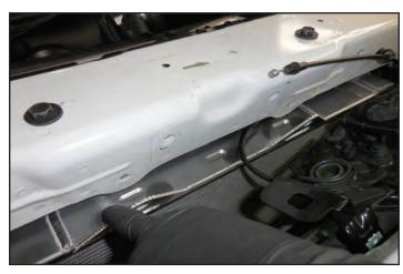
272. Reconnect the cable to the hood latch.
