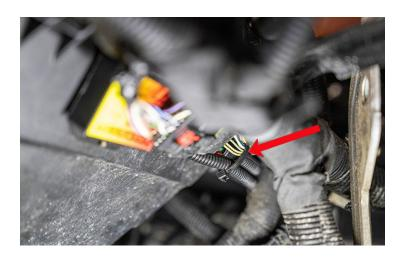
186. Plug in MAP Connector from SCM-001 harness to the MAP Sensor that was just installed on the airbox for Global B vehicles.
