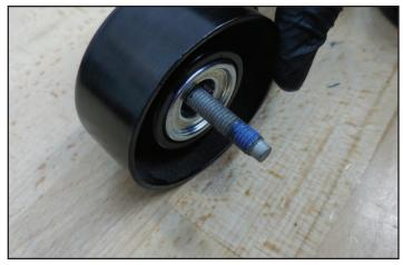
101. Install the idler and bolt from the last step into the location below the alternator shown with the arrow using a 13mm socket wrench and **torque to 18 ft-lbs.**
