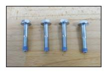
226. Torque the four M6x40 mm bolts in two stages with the final torque of 13o in-lbs
