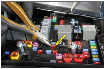
138. Install the "#47 TCM IGN" fuse on the metal terminal at the end of the yellow trigger wire.
