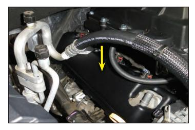
208. Route the vacuum line for the supercharger bypass behind the wiring for the coils as shown at the arrow.
