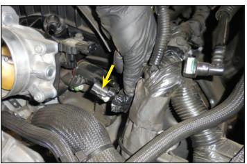
59. Disconnect the ETC connector from the throttle body. Depress the locking tab and pull the connector free.
