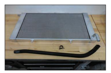
38. Mark the LTR on the front side to show the pin locations that are on the bottom side. Ensure that you mark over the top of the fl ange as shown in the photo below. This will aid in aligning the LTR later.
