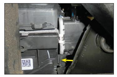
32. Tilt the cover at an angle and pull it free. The small photo shows the tab on the passenger side.
