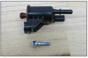
215. Install the EVAP solenoid in the location shown with the arrow using the provided M6x25mm bolt from the last step.
