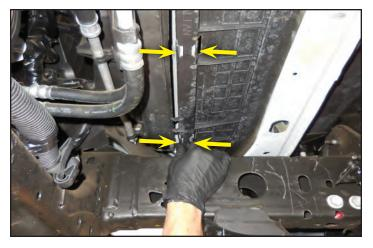
31. Release the tab on the passenger side shown for the cover from the last step.
