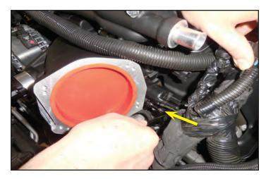
216. Plug in the electrical connection for the EVAP solenoid at the red arrow location for Global B vehicles. Ensure that you have secured the locking tabs on both fittings. Plug the factory engine harness into the MAP sensor at the red "X" location. For Global A vehicles, the factory MAP harness will plug into the factory MAP sensor mounted to the Lingenfelter Relocation Block.
