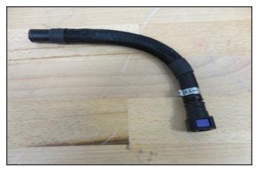
219. Preinstall the provided spring clamp shown below on the side of the hose from the last step without the fi tting and secure that end on the supercharger at the arrow location.
