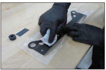
23. Peel the white cover off the double sided adhesive strip.
