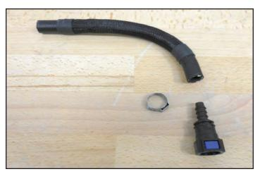
218. Slide the Oetiker clamp on the hose followed by the fitting. Use the Oetiker clamp pliers to crimp the end of the clamp as shown.
