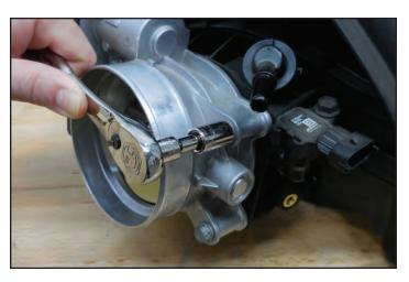
214. Gather the EVAP solenoid that you just removed and the provided M6x25mm bolt shown. Apply Loctite Blue 242 to the bolt prior to installation.
