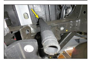
42. Line up the LTR using the marks that you made earlier with the holes in the bracket. This will allow you to line up the pins with the holes in the bracket. Verify the pins have aligned in the grommets by feel or with an inspection mirror.
