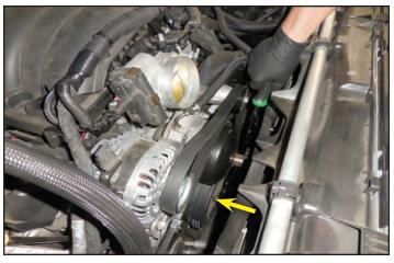
55. Remove the driver side PCV hose at the valve cover.
