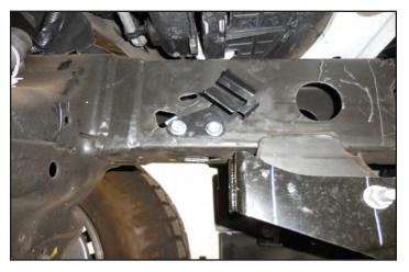
47. Install the pump in the rubber insulator with the orientation shown with the pump bolt location close to the rubber boss at the arrow.
