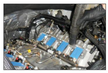
166. Remove the tape from the intake ports and vacuum them out to remove any debris.
