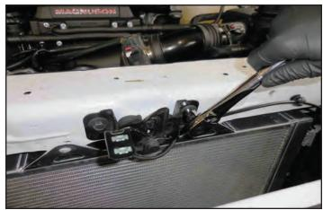
275. Reconnect the two large diagonal braces shown here with a 15mm socket wrench. Torque the two upper bolts to 25 ft-lbs and hand tighten the two lower bolts (one is shown below with the arrow.)
