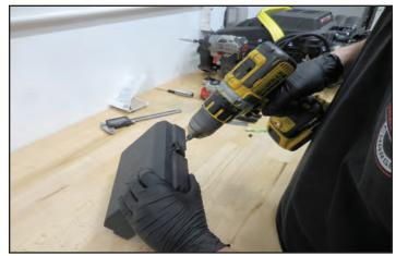
133. Use a step drill to open the hole up to 1/4" in diameter.
