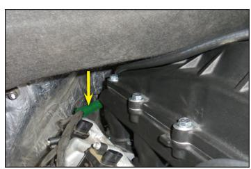
206. Plug in the electrical connections for all the coil packs on both sides.
