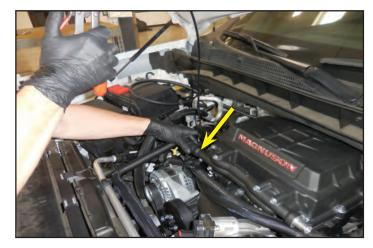
259. Here is a close-up of the inlet pipe hose connection to the supercharger charge air cooler.
