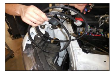
124. Run the other length of wire with the in-line fuse through the triangular hole shown with the arrow. This will be fed under the fuse box.
