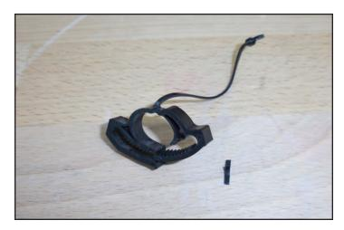
164. Reinstall the securing clip ensuring that it is now oriented to the side as shown with the arrow. This will allow the necessary clearance for the supercharger.
