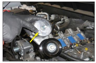
104. Line up the boss from the tensioner with the hole shown here at the red arrow in the photo below. The yellow arrow shows the location for the M10x80mm bolt. This is located below the alternator as shown in the photo to the right.
