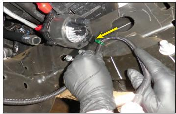
145. Hook the intercooler pump wire loom onto the two OEM connections shown with arrows if they are present. If these hooks are not present use some provided cable ties to secure this cable.
