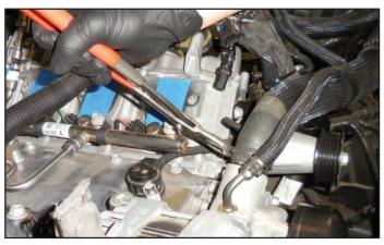
83. Reinstall the hose with the tabs for the clamp facing to the rear.
