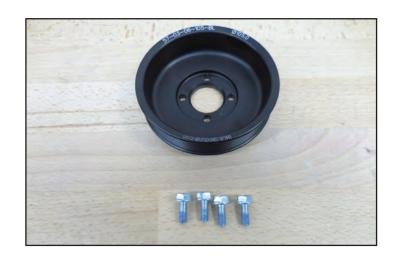
198. Use a strap wrench to hold the supercharger pulley in place while you **torque it to 108 in-lbs** using a 10mm socket wrench.
