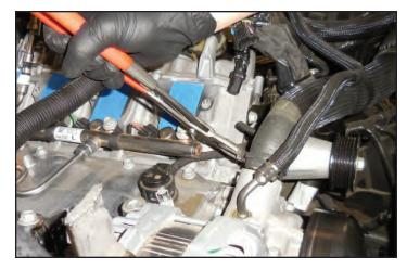
84. Slide the mesh down close to the clamp.
