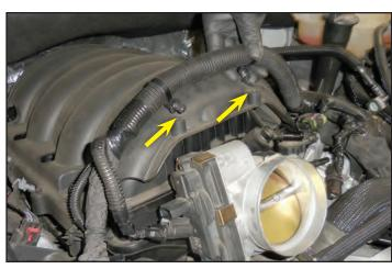
62. Remove the two cable tie fasteners shown with the arrows using a plastic pry bar.
