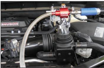
271. Remove the two bolts holding the LTR in place to allow the reinstall of the hood latch.
