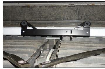
29. Reinstall the OEM center bracket that was removed earlier.
