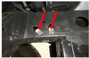
49. Mount the bracket with the two bolts as shown.
