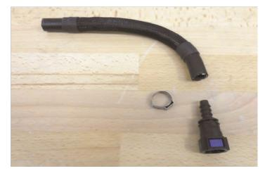
197. Slide the Oetiker clamp on the hose followed by the fitting. Use the Oetiker clamp pliers to crimp the end of the clamp as shown.
