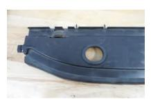
35. Reinstall the cover. Ensure that the tabs are lined up and the clips are locked in place.
