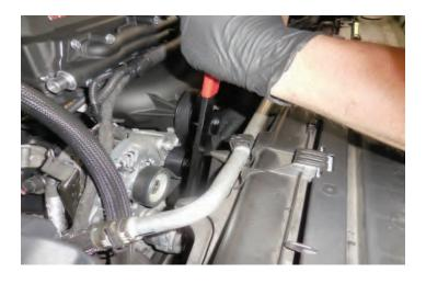
176. Remove the four supercharger lid bolts that are holding the two metal brackets that are securing the lift strap using a 12mm socket wrench. The 4 bolts will be reinstalled in the next step. Save the strap and brackets in case you ever need to remove the supercharger.
