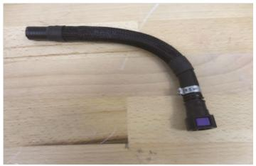
198. Preinstall the provided spring clamp shown below on the side of the hose from the last step without the fitting and secure that end on the supercharger at the arrow location.
