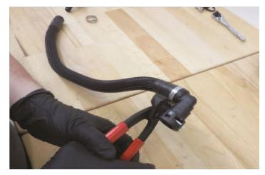
225. This photo shows the final location for the fitting from the last step.
