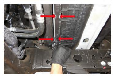
31. Tilt the cover at an angle and pull it free.
