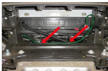
134. Ensure that there is enough slack to connect the cable from the previous step to the intercooler pump as you attach a provided cable tie with a tree connector on it (highlighted in green) at the location shown with the arrow here. This will provide stress relief at the cable connection.
