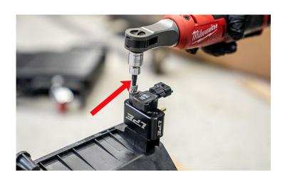
213. Install Lingenfelter SCM-001 Sensor Control Module onto the bottom of the airbox through the left front wheel opening. Make sure you remove the red tape, so you expose the sticky part of the double-sided tape that is already on the back of the module.
