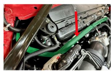
233. Here you can see the hose assembly from the last step being passed by the rubber shield.
