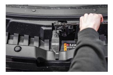
8. Remove the 9 plastic rivets holding the radiator cover. Remove the inner portion of the rivet first and then extract the outer portion.
