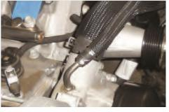
88. Secure the upper radiator hose in the same location as the OEM clip and secure the smaller hose to it.
