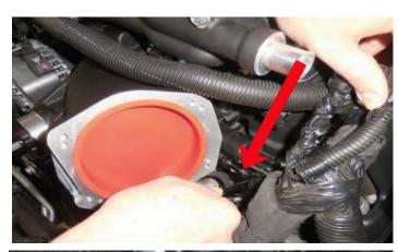
195. Plug in the electrical connection for the EVAP solenoid at the red arrow location for Global B vehicles. Ensure that you have secured the locking tabs on both fittings. Plug the factory engine harness into the MAP sensor at the red "X" location. For Global A vehicles, the factory MAP harness will plug into the factory MAP sensor mounted to the Lingenfelter Relocation Block.
