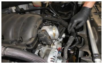
67. Remove the cable tie fasteners from the arrow locations. Repeat this process on the opposite side of the intake manifold.
