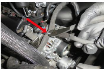
207. Install the power wire back onto the alternator and tighten the nut with a 17mm socket wrench.
