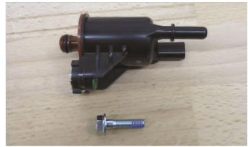
194. Install the EVAP solenoid in the location shown with the arrow using the provided M6x25mm bolt from the last step.
