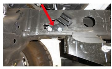
50. Install the pump in the rubber insulator with the orientation shown with the pump bolt location close to the rubber boss at the arrow.
