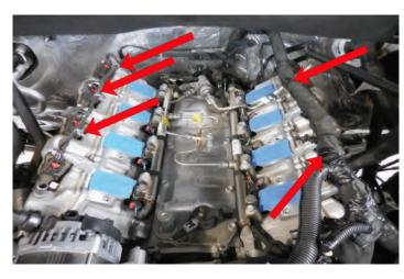
78. Unplug the spark plug wires for the back two coils on both sides of the engine. Mark the two rear coils on each side to ensure that they are installed in the original location later. Remove the two bolts holding each of the two rear coil packs on both sides of the engine using a 10 mm wrench.
