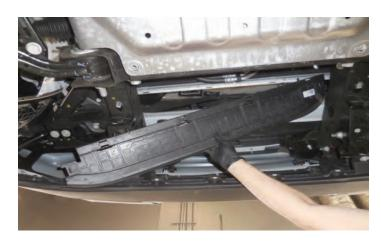
32. Use the template provided at the back of this manual to determine the location for the 1 3/4" diameter hole. Line up the template as shown here on the smooth underside of the cover on the passenger side. Use a center punch to transfer the hole location.
