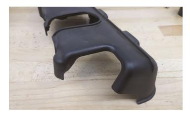
190. Reinstall the driver's side coil cover.
