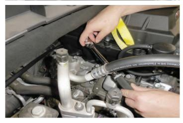
166. Ensure that the idler bracket sits flush with the front of the supercharger at the arrow location.
