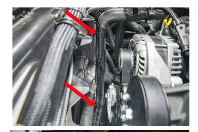
244. Use provided buddy clip and put the hose clip around the Reservoir to Pump hose and then zip tie to the LTR to supercharger hose.
