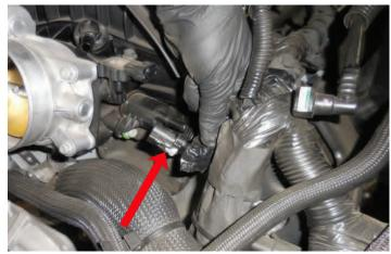
62. Disconnect the ETC connector from the throttle body. Depress the locking tab and pull the connector free.
