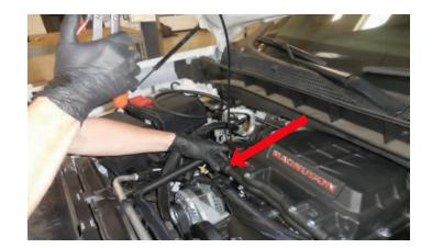
238. Here is a close-up of the inlet pipe hose connection to the supercharger charge air cooler.
