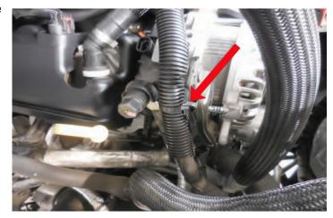
209. Plug in the electrical connection for the alternator and engage the lock.
