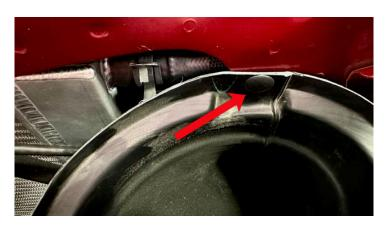
237. Attach the opposite end of the hose from the last step onto the inlet of the supercharger charge air cooler pipe at the arrow location.
