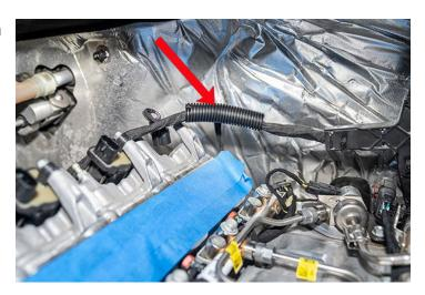
147. To remove the fuel line secondary clip: use a small screwdriver as a lever to pop the security clip from the fuel line at the red arrow location. Then push the clip in the blue arrow direction to remove it.
