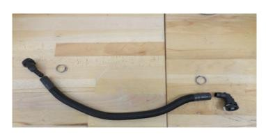
224. Install the provided 90-degree fitting oriented on the hose as shown and secure it with Oetiker pliers.
