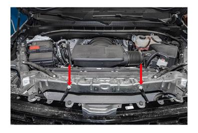
14. Loosen the bolt on the opposite side of the long diagonal brace from the last photo. Use a 15mm closed ratchet wrench to loosen 1/4 to 1/2 turn. **You do not need to remove this bolt**. The passenger side bolt is below the horns at the red arrow location.
