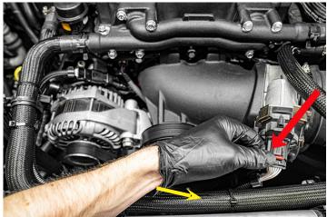
248. Secure the harness from the previous step to the coolant hose with the provided zip ties as shown in the photos.
