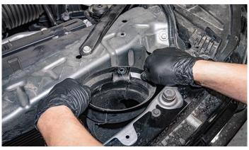
17. Pivot the long diagonal braces up and outward to get them out of the way as shown. This will give the necessary room to install the Low-Temperature Radiator (LTR) for the intercooler system
