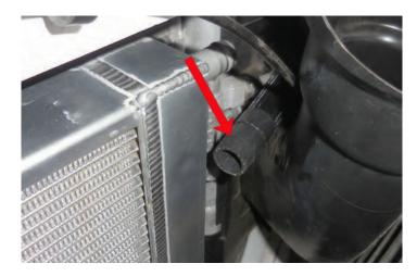
235. Attach the hose to the outlet pipe of the LTR at the arrow location with a provided spring clamp.
