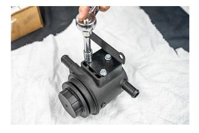
179. Install reservoir and bracket assembly on passenger side of supercharger. Apply Loctite Blue 242 to the fasteners and torque to 18 ft-lbs.
