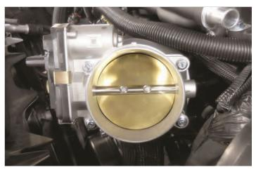
205. Torque the four M6x40 mm bolts in two stages with the final torque of 130 in lbs.
