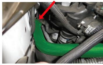
234. After the hose passes through the rubber shield it will be seen through the front like this.
