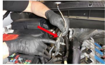
127. Route the yellow trigger wire through the hole that was made in the fuse box cover. Make sure the grommet is fully seated on both sides.
