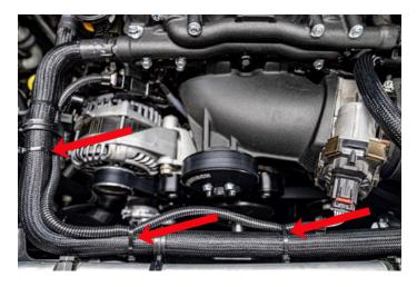
249. Use the supplied zip ties to secure the hose to the A/C line.
