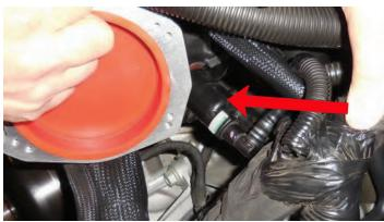
201. Remove the red cap at the supercharger inlet.
