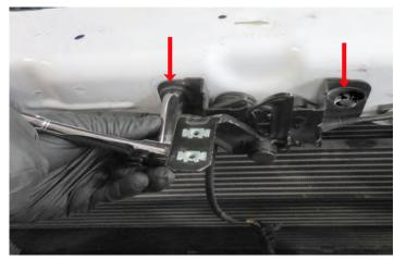
13. Remove the two bolts holding the diagonal brace shown with red arrows with a 15mm socket wrench.
