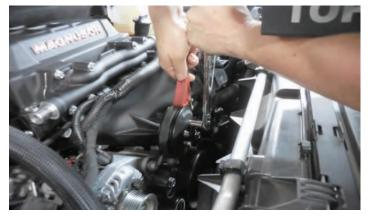
175. Install the belt following the diagram at the back of this manual. Connect a belt tensioner wrench or 1/2" breaker bar at the tensioner and rotate it counterclockwise. The last pulley to place the belt over should be the smooth pulley that was installed on the right side three steps ago.
