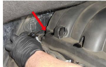
70. This image shows the location of the four tree connectors on the back of the intake manifold.
