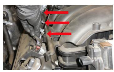
68. Remove the 10 bolts holding the intake manifold in place using a 10mm socket wrench.
