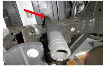
41. Line up the LTR using the marks that you made earlier with the holes in the bracket. This will allow you to line up the pins with the holes in the bracket. Verify the pins have aligned in the grommets by feel or with an inspection mirror.
