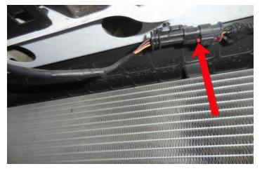
11. Disconnect the electrical connection for the hood release and at the same time remove the anchor holding the connector to the frame.
