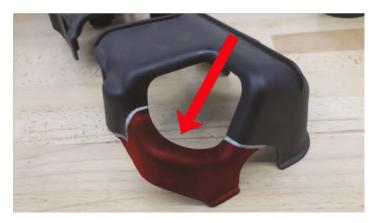
189. Trim the driver's side coil cover at the lines that were made in the last step.
