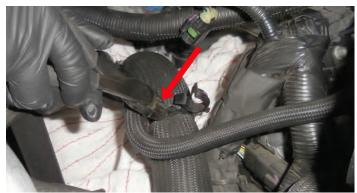
82. Pull the mesh away from the end of the hose connection. This will allow room for the hose to be cut. Wrap the connection location with rags as shown to catch any coolant.
