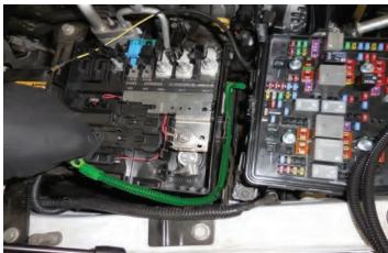
121. Place the ground wire eyelet from the intercooler harness on top of the OEM ground and reinstall the bolt from two steps ago.
