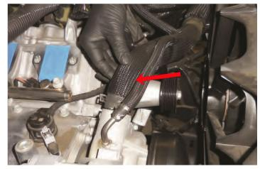
87. Rotate the clamp for the smaller hose so that the tabs face to the rear as you did with the other clamp.
