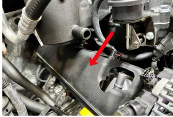
187. Route the vacuum line for the supercharger bypass behind the wiring for the coils as shown at the arrow.
