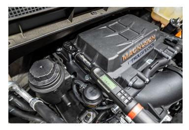
180. Apply Loctite Blue 242 to the 2 remaining lid bolts from step 197. Reinstall the bolts in their original location and torque them to 18 ft-lbs.
