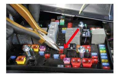
129. Install the "#47 TCM IGN" fuse on the metal terminal at the end of the yellow trigger wire.
