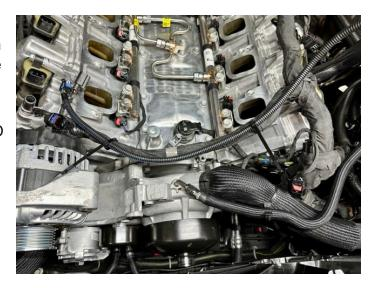
Performance Cold Air Intake shown below install the included MAP Relocation Block to the lower tab of the intake box tab with the supplied lock nut, washer, and M6x30 bolt as shown then install the MAP Sensor from the original intake with the included M6x25 bolt and washer. Be sure to use Loctite on the threads. DO NOT OVER-TIGHTEN. If you DO NOT have the GM Performance Cold Air Intake, the MAP Relocation Sensor Block will be installed later in the manual.
