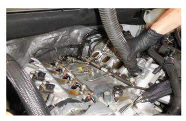
153. Lay the engine harness between the water pump and valley cover as shown.
