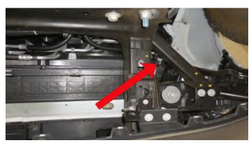
5. Attach a hose at the red arrow and loosen the drain plug at the yellow arrow.
