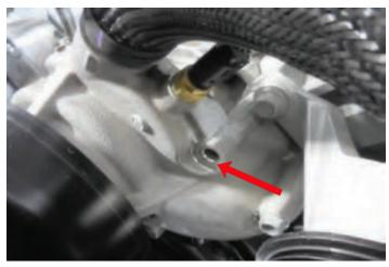
96. Use the provided bolt shown below to press out the bushing as shown by the arrow.
