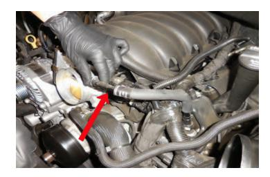
59. Release the secondary locking tab, shown at the arrow, on the MAP sensor electrical connection and unplug it.
