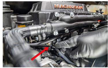
216. Plug in the IAT Sensor Connector from the Lingenfelter SCM-001 Sensor Control Module to the Factory MAP Sensor previously installed on the Lingenfelter Performance Engineering MAP Relocation Block. The GM MAP Sensor and MAP Sensor Relocation Vacuum Hose will not be used.
