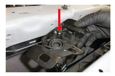
45. Plug in the electrical connector for the hood latch shown that is on the underside of the cross support for the radiator.
