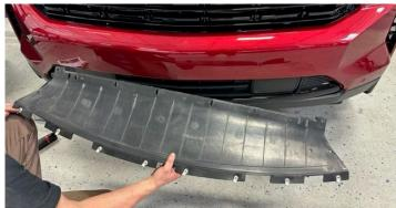
30. Raise the vehicle and remove the plastic cover shown by pinching at three areas and pulling down. Two of the areas are shown here with pairs of arrows.
