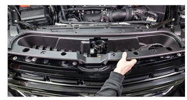
10. Locate the electrical connector for the hood latch shown that is on the underside of the cross support for the radiator.
