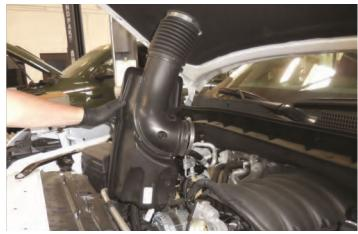
55. Pull the air intake plenum to the passenger side to remove it from the vehicle. This will not be reused.
