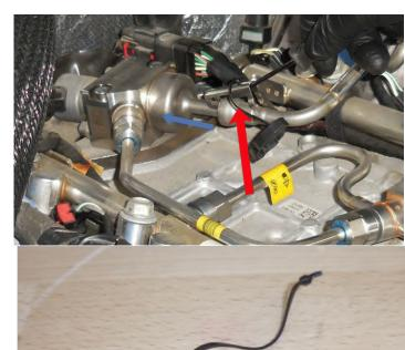
149. Reinstall the securing clip ensuring that it is now oriented to the side as shown with the arrow. This will allow the necessary clearance for the supercharger.
