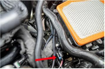
217. Plug the MAF Sensor Connector from the Lingenfelter SCM-001 Sensor Control Module to the connector between the vehicle harness and the MAF Sensor as shown in the photos.
