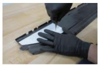
33. Use an electric drill with a hole saw to drill out the 1.75" diameter hole. Debur the hole after drilling.
