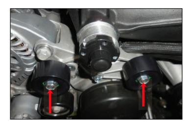
173. Gather the pulley and bolts shown. Apply Loctite Blue 242 to the four bolts as shown.
