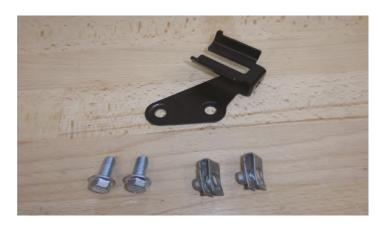
48. Install the two clip nuts in the locations shown.
