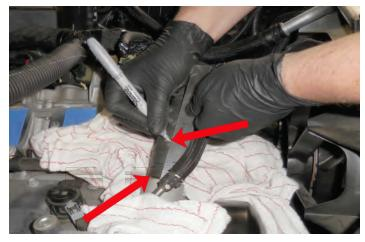
84. Release the clamp at the hose connection and pull the hose off.
