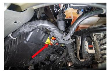
214. Tighten and trim any previously installed zip ties on the harness coming out of the Lingenfelter SCM-001 Sensor Control Module to the vehicle harness.
