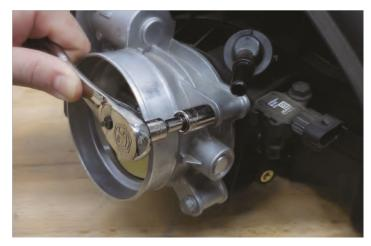
193. Gather the EVAP solenoid that you just removed and the provided M6x25mm bolt shown. Apply Loctite Blue 242 to the bolt prior to installation.
