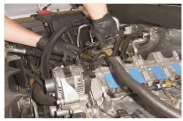
92. Remove the alternator bolt shown at the arrow using a 15 mm socket wrench.
