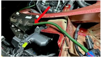
115. Run the other length of wire with the in-line fuse through the triangular hole shown with the arrow. This will be fed under the fuse box.
