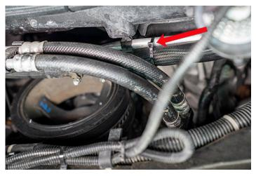
250. Here is a photo of the completed routing of hoses and cable ties under the SUV.
