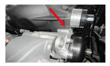
167. Gather the provide M8x40mm bolts shown below and apply Loctite Blue 242 to the ends. Install these two bolts at the locations shown with arrows below the supercharger input shaft. You may need to loosen the other 3 slightly to get these to align.
