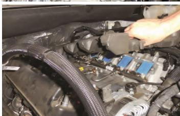
75. Remove the two plastic coil covers on the valve covers.
