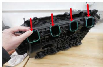
143. Install the 8 gaskets from the last step into the bottom of the supercharger as shown here. Ensure that the tab lines up with the notch in the top edge at the locations shown with yellow arrows.
