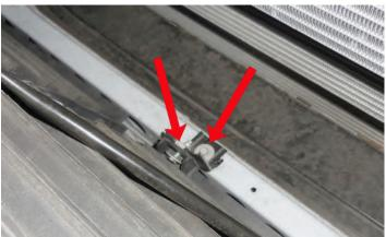
20. Clean the lower cross brace shown here in white with a degreaser followed by rubbing alcohol to prepare it for the provided lower radiator bracket.
