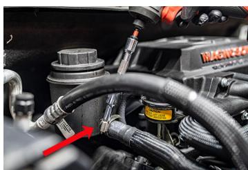
246. Use the provided buddy clip to secure the reservoir to the pump hose and A/C line.
