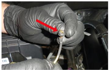
126. Slide the provided grommet from the last step over the yellow trigger wire just above the tape that was added in a previous step at the arrow.
