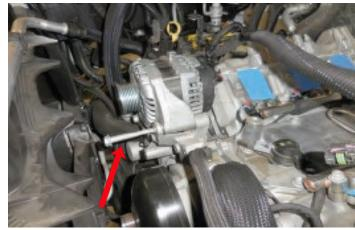
93. Loosen but do not remove the alternator mounting bolt on the opposite side with a 15 mm socket wrench.
