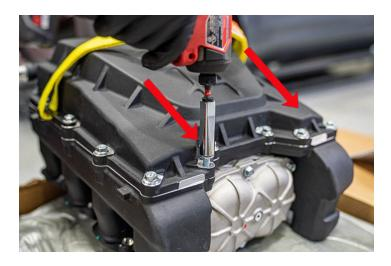
139. Gather the bracket, clamp, zip tie, and hose, and secure the bracket to the supercharger. Apply Loctite Blue 242 to the fastener and torque to 18 ft-lbs.
