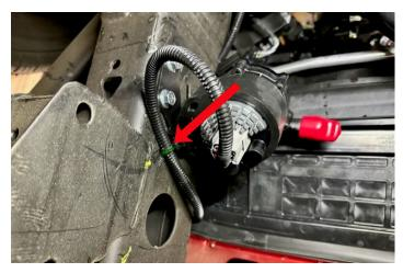
135. Attach the hose that comes from the lower LTR inlet pipe to the output of the intercooler pump at the arrow and secure it with the provided spring clamp.
