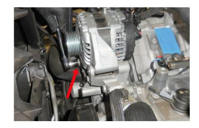
94. Use a prybar to lever the alternator up as shown.
