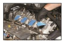
152. Use a degreaser to wipe away any leftover adhesive or debris. Apply some Tri-Flow or equivalent lubricant to a clean rag and wipe down the sealing surfaces.
