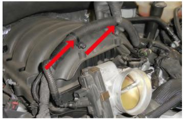
65. Remove the two cable tie fasteners shown with the arrows.
