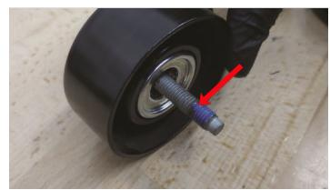
106. Install the idler and bolt from the last step into the location below the alternator shown with the arrow using a 13 mm socket wrench and torque to 18 ft-lbs.
