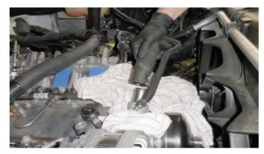
85. Cut the hose at the 2" mark that was made earlier. Reinstall the hose with the tabs for the clamp facing the rear.
