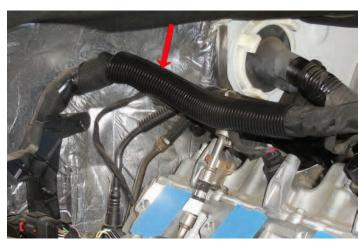
146. Cut the provided 3/4" slit loom to 4" long then install the slit loom from the last over the wiring harness at the arrow location.
