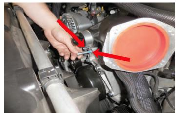
168. Torque all the bolts at the idler bracket according to diagram at the back of this manual.
