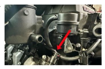
188. Mark the driver's side coil cover at the silver lines shown here. The area to be removed is highlighted in red.
