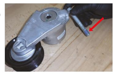
102. Once you have installed the bolt from the last step you will see the boss at the back of the tensioner shown with the arrow.
