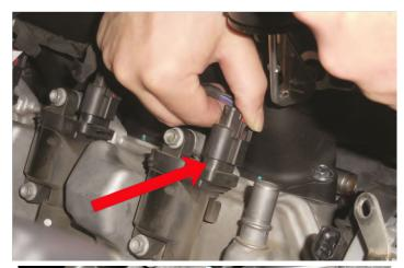
186. Reinstall the coil covers on the passenger side.
