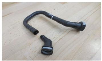
223. Gather the hose assembly, fittings and Oetiker clamps shown. The fitting on the left was removed earlier from the OEM PCV hose. The other items are provided.
