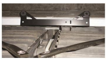
28. With a 10 mm socket, reinstall the OEM center bracket and fastener that was removed earlier in step 19.
