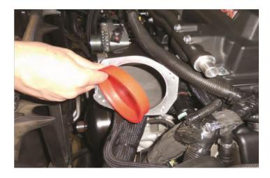
202. Remove the rubber adaptor from the end of the provided inlet duct.
