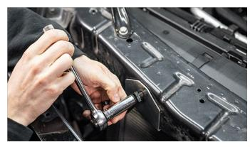
43. Reinstall the horn bracket and horns.
