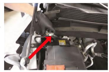
2. Remove the front fender well liners from the vehicle. On the left front side of the wheel, you will see the ECM module with three electrical connectors. Remove the connectors and then remove the module from the bracket.
