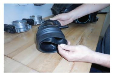
203. Install the provided gasket oriented as shown below highlighted in green.
