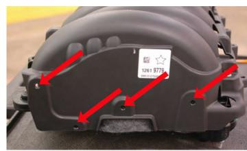
71. Carefully remove the intake manifold from the engine bay. Be careful not to drag the bolts across the sealing surfaces.
