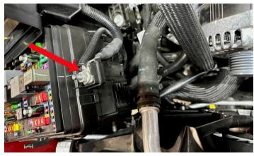
119. Remove the grounding bolt at the arrow location.
