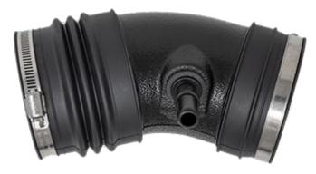
221. Install the air inlet duct between the throttle body and the airbox lid. Secure in place with the two hose clamps. Install first on the airbox lid and then lower the lid/duct assembly down, sliding the duct onto the throttle body. Secure the upper air box lid to the lower air box lid.
