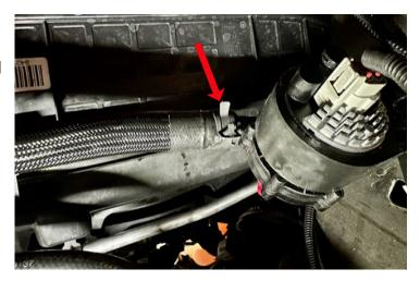
136. Use the two provided edge mount cable ties and secure the "LTR to Pump Hose" to the lower plastic radiator panel that was removed earlier at the arrow locations.
