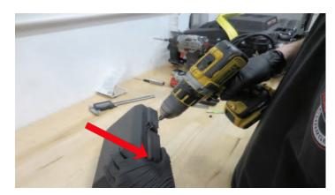
124. Use a step drill to open the hole up to 1/4" in diameter.
