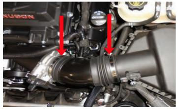
222. Gather the OEM PCV hose shown and carefully remove the fitting shown. Ensure that you do not cut into the barbed fitting when cutting through the plastic hose.
