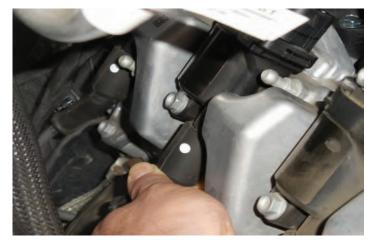
184. Reconnect the spark plug wires to the coils.
