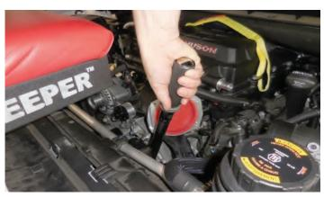
169. Rotate the alternator into the new idler bracket and insert the stock bolt.
