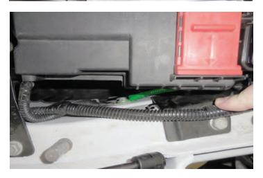
122. Make sure you are referencing the lock tab/side that faces the rear of the vehicle. Mark a cross on the back of the fuse box lid indicating a location .5" from the release lever and level with it as shown here.
