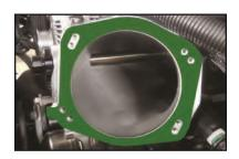
204. This photo shows the 95mm LT5 throttle body installed. Apply Loctite Blue 242 to the ends of the provided M6x40 mm bolts as shown below.
