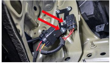
117. Route the red positive wire, and yellow trigger wire under the fuse box.
