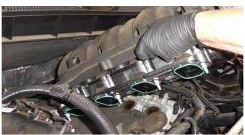
72. Clean the sealing surfaces on the heads using a degreaser.
