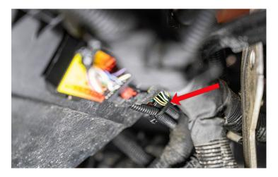
215. Plug in the IAT Connector from the Lingenfelter SCM-001 Sensor Control Module to the sensor on the front passenger side of the superchargER.
