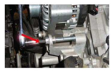
98. Gather the OE alternator bolt shown below along with the bushing that was removed in the last step. Insert the bushing into the provided bracket and tighten it in place with the bolt. See the next step for the bushing depth.
