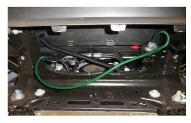
133. Hook the intercooler pump wire loom to the two OEM connections shown with arrows if they are present. If these hooks are not present, use some provided cable ties to secure this cable. Remove the two red caps from the intercooler pump.
