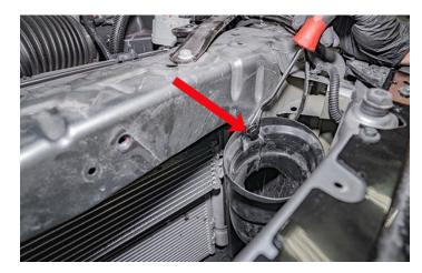
19. With a 10 mm socket and extension remove the two bolts from the center bracket at the bottom of the grill and remove the bracket as shown.
