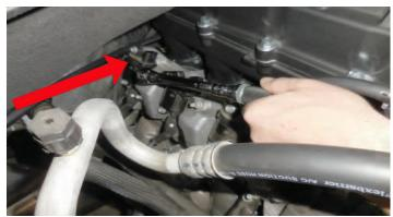
185. Plug in the electrical connections for all the coil packs on both sides.
