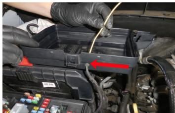
128. Remove the 10-amp fuse labeled as "#47 TCM IGN" at the location shown with the arrow.
