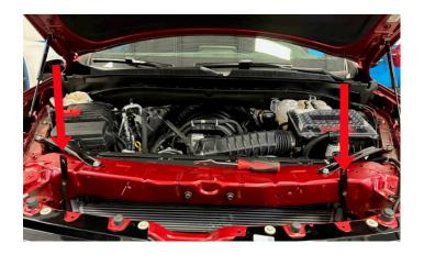
18. Remove the push pin holding the air inlet duct to structure do not remove the air inlet duct.
