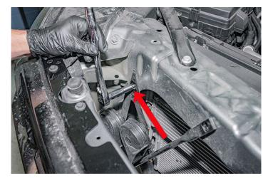
16. Remove the air inlet duct.
