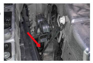
15. With a 10 mm socket remove the horn bracket, and horn.
