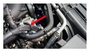
247. Gather the provided electronic throttle control (ETC) cable extension shown below. Secure the harness first to the body side connector and then to the throttle body as shown with the red arrows. Route the harness along the coolant hose as shown with the yellow arrow.
