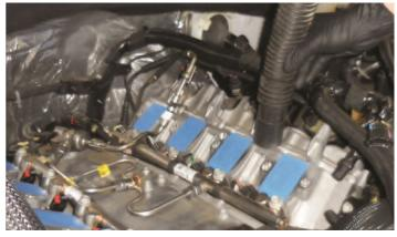
151. Remove the tape from the intake ports and vacuum them out to remove any debris.
