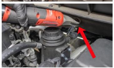
182. Properly pull tight and secure the zip ties holding the coolant hose to the bracket at the rear of the supercharger. Be sure to snip off the tails of the zip ties.
