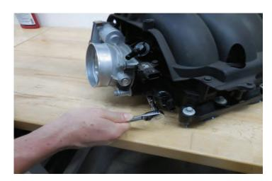
192. Remove the four bolts holding the throttle body to the OEM manifold. You may be using your OEM throttle body depending on how your calibration is being handled. These bolts will not be reused. If you have a 5.3L engine you will need to purchase a throttle body (GM Part# 12678223).
