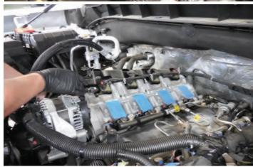
76. Remove the cable ties that are on the electrical harnesses. Several of these cable ties are shown below.
