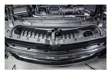
254. Reinstall the lower closeout panel in reverse from step 29.
