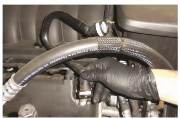
53. Using a 7 mm nut driver or a flat blade screwdriver, loosen the clamps at the two arrow locations.
