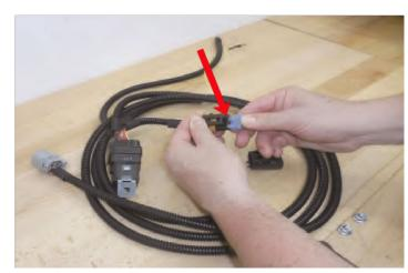
109. Remove the tape from the positive terminal side and remove one inch of the slit loom as shown.
