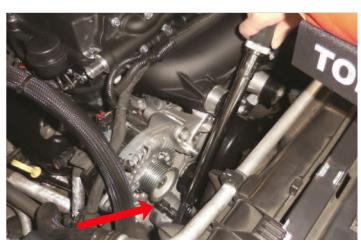
170. Torque the two alternator bolts shown in the last step with arrows to 25 ft-lbs.
