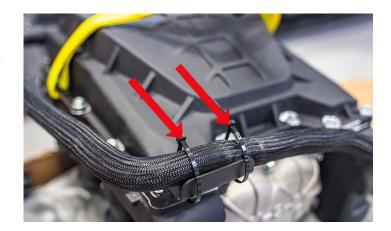
141. Install the hose and clamp onto the supercharger.
