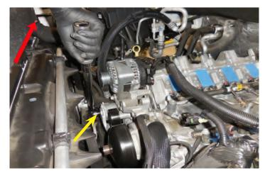
105. **Apply Blue Loctite 242** to the threads of the pre-installed bolt on the idler.
