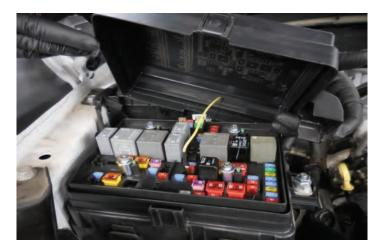
130. Reinstall the fuse at its original location.
