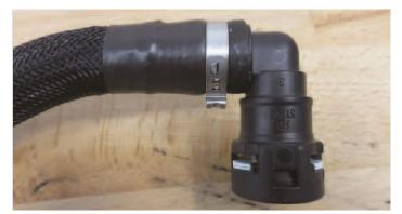
226. Secure the OEM 45-degree fitting on the opposite side as shown with another Oetiker clamp.
