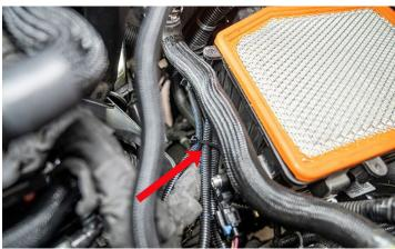
219. Install the Lingenfelter Performance Engineering Intake Air Temperature Relocation Harness to the MAP Sensor Harness as shown.
