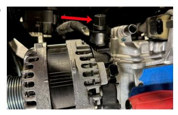
91. Remove the alternator positive cable terminal.
