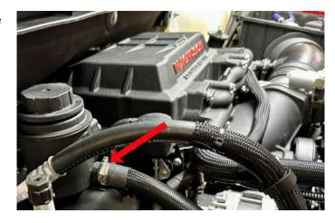
242. Attached both provided edge biter clips as shown.
