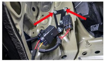
114. Run the gray plug from the intercooler pump harness highlighted in green through the opening shown.
