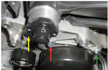
165. Use the socket from three steps ago with a 1/4" drive long extension to tighten the 8 bolts that were just installed. Start out by spinning these bolts in place by hand without a wrench. Follow the torque order given at the back of this manual and gradually work your way up to the **final torque of 120 in-lbs.** Spin the supercharger at the input shaft to ensure that it is rotating freely after torquing the bolts.
