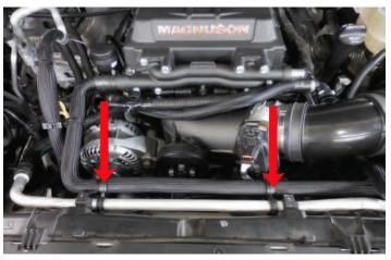
241. Take the Reservoir to Pump coolant hose and secure end to reservoir with worm gear clamp. A worm gear clamp must be used to provide a proper seal.
