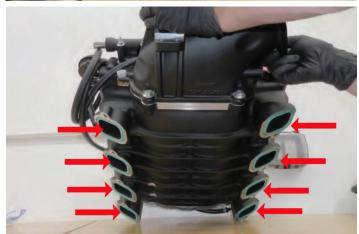
144. If you need to install a boost reference port, you should do so now at the rear left of the supercharger shown at the arrow.
