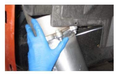
30. With one person guiding the top of the tank up, slide the tank in through the bottom and line up the bolt holes to the brackets on the bottom.
