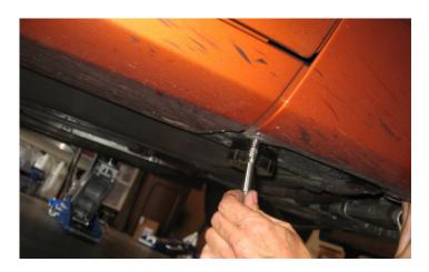
10. With the liner removed, locate the bolt on the bottom of the fender directly under the front of the passenger side door. Remove this bolt using a 7 mm socket (this is needed to push the fender out of the way slightly to make way for the removal and installation of the tanks).
