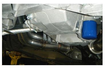
5. After all of the oil has drained out, replace the oil filter with filter part number UPF48R (PN 12626224) and torque the filter to 18lb-ft (25 Nm). Replace both drain plugs and torque both of them to 18lb-ft (25 Nm).
