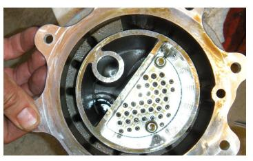
21. Inspect the top of the tank for damage or corrosion. Be sure to wipe the mounting surface clean before installation on the new tank.
