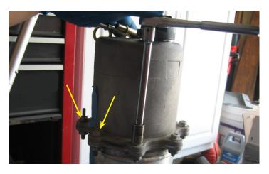
20. Using a 13 mm socket and extension, remove the eight (8) nuts and bolts on the tank to separate the top and bottom of the tank. You will need a deep well socket or an open end wrench to remove the two bolts (in which the tape is in between) indicated to the left.
