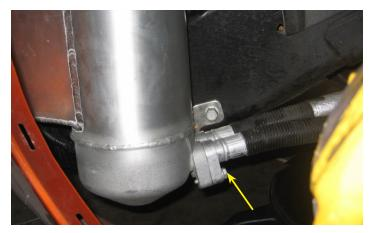
32. Install both oil lines and, using a 13 mm socket, torque the two (2) bolts to 16 lb-ft (22 Nm).
