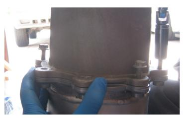
27. After aligning the tanks, using a 13 mm socket and extension, torque the eight (8) bolts to 18 lb-ft in an 8-bolt star pattern (25 Nm). Remember that you will need a deep well socket to torque the longer bolts. The tape used to mark the tank should be in between the two (2) longer bolts.
