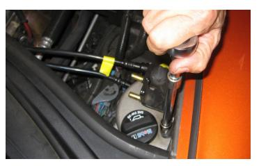
13. Using a 10 mm socket and extension, remove the bolt on the top of the tank located directly between the oil cap and the fender.
