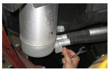
15. Remove the oil lines from the bottom of the tank by using a 13 mm wrench to remove the two bolts directly under the oil lines. Be sure to have an oil pan below to catch any residual oil that may drain out of the tank.
