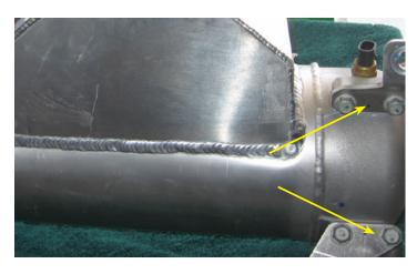
22. Using a 13 mm socket, remove the two (2) mounting brackets from the old tank by removing the four (4) bolts on the brackets. Install the old brackets to the new tank and torque to 18 lb-ft (25 Nm).
