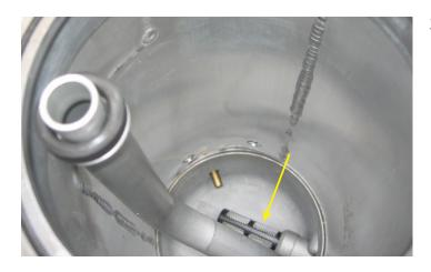
24. Remove the oil screen from the old tank by gently twisting, wiggling, and pushing the screen towards the outside. Install the oil line screen onto the new tank by pushing the screen into the inlet bore from the outside of the tank until the locking tabs locate in the grooves.
