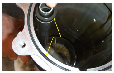
25. Inspect the O-ring and engine oil tank gasket from your old tank to your new tank
