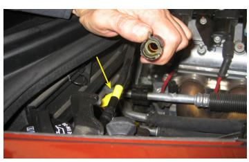
11. Mark one of the vapor lines as well as its respective port with a piece of tape (or equivalent) and remove the vapor lines from the top of the tank. This is done by pushing the small tabs on the ends of the lines clockwise and pulling outward.
