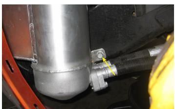
31. Using a 15 mm socket, bolt the two (2) bottom brackets of the tank to the frame rail and torque to 27 lb-ft (36 Nm).
