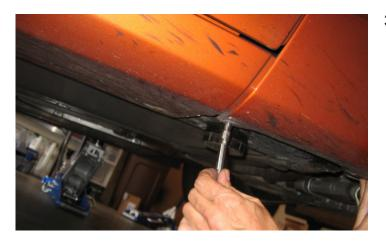
37. Position the fender back into place and, using a 7 mm socket, install the bolt that was taken off in step 9.
