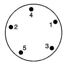
40. Torque the wheel lug nuts to 100 lb-ft (140 Nm). Be sure to use the proper torque sequence for a 5 bolt wheel. Remove jack and jack stands and enjoy your new oil tank.
