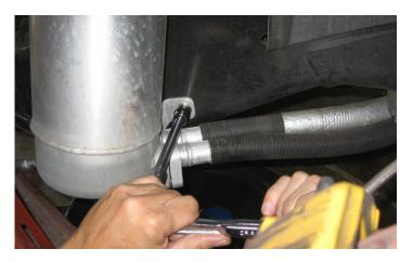
16. At this point in the installation it is recommended to have another person to help remove and place the oil tank. While one person is holding the top of the tank, remove the two (2) 15mm bolts on the mounting bracket on the bottom of the oil tank that secure the tank and bracket assembly to the vehicle.
