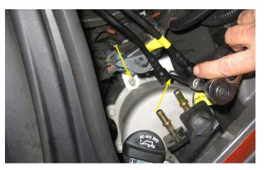
12. Using a 10 mm socket and extension, remove the two bolts from the bracket holding the middle of the tank. Be careful not to drop the two bolts once you remove them.
