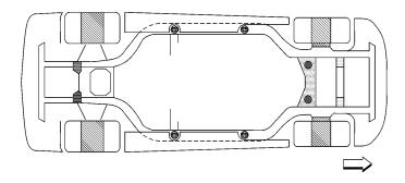
2. Raise the vehicle with a vehicle hoist or a jack and jackstands. Be careful to follow the GM lifting procedures on the Z06 Corvette due to the aerodynamic components being easily damaged and the low ride height of the vehicle.
