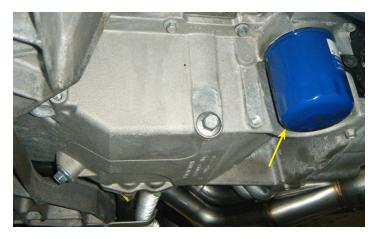
4. Allow all oil to drain out of the oil pan.
