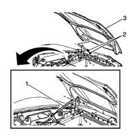
1. Open the hood of the vehicle. If you have been driving the vehicle, allow the vehicle to cool down for a few hours before starting this installation.
