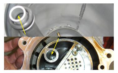
26. Line up the holes on the top and bottom tank and also make sure that the bolt holes line up correctly. Line up the tape on the top tank with the oil line fittings on the new lower tank. Remember your marking that you made on your old lower tank and compare it with the new tank.
