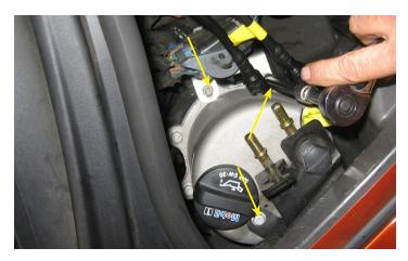
33. Using a 10 mm socket, install the three (3) bolts on top and torque each to 89 <u>lb-in</u> (10 Nm).
