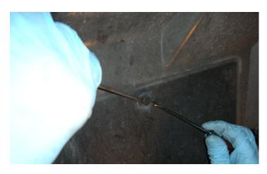
38. Push the liner back into place and replace the two (2) push pins that were taken out by inserting them with the pin in the out position, and once inserted into the hole push the pin into the hole and it will lock into place.
