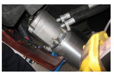
29. Place the tank inside of the passenger front fender with the tank's expanded oil volume section pointing towards the rear of the vehicle.
