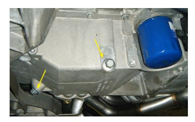
3. Using a 15 mm socket, remove **both** drain plugs from the oil pan to drain the oil.
