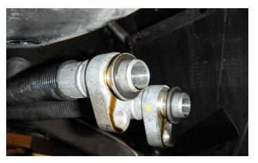
28. Replace the two oil seals on the bottom oil tank lines with the supplied oil seals (GM part # 15217990). Make sure that the rubber side of the seals are facing toward the tank.
