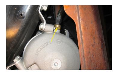
14. On the bottom of the tank remove the oil temperature sensor by first disconnecting the harness and then unscrewing the sensor using a 19 mm wrench. Inspect the sensor for damage as you will be using this sensor again.
