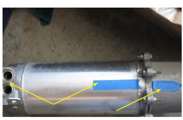
19. Mark the top and bottom portion of the tank as shown. You will use this to reference putting the assembly back together correctly, notice the location of the oil line fittings on the stock lower tank.
