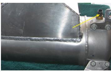
23. Using a 19 mm socket, replace the oil temperature sensor and tighten to 15 lb-ft (20 Nm) of torque.
