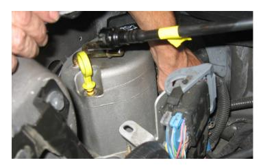
18. Remove the tank from the car by having one person pull the tank down through the bottom of the fender while the other person carefully moves the tank out of the way of the wiring harness as well as any other obstructions.
