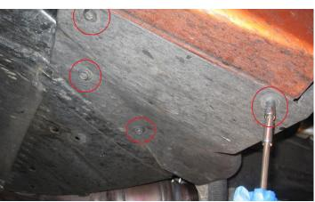
39. Using 7 mm and 10 mm sockets, replace the four (4) bolts that were removed from the fender liner.
