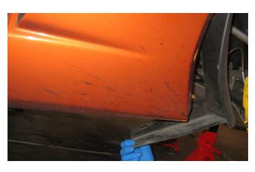
9. The liner is attached to the fender with metal push-clips. Start with the lower portion of the liner and pull the liner strait out of the fender.
