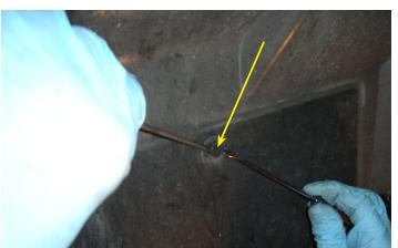
8. Remove the two (2) plastic push pins from the side of the fender liner by using a fork pry tool. Pull out on the center (smaller) pin until it pops out, then remove the whole push pin.
