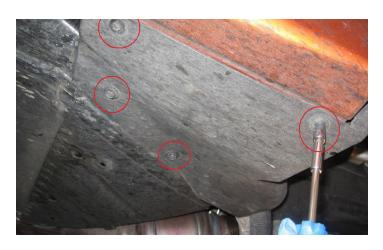
7. Using a 7mm socket for the outer bolts and a 10 mm socket for the inner bolts, remove the passenger front fender liner.
