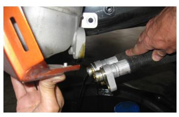
17. Move the bottom of the tank out of the way and remove the oil lines. Be sure to point the lines into the oil pan as residual oil will most likely drain out.
