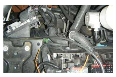
34. Pull the orange wire from the remaining bundle of wires in the fan relay harness. Pull the wire out so that it exits the plastic convoluted loom near the fuse relay center.
