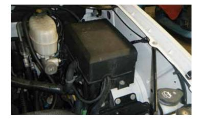
19. Remove the plastic cover from the main fuse and relay center.
