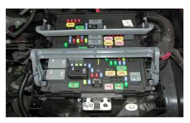
20. Un-clip the gray locking tabs securing the fuse block and remove fuse block center.
