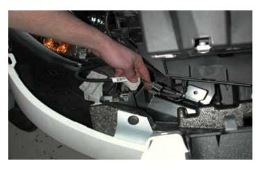
8. With help from an assistant, carefully pull the front fascia loose from the vehicle and unplug the fog lights on each side. Set aside somewhere it will not get damaged.
