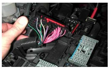
35. Now you will connect the orange wire (from the fan relay harness) to the dark green wire in connector #X2 (sometimes referred to as C2) pin D4. This wire is the AC compressor clutch supply voltage, circuit 59.
