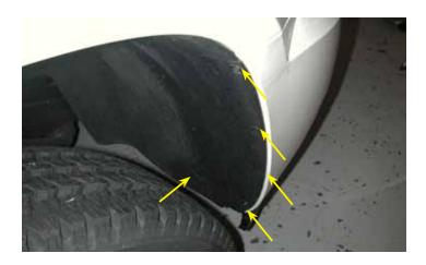
5. Next remove the two 7mm bolts and three push clips from both of the front inner fender wells.
