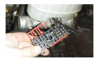
33. Remove the terminal retainers (red plastic clips) from front end of the connector as shown.
