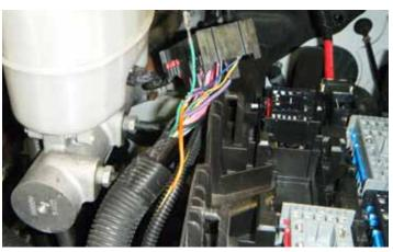
42. Roughly 1-1/2" from the terminal, strip 1/4" section of insulation from the green wire. Cut the orange wire to length and then strip 3/8" of insulation from the end of the orange wire. Splice the orange wire to the green wire by wrapping the orange wire around the exposed section of the green wire and then solder the connection.
