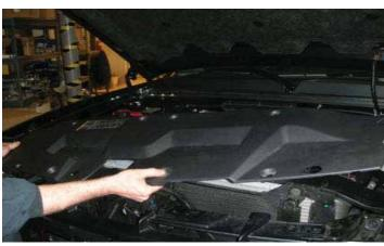
54. Reinstall the radiator support cover on the vehicle using the stock hardware.
