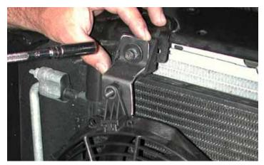
14. The 255 mm (10") fan, the larger of the two fans, will be mounted on the passenger side of the vehicle. Using a 10mm socket, remove the bolt that secures the passenger side upper corner of the AC condenser. Use the factory bolt you just removed to secure the passenger side fan bracket (L960150607).
