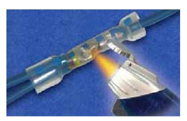
39. Apply heat evenly around the length of the tubing (including the crimp area) from the center out to the ends until the tubing fully recovers and the adhesive flows. During the heating process, separate the two wires in the larger end of the connector to allow the adhesive to flow in between the wires.
