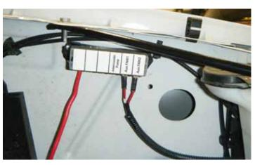
24. Apply the fuse panel decal to the fuse panel cover as shown. Now connect the two red fan harness power wires to the fuse block you installed in step 21. The red wire with the #3 on it, labeled fan #1, goes into the #2 position on the fuse block (labeled Aux FAN1) and the other red power wire goes to the #1 fuse block position (labeled Aux FAN2).
