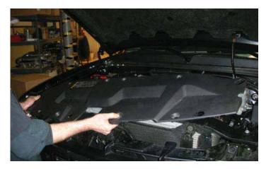
3. Remove the radiator support cover from the vehicle. Set aside to be re-installed later.
