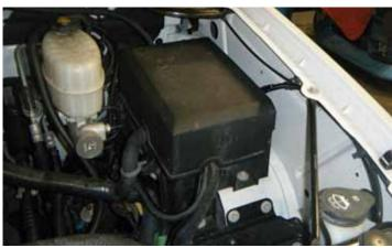
50. Re-install the fuse and relay panel cover.
