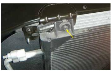
10. Remove the eight bolts on the upper radiator support bracket and then remove the upper radiator support bracket.
