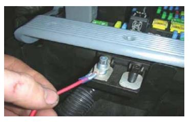
47. Attach the main power wire from the supplied 6 position fuse block to the stud in the factory fuse box using the M8 nut. Tighten using a 13 mm socket.
