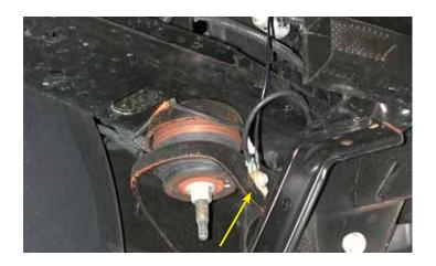
29. On the passenger side, connect the ground wire from the fan # 2 side of the harness to the frame of the vehicle on the passenger side using the existing factory ground bolt found in front of the wheel well next to the end of the bumper beam as shown.
