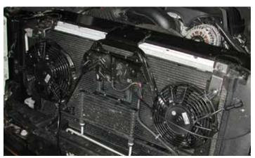
18. Secure the fans to the "A" frame using the supplied self tapping screws (AV12351 & AV12354). On the driver side use the longer 30mm screws along with the supplied 1/4" thick round spacers for the smaller 9" (225mm) fan. Install the spacers between the fan mounting feet and the holes in the "A" frame.
