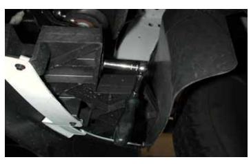
6. Remove the two, one on each side, 10mm bolts securing the plastic fascia support brackets to the metal bumper support brackets.
