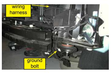
28. On the driver side, connect the ground wire from the fan #1 side of the harness to the frame of the vehicle on the driver side using the existing factory ground bolt found in front of the wheel well next to the end of the bumper beam as shown. Secure the harness in place with Zip ties.
