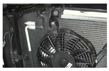
16. Using a 7/16" socket wrench, secure the fan and mounting tab assembly to the bracket using one of the supplied 1/4-20 Spin Lock nuts.
