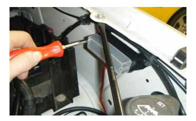
21. Mount the supplied fuse block to the inside of the driver side front fender by drilling two holes (1/8" drill) through the fuse block mounting tabs. Be careful not to drill too far or you risk damaging the outer fender. Now using a Phillips head screw driver secure the fuse block to the vehicle with the two M4.2x1.41x20mm Phillips head self tapping screws.
