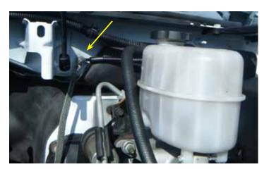
49. Route the ring terminal equipped yellow/black ground wire from the fan wiring harness back alongside the fuse block to the firewall and across the brake booster to the ground stud. Install the ring terminal onto the ground stud and then secure it in place with the factory nut.
