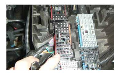
45. Re-install terminal retainer clip on the X2 connector and install it into the fuse black and relay center base.
