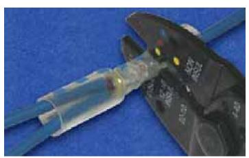
38. On the terminal side of the green wire, strip back the insulation 5/16". Insert the wire into the smaller side of the connector, make sure the wire is properly seated and crimp the connector using an insulated connector crimping tool.
