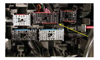
31. Image of fuse block and relay center with cover removed.
