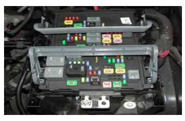
46. Re-install the fuse block onto the fuse block base.
