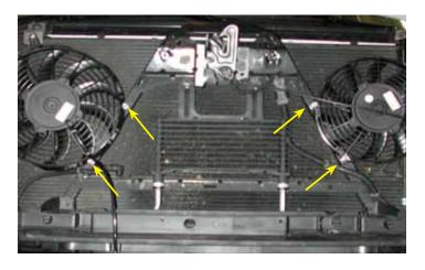
17. Mark with a center punch the location of where the fan shroud mounting holes overlap the factory front support structure as shown on the left (yellow arrows).
