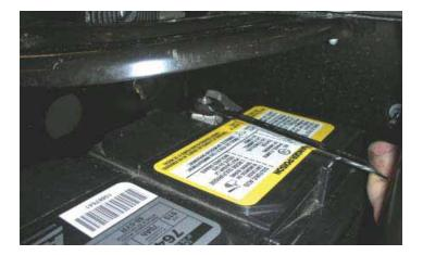
55. Re-connect the battery cable with a 10mm socket wrench.
