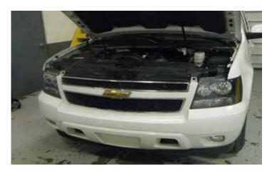
53. Reinstall the front fascia on the vehicle using the stock hardware.
