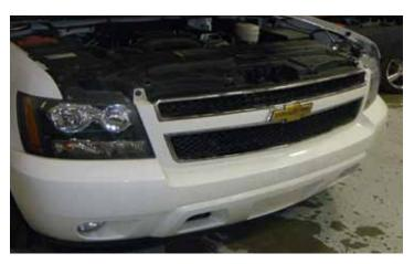
4. The front fascia and grill assembly are all one piece. Start by removing the bolts at the top of the grille.
