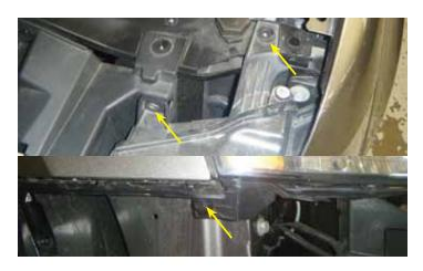
9. Remove the headlights from the vehicle, being careful not to scratch the lens or break the plastic brackets. Two bolts secure each headlight assembly.
