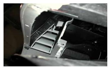
7. Next remove the four bolts, two on each side, holding the fascia to the fenders.
