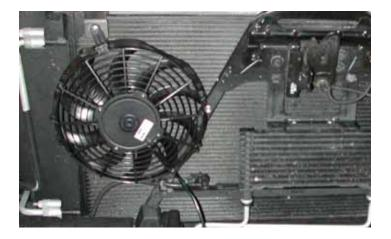
15. Install the remaining plastic fan mounting tab onto the 255 mm (10") fan.
