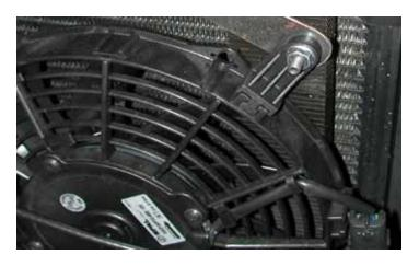
fans will be mounted on the driver side of the vehicle. Install one of the plastic fan mounting tabs onto the 9" (225 mm) fan as shown.
