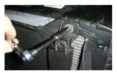
11. Locate the power steering cooler on the driver side of the radiator assembly. Using a 10mm socket wrench, remove the bolt shown that holds the top of the power steering cooler in place. Save this bolt for the next step. Do not remove the cooler.
