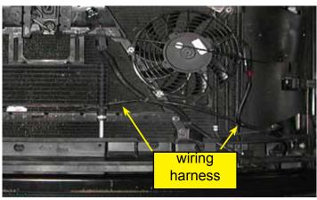
26. Route the fan wiring harness around the radiator support on the driver side and along the front of the truck. Zip tie the harness along the way to hold it in place.
