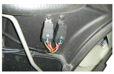
22. Mount the relays to the left-hand side (driver side) of the upper fan shroud by drilling two 1/4" holes into the plastic shroud and securing with the supplied push-lock rivets.
