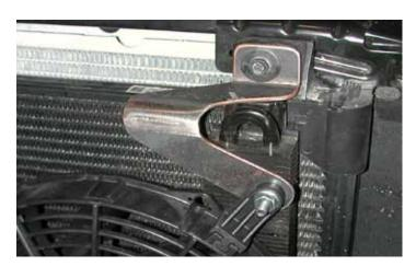
12. Using a 10mm socket wrench, install the driver side fan bracket (L960160607) as shown on the driver side using the factory bolt.
