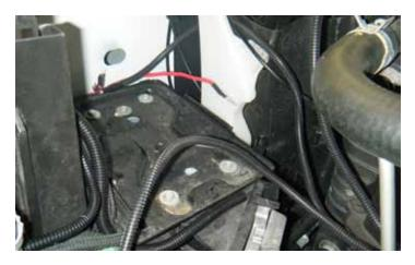
23. With the relays mounted, route the red power wires up and behind the windshield washer bottle and over to the 6 position fuse block.
