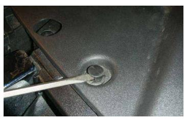
2. Using a pry tool or flat blade screwdriver, remove and save the eight plastic pushpins from the radiator support cover. The pushpins will be used to re-install the cover.
