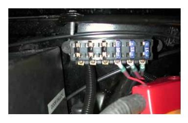
25. Install the two supplied 15 amp fuses into the fuse block in the two far right-hand positions.
