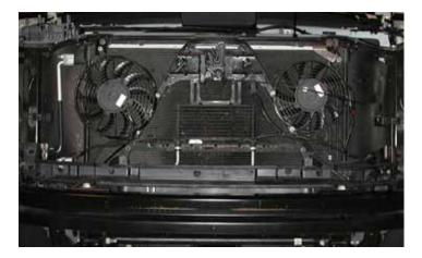
27. Connect the wiring harness to the fans.
