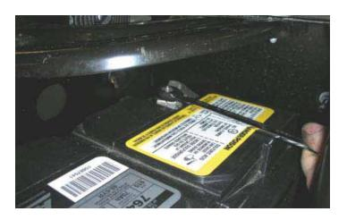
1. Using a 10 mm socket wrench, disconnect the negative (-) battery cable from the terminal on the battery. Cover the cable end with electrical tape so accidental connection to the battery does not occur during installation.
