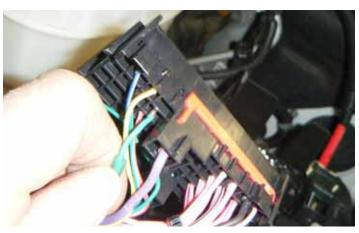
44. Re-install the terminal into the connector X3, cavity D4.
