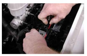
32. Using a pin depressor tool or a small screwdriver, remove connector X2 from fuse block (see fuse block diagram for connector numbers).
