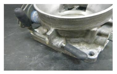
3. The adjacent illustration shows the rubber cap plugs installed on the lower throttle body hose nipples.
