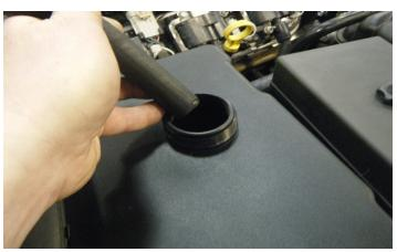
6. Fill the intercooler reservoir with green ethylene glycol. Screw on the pressure cap supplied in the LPE kit (PN: 703-1726). Refer to figure 1 on page 4 for the boiling points of different ethylene glycol aqueous solutions at different pressure levels.
