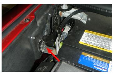
2. Using a 10 mm socket, install the supplied bracket (PN: XX04468-0010) on to the hood latch for the coolant reservoir using the existing fastener.
