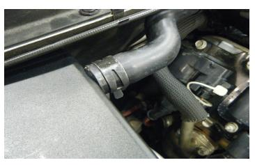
4. Using a spring or constant tension clamp, connect the rear intercooler hose to the top coolant reservoir fitting.
