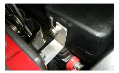
3. Loosely install the supplied M6x1x16mm bolt (PN: 47313) and M6 washer (PN: 91116A150) into the coolant reservoir (PN: XX04468-0015) and slide the assembly into the bracket installed in the previous step. Tighten the bolt to secure the coolant reservoir to the bracket.
