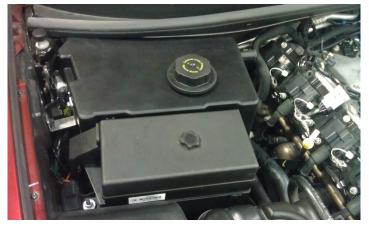
Installation of the LPE intercooler fluid reservoir kit is now complete.
