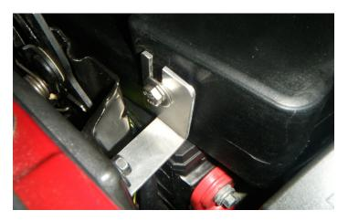
3. Loosely install the supplied M6x1x16mm bolt (PN: 47313) and M6 washer (PN: 91116A150) into the coolant reservoir (PN: XX04468-0015) and slide the assembly into the bracket installed in the previous step. Tighten the bolt to secure the coolant reservoir to the bracket.
