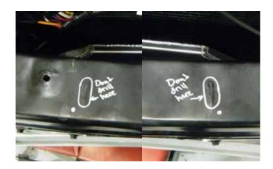
29. Make sure your hole locations do not line up with the two weld marks in the bumper beam (examples shown here).
