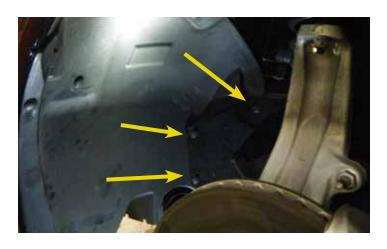
53. Install the engine splash shield and secure with four (4) pins.
