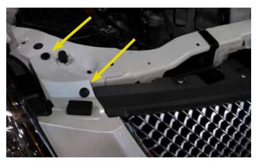
6. Using a fork tool, remove the two (2) push fasteners from each side of the vehicle (four total) that secure the front fascia to the vehicle.
