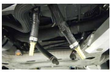
36. Insert one end of each of the two supplied brass barbed unions (PN: LN-TT23) into the ends of the power steering hoses that are attached to the power steering cooler.
