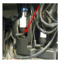
14. The washer fluid pump is located on the passenger side of the vehicle behind the fog light area. Remove the line from the washer fluid pump that is used for the headlight washers. A rubber vacuum cap may be used to prevent washer fluid from leaking until reassembly.
