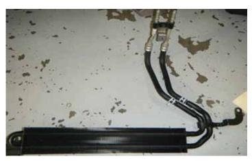
20. Remove the OEM power steering cooler assembly.
