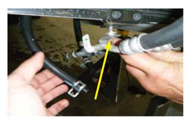
17. Using a 10 mm wrench undo the bolt holding the bracket for the PS hoses.
