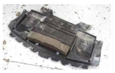
8. The front air deflector is located on the underside of the vehicle and is attached to the front fascia and the front portion of the frame. Remove the two (2) M6 bolts with a 10mm socket, remove the 10 push pins, and then remove the cover.
