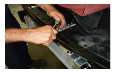
35. Place the power steering cooler back into place on the impact bar. As indicated previously, it is recommended to have the hoses point inwards towards each other. This will help with the packaging of the hoses. Tighten the screws in place using a 3/8" socket and wrench. Torque to 5 lb-ft (7 Nm).
