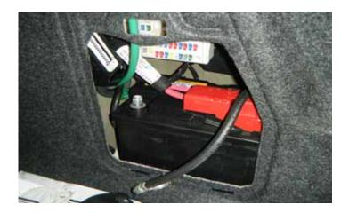
3. Disconnect the ground terminal from the vehicle's battery using a 10 mm wrench. The battery is located in the trunk on the passenger side of the vehicle.
