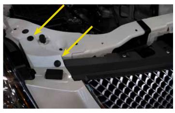
50. Install the two (2) push fasteners on each side of the fascia.
