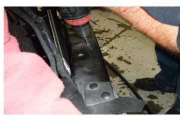
30. Using a punch. mark the center of the holes. Using a 3/16" drill bit drill out the two marked holes. It is recommended to use a carbide drill bit or have a few brand new drill bits as they will dull out quickly when trying to drill through the hardened steel.
