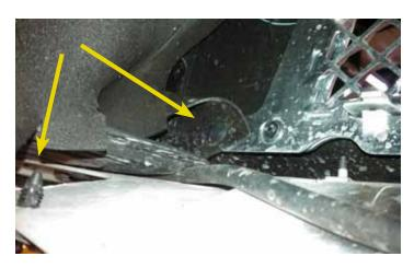
48. Secure the rubber shrouds on either side of the radiator with the Christmas tree fasteners (two per side).
