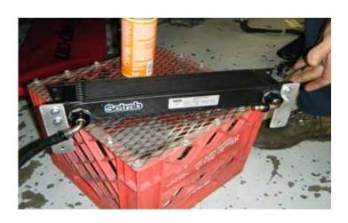
32. Remove the plastic plugs from the supplied power steering heat exchanger. Apply a light coating of oil or O-ring safe assembly lubricant to the threads of the 3/8" pushto-lock 90 degree fittings (PN: SET22-M22PL06-90). Install the 90 degree hose end fittings into the power steering cooler as shown.
