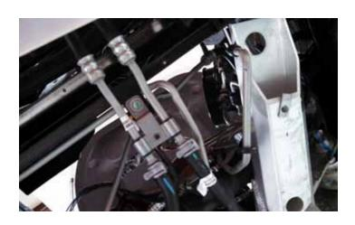
16. Locate the power steering (PS) hose bracket that is found where the PS lines cross under the intercooler radiator and engine radiator on the driver side. Using hose clamp pliers to relieve the tension on the clamps, slide the hose with the attached clamps off of the metal lines and drain the fluid into a basin.
