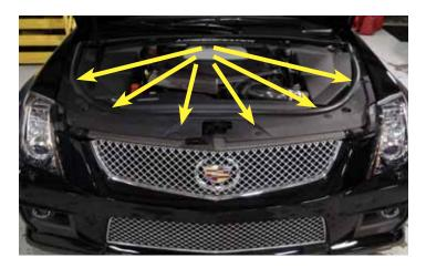
55. Install the sight shield and secure in place with the six plastic retainer clips (clockwise to tighten).
