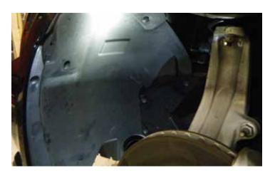
11. Remove the eight push pins holding in the front part of the fender liner and remove the fender liner. Repeat this process for both the passenger and driver side front inner fender.
