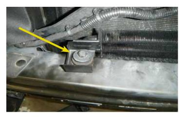
19. Remove the remaining bolt, located on the passenger side of the vehicle, that secures the OEM PS cooler to the front bumper impact bar.
