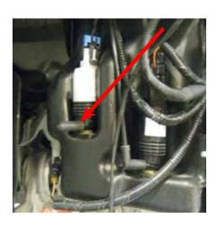
46. Connect the hose to the washer fluid pump.
