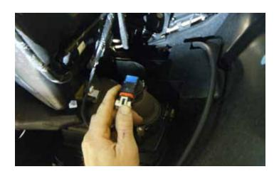
13. Disconnect the electrical connector from each fog light.
