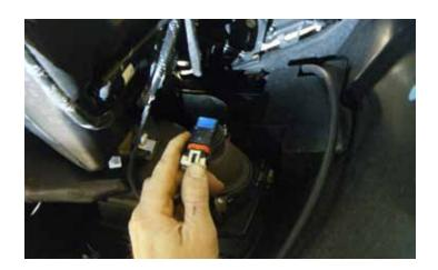
13. Disconnect the electrical connector from each fog light.
