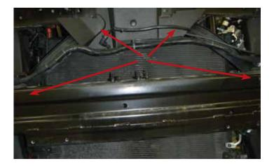
27. Using a 13mm socket, torque the four bolts to 20 lb-ft (27 Nm).
