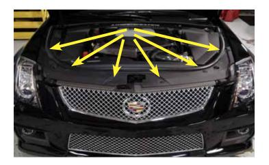
55. Install the sight shield and secure in place with the six plastic retainer clips (clockwise to tighten).
