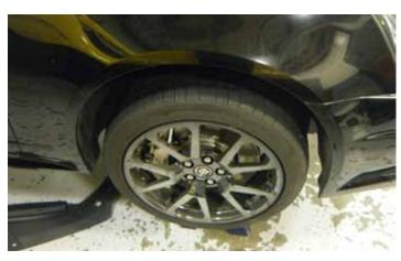
4. Remove the front two wheels. It is recommended breaking the lug nuts loose in a star pattern.
