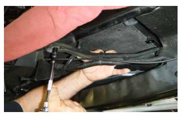
24. Locate the passenger side support brace above the power steering cooler. Using a 13mm socket, loosen the top bolts, one on each brace.
