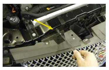
7. Remove the two M6x1.0 screws that secure the fascia to the bumper core support using a 10mm socket.
