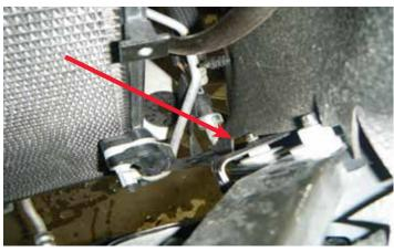
18. Using a 13mm wrench, remove the bolt on the passenger side power steering cooler bracket.
