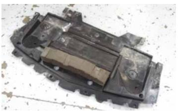
54. Install the front air deflector under the engine.
