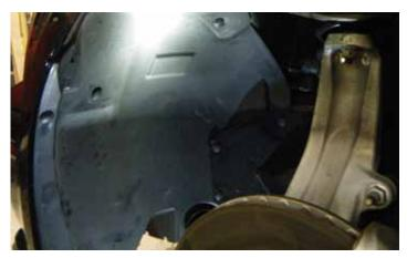
52. Install the front fender liners and secure with eight (8) push pins.
