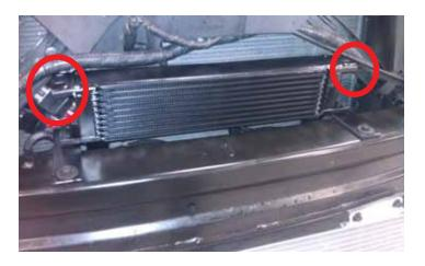
23. Place the power steering cooler in between the diagonal support braces on the front of the core support with the mounting brackets setting on top of the front bumper impact bar.
