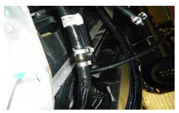
38. Connect the OEM power steering hoses, from the rack and P/S pump, to the brass barbs. Using a pair of hose clamp pliers, release the tension from the clamps and slide the hose and the clamps into place. These clamps are attached to the hose and cannot be moved or rotated.
