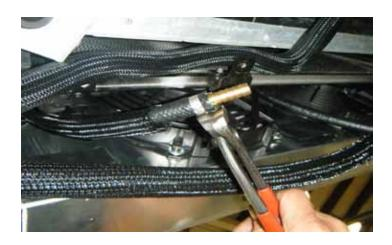
37. Slide one piece of the supplied shrink tubing (DC980845) over each hose section and then install one 17mm Oetiker clamp (PN: 52545K55) onto each of the hoses. Use the Oetiker pliers to secure the brass barbs in place.
