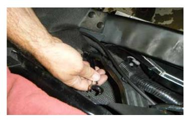
25. Then loosen the bottom bolts. These are located between the impact bar and AC condenser.
