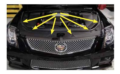
Open the hood and remove the six plastic retainer clips from the sight shield by turning the clips counterclockwise. Remove the sight shield
