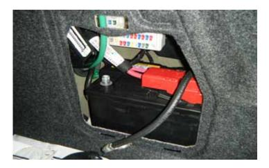
3. Disconnect the ground terminal from the vehicle's battery using a 10 mm wrench. The battery is located in the trunk on the passenger side of the vehicle.
