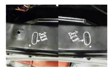
29. Make sure your hole locations do not line up with the two weld marks in the bumper beam (examples shown here).
