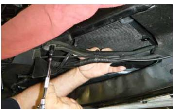
26. To allow the most room for the power steering cooler, tighten the top bolts while pushing up and out on the brace.
