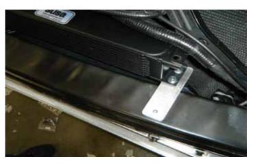
28. Mark the locations for the holes for mounting the power steering cooler with a scribe or marker pen.
