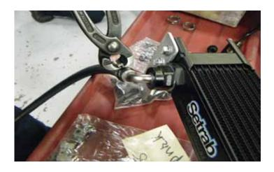
33. Slide the supplied 17mm Oetiker clamps (PN: 52545K55) over the 3/8 hoses from step 27, and then push the hoses (H1937) onto the barbed ends of the fittings. Using Oetiker pliers, crimp the clamps over the hoses to secure them onto the fittings. Install a piece of the supplied heat shrink tube over the hose.
