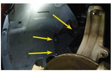
10. In each wheel well, an engine splash shield exists. This felt-like material shield is secured to the wheel well liner with four push pins. Remove the four (4) push pins and remove the splash shield. Repeat this process for both the passenger and driver side splash shield.
