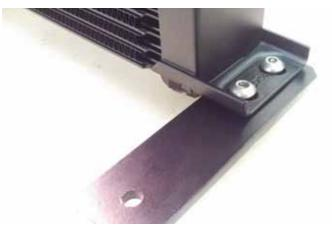
22. Attach the brackets to the cooler using the four (4) 1/4"-20 Nylon insert lock nuts (PN: 30634) and 1/4-20x3/4" button head cap screws (PN: 93107). Using a 5/32" Allen wrench and 7/16" socket, tighten the bolts to 6 lb-ft (8 Nm).
