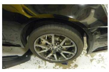
4. Remove the front two wheels. It is recommended breaking the lug nuts loose in a star pattern.
