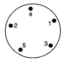
56. Install the front two wheels Have the assistant hold the brakes or lower the vehicle to the ground while you torque the lug nuts. Use a star pattern to tighten.
