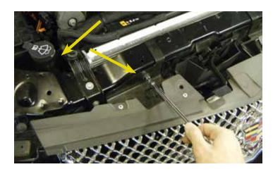
49. Install the M6x1.0 screws that secure the fascia to the bumper core support using a 10mm socket.
