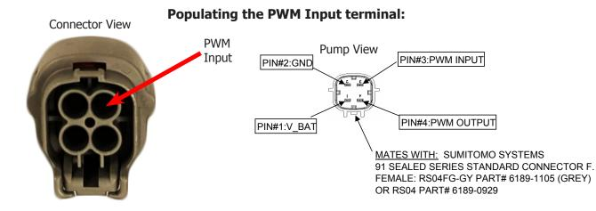
If you would like to control the LPE Varimax high flow intercooler pump by **PWM control**, populate the PWM Input terminal above using the provided terminals and seals. Control information can be found on page 10 and 13.
