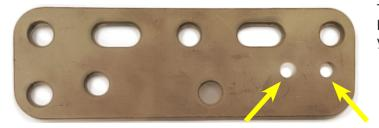
The bolt holes from the clamps above will align with the holes on the bracket (PN: XX00054-0001) indicated by the yellow arrows.
