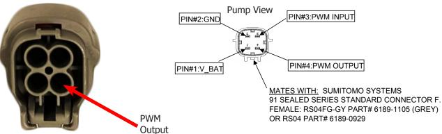
The PWM output terminal is used for diagnostic purposes only. It does not need to be populated in order to control the pump by PWM. If you are not using this terminal, use the provided plugs to plug this hole. More information on page 14.
