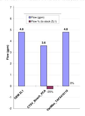
LPE electric intercooler pump flow comparison - CTSV vs ZL1 vs VariMax flow in gallons per minute (GPM) versus differential pressure across the pump (psi) Test conditions: 13.5 volts, 3/4" hose in and out of pumps, variable restriction after pump
