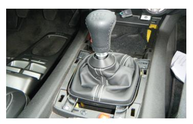
11. Place the LPE shift knob boot adapter onto the gear lever with the tapered end pointing up. Then push the shift knob onto the shift lever. The shift knob should bottom out on the shift lever when the shift knob is adequately pressed on.
