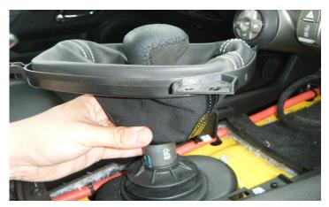
13. Screw the LPE shift knob boot adapter onto the shift knob. The tapered surface of the collar can be difficult to get ahold of, so it may be necessary to screw on the collar from the inside of the shift boot, as shown in the adjacent picture.
