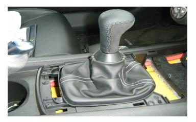
14. Orient the shift boot to it's proper position.
