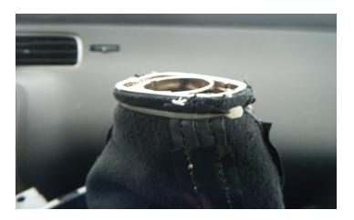
6. Flip the shift boot inside-out. You will see a zip-tie that holds the shift boot to the chrome collar. Using a knife or equivalent, remove the zip-tie, taking special care not to damage the shift boot.
