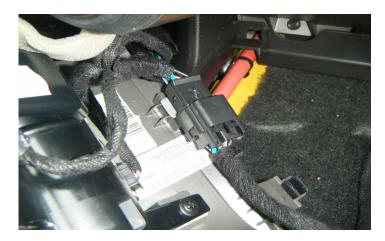
Disconnect the electrical connector on the back of the front cover. The front floor console front cover can now be removed and set aside.
