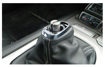
2. Gripping the shift knob above the chrome collar with both hands, pull upward to remove the shift knob.
