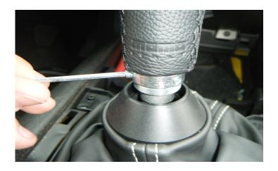
12. Verify that the shift knob is properly aligned. Then, applying constant downward pressure on the shift knob, tighten the three (3) 5mm set screws in a uniform manner to secure and center the shift knob onto the gear lever.
