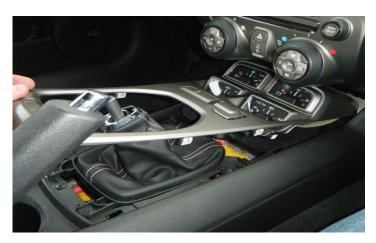
Using a small flathead screwdriver, plastic pry tool, or your fingers, gently pry up on the end of the front floor console front cover. Work your way around the front cover until the front cover completely separates from the floor console, taking care not to damage the plastic console or the retaining tabs that hold it down.
