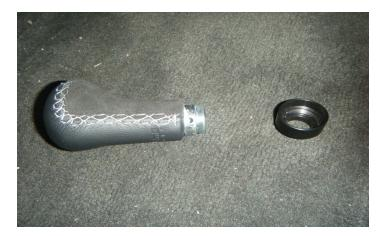
10. Remove the black threaded ring that is screwed onto the end of the LPE shift knob.
