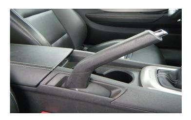
1. Before beginning installation, make sure to apply the emergency brake.
