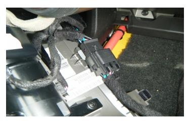
15. Reconnect the electrical connector on the back of the front floor console front cover.
