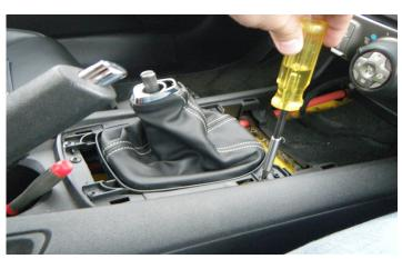
5. Using a #2 Phillips screwdriver, remove the four (4) shift boot mounting screws. The shift boot can now be removed.
