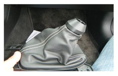
7. After flipping the shift boot back to it's normal orientation, work the LPE shift boot collar into the shift boot as shown in the adjacent picture. The tapered end of the new collar should be pointing up.
