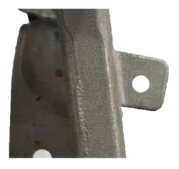
3. Using a drill and a 1/8" drill bit, make a pilot hole in the center of the tab. Then use a 1/4" drill bit to make the hole larger.
