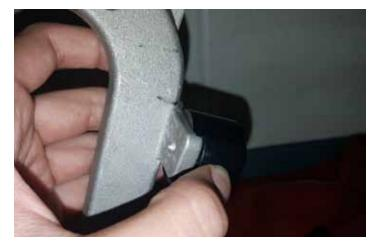
4. Apply Blue Loctite to the threads of the button head socket cap screw, 1/4-20 x 3/4" (PN: 93107). Then place the clutch pedal stop main body (PN: XX07206-0001) over the back of the tab as shown.
