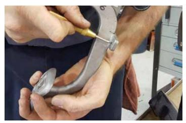
2. Using a center punch, make a divot on the mark you made in the center of the tab in step 1.
