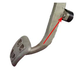
5. Using a 5/32" Allen wrench, tighten the screw with the blue Loctite into the clutch pedal stop main body.
