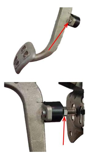
5. Using a 5/32" Allen wrench, tighten the screw with the blue Loctite into the clutch pedal stop main body.
