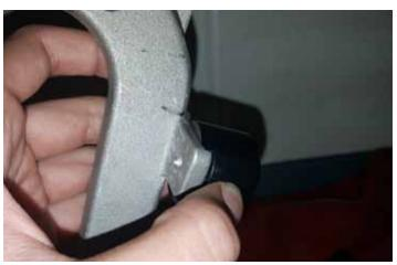
4. Apply Blue Loctite to the threads of the button head socket cap screw, 1/4-20 x 3/4" (PN: 93107). Then place the clutch pedal stop main body (PN: XX07206-0001) over the back of the tab as shown.
