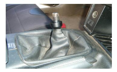
3. Place the black threaded ring onto the shift lever with the tapered end pointed down.
