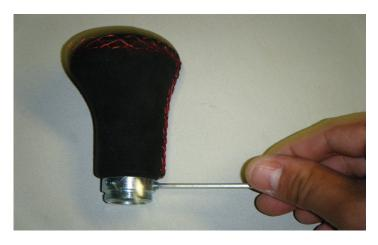
5. Insert three (3) of the supplied set screws into the holes on the LPE shift knob. If your gear lever measured either 8mm or 10mm in diameter, use the longer 6mm set screws. If your gear lever measured 12mm or larger in diameter, use the shorter 5mm set screws. Make sure not to turn the set screws too far into the shift knob as it will prevent the shift knob from fitting over the gear lever properly.
