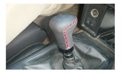
7. Screw the black threaded ring onto the base of the shift knob.
