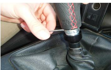
6. Push the shift knob onto the shift lever until it bottoms out. Applying constant downward pressure on the shift knob, tighten the three (3) set screws in a uniform manner to secure and center the shift knob onto the gear lever.
