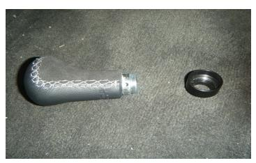
2. Remove the black threaded ring that is screwed onto the end of the LPE shift knob.
