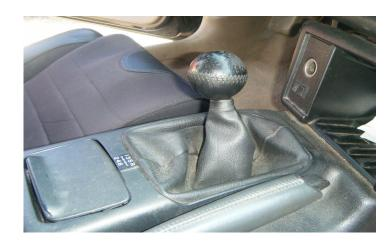
1. Remove the factory shift knob by rotating it in the counterclockwise direction.
