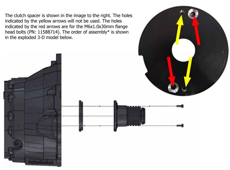
Bell Housing Clutch Spacer Clutch Slave M6x1.0x30mm Flange Head Bolts
