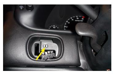
11. Remove the T15 Torx screw behind the release/fog light panel.
