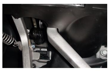
23. Pull the bracket and secure it around the clutch pedal. Using a 1/8" hex key, tighten the set screw to the pedal and install the retaining nut onto the set screw.
