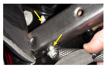
22. Locate the bolt on the frame that is indicated. There is a nut on top of the frame that must be loosend to allow the bolt to drop down. Using two (2) 13mm wrenches or sockets, loosen the bolt so that you can hook the end of the spring around it as shown.
