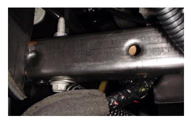
24. Make sure that there is no interference between the spring and the wiring harness. Using a 15mm wrench and socket socket, torque the dash frame bolt to 22 ft-lbs.
