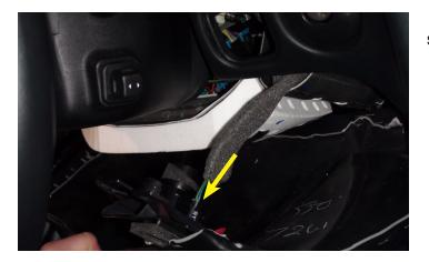
26. Re-install the ambient inside temperature sensor in the lower dash panel.
