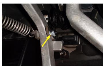
6. Install the locking nut on the end of the set screw. Using a 7/16" socket and torque wrench, torque the locking nut to 89 in-lb.
