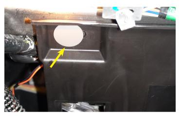
31. Install the plastic push tab on the left of the kick panel back into place.
