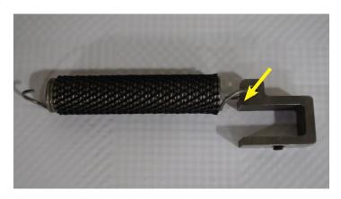
8. One side of the spring has a longer loop on it than the other. Insert the free end of the spring with the longer loop into the supplied bracket.
