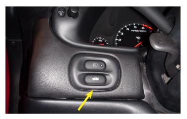
36. Re-install the trunk release/fog light module.
