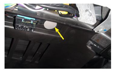
30. Install the plastic push tab on the right of the kick panel back into place.
