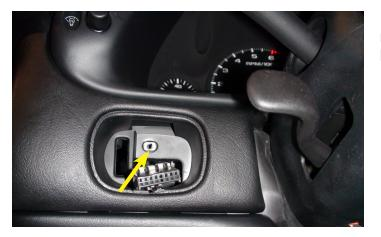
34. Re-install the T15 Torx screw on the trunk release/fog light panel. Torque this bolt to 89 in-lb.
