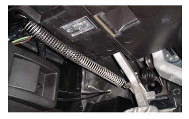
4. Pull the bracket and hook it around the clutch pedal as shown.
