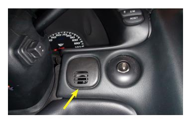
12. Locate the inside air temperature sensor panel on the bottom right side of your gauge cluster. Using a small pry tool, remove this panel.
