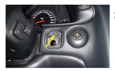
32. Re-install the T15 Torx screw on the ambient inside temperature sensor panel. Torque this bolt to 89 in-lb.
