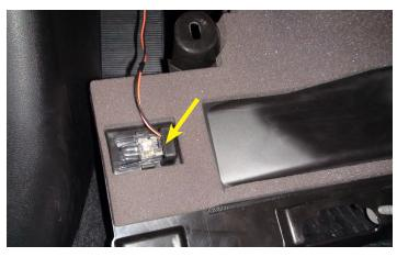
17. Gently pull the kick panel down. Remove the light on the inner portion of the kick panel.
