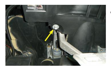
16. Using a pry tool, remove the metal push clip located above the clutch pedal.
