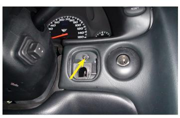
13. Remove the T15 Torx screw from behind the panel.
