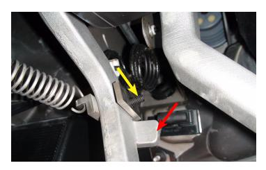
5. Slide the bracket down to the machining tab on the clutch pedal as indicated by the red arrow. Insert the set screw and, using a 1/8" hex key, tighten it down to secure the clutch return spring bracket to the clutch pedal.
