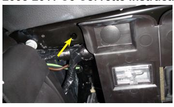
1. Locate the hole directly above the hood release lever located on the driver side foot well underneath the dash.
