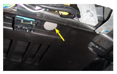
15. Using a pry tool, remove the push clip from the right side of the kick panel located next to the OBD-2 connector.
