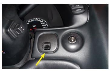
33. Re-install the plastic panel over the ambient inside temperature sensor.
