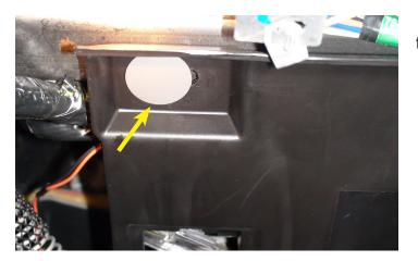
14. Using a pry tool, remove the push clip from the left side of the kick panel.
