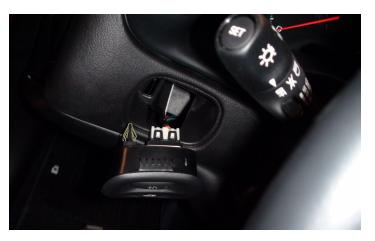
35. Reconnect the trunk release/fog light electrical connector.
