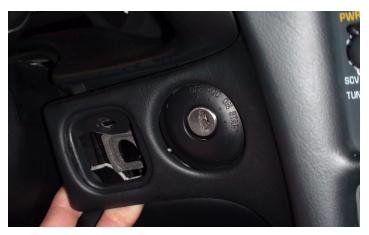
19. Gently pull the left side of the front dash panel toward you and remove the lower dash panel from behind it as shown.
