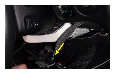
20. Disconnect the ambient inside temperature sensor from the lower dash panel.
