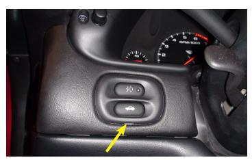
9. Locate your trunk release/fog light panel located on the bottom left side of your gauge cluster. Using a small pry tool, pop the panel out from the bottom of the instrument cluster.
