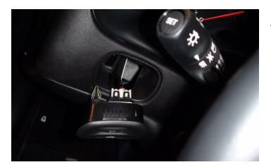
10. Remove the connector from the back of the panel and set it off to the side.
