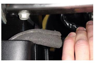
21. Locate the 13mm bolt above and slightly in front of the hood release. There is a brace that holds the wiring harness to the frame. This must be removed to relocate the wires away from the spring on the clutch return spring bracket.
