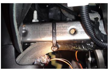
25. Move the wiring harness over to the right and secure it with the supplied cable tie as shown. This is to prevent the wiring harness from getting pinched between the spring.
