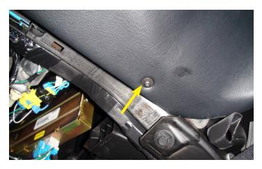
18. Remove the two (2) T15 Torx screws located on the bottom of the lower dash.
