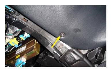
28. Re-install the two (2) T15 Torx bolts on the bottom of the lower dash panel. Torque both bolts to 89 in-lbs.
