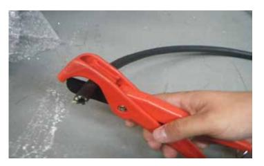
5. After test fitting the rubber hose (PN: 5283K31) from the bladder to where it will connect to the differential, cut the hose to length.
