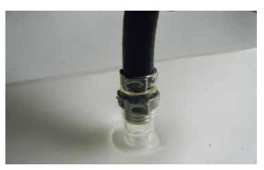
6. Using the two (2) 13.3mm Oetiker clamps (PN:52545K51) and the correct length of hose, connect the hose to the hose joiner and the differential.
