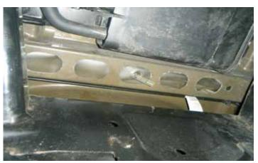
2. Place the bladder (PN: XX04556-0010) into the undercarriage of the vehicle. For 5th generation Camaros, LPE generally recommends placing the bladder in the vehicle's frame, just above the differential. Make sure that the bladder's cut breather tube is portruding downward from the frame, as shown in the adjacent picture.
