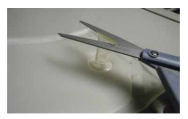
2. In some cases, it may be desirable to run a vent hose from the bladder to a higher point on the vehicle. If this is required for your application, simply cut the tip off of the breather to connect to the differential and connect a hose to the breather. On the other end of the hose attach a breather fitting.
