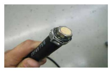
**OPTIONAL STEP:** If installing the breather fitting, run a second hose from the bladder to a higher point on the vehicle so that the fluid drains back down to the bladder. Attach the breather fitting to the hose and use an Oetiker clamp to secure them together.
