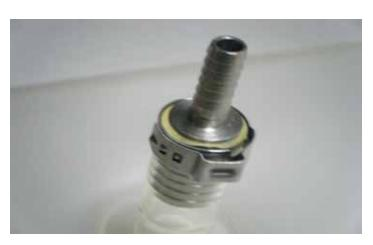
4. Press the 1/4" to 1/2" hose joiner (PN: WWG4HFL2) into the bladder tube selected in the previous step. Secure the hose joiner to the bladder using a 17.0mm Oetiker clamp (PN:52545K55). Tighten the clamp with a pair of Oeticker clamp pliers (or equivalent).
