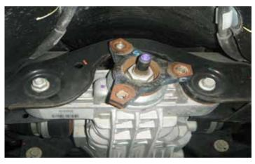
4. Connect the bladder to the differential and reinstall the rear subframe.
