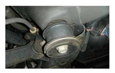
1. Using a floor jack to support the weight of the subframe, remove the four (4) rear subframe bolts. Slowly lower the subframe. Lowering the rear subframe will provide adaquate clearance for installation.
