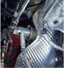
**14.** Use a 7/8" O2 socket and ratchet to remove the O2 sensor from the factory manifold. Keep for Install Step 10.
