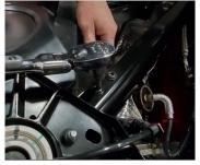
**16.** Reinstall the cross brace from removal step 9-10, then using a T40 torx head, tighten the bolts to the factory torque specification.
