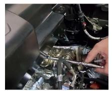
**15.** Use a 7/8" O2 socket and ratchet to remove the O2 sensor from the factory cat. Keep for Install Step 6.
