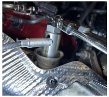
Reinstall the O2 sensors into the headers or exhaust manifolds. Torque to factory specifications
