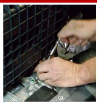
11. Replace the air box from removal step 18. Using a 10mm socket and torque wrench tighten the bolts to the factory torque specification holding the air box in place.
