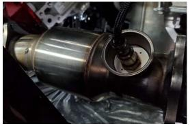
Install the new cats in their place. Secure to the manifold or header with 15mm nuts. Snug the nuts.
