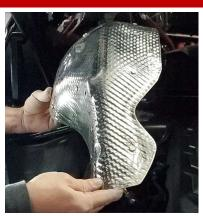
**12.** Remove the heat shield and set aside to be reused in install step 9. Repeat steps 11 and 12 for both sides.
