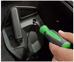
Using a T15 torx head screwdriver, remove the (4) screws holding the plastic pieces as shown. Then remove the plastic pieces. Keep for reinstall step 20.
