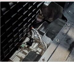
**12.** Re-install the harness clips to the airbox.
