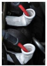
Install the plug heat shields over the spark plug boots. Then plug all the spark plugs back in.
