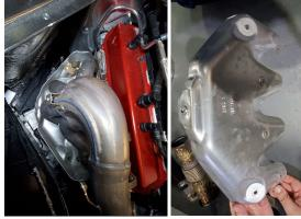
**24.** Use a 10mm wrench to remove the 2 bolts holding the bottom heat shield on. Then remove the shield.
