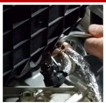
**17.** Using a clip remover, remove the clip holding the harness on the bottom of the air box.
