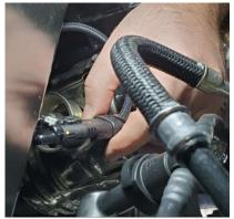
**14.** Plug the all the O2 sensors back into the harness. Into their correct locations
