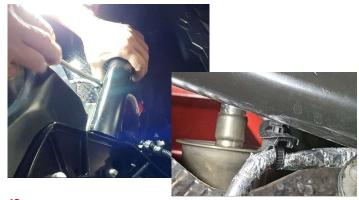
**10.** Before pulling the brace, use a clip remover or screwdriver to remove harness clip. Repeat steps 9 and 10 for both sides.
