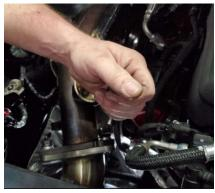
**9.** Using a 15mm wrench, tighten the flange bolts. Then torque all the flange bolts and hanger bolts to factory specifications. Repeat steps 7-9 for both sides.
