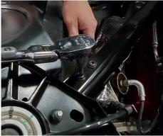
**9.** Going topside again, using a T40 torx head, remove the bolts holding the cross bracing. Keep this for install step 16.
