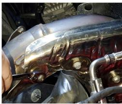
**22.** Using a 10mm wrench, remove the 3 bolts holding the top heat shield on. Then remove the shield.
