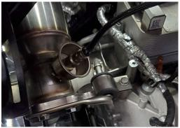
**8.** Install the hanger to the cat and frame using 13mm bolts provided and the 10mm bolts saved from uninstall step 19. Hand tighten.
