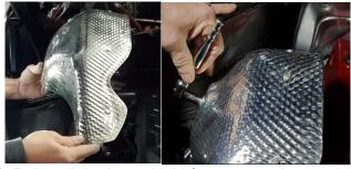
15. Reinstall the heat shield from removal steps 11-12. Use a 10mm socket and ratchet to tighten the bolts. Repeat for the other side. \*NOT USED WITH HEADERS.
