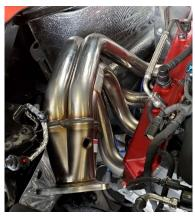
Using the provided hardware and gaskets, bolt the header to the head. The heat shielding is not re-used. Follow the factory torquing specification and procedure. Repeat for both sides.
