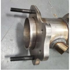
**4.** Install the studs on the outlet sides. 16CG4063 uses (2) M10 x 62mm on the outlet side.
