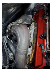
**23.** Use a 10mm wrench to remove the 3 bolts holding the middle shield. Then remove the shield.
