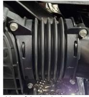
**13.** On both sides of the intake box, use a 10mm socket to re-install the flex connections from removal step 16. Tighten to factory torque specifications.
