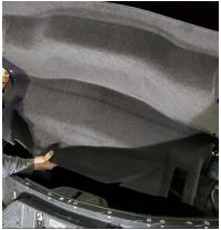
Remove the entire carpet section and set away for re-install step 19.
