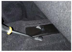
Using a clip remover tool, remove the (2) clips per side holding the carpet in the trunk. Keep for re-install step 19.
