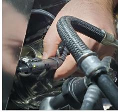
**13.** Unplug all the O2 sensors from on both sides. Label the sensors by where they were removed from. There should be 4 sensors total.
