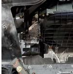
**16.** On both sides of the intake box, use a 10mm socket to remove the flex connections.
