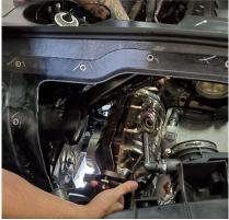
**20.** Using a 15mm socket and ratchet, remove the (3) nuts holding the cats to the exhaust manifolds. Then remove the cat. Repeat for both sides.
