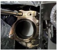
**8.** Starting underneath the vehicle. Using a long extension and a 13mm socket, remove the bolts holding the hanger to the factory cat assembly. Repeat for both sides.
