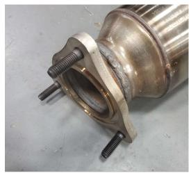
**3.** Install the inlet studs on both cats. The inlets require (3) M10 x 42mm studs on each cat.
