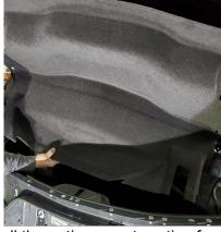
**19.** Re-install the entire carpet section from removal step 4. Secure with the clips from removal step 3.
