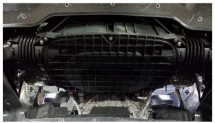
Once the section is removed, you will have access to the air box.
