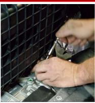
**18.** Using a 10mm socket and ratchet, remove the (2) bolts in front and (2) bolts in back holding the air box in place. Then remove the air box.
