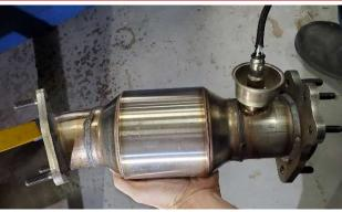
**6.** Install the O2 sensor as shown. Torque to factory specifications. Make sure they are on the same side as removed. Repeat for both sides.
