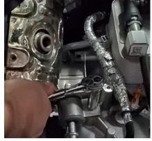
**19.** Using a 13mm socket and ratchet, remove the single bolt holding the cat hangers to the frame. Repeat for both sides.
