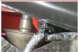
17. Re-install the harness clip under the brace
