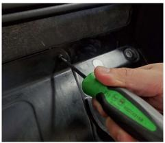
**6.** Using a T15 torx head screwdriver, remove the screws as shown. Keep for re-install step 18.
