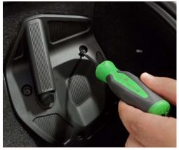
**20.** Using a T15 torx head screwdriver, reinstall the plastic pieces from removal step 2.
