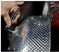
**11.** Using a 10mm socket and ratchet, remove the bolts holding the heat shields over the headers.
