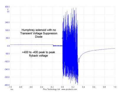
In an automotive environment there can be many sources that can create harmful voltage spikes. The captured scope image to the left is the actual flyback voltage produced when a common control solenoid is switched OFF. Peak voltages of +/- 400 volt are present. This flyback voltage can and will cause intermittent and permanent failure of electronic devices.
