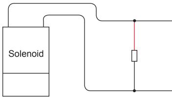
Install the TVS diode across the solenoid wires as close to the solenoid as possible. Polarity does not matter (Red and Black wires can go to either solenoid wire). If there is no accessible ground terminal to connect the diode to, such as the case with a transbrake solenoid, the diode should be connected to the nearest ground source. In the case of the diode for the trans-brake solenoid, the diode should be connected to the transmission case as it will provide a ground path.
