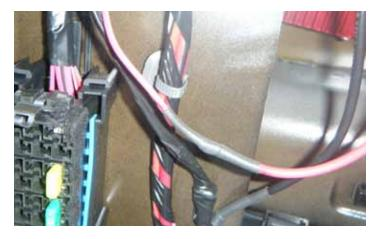
9. Using a small screwdriver, pop the fuse box out of it's base and, using a pin tool remove the FSCM wire (circuit 2640) from the pin location listed below. Cut the terminal off and strip the end of the wire.
