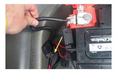
20. Install the in-line fuse connector as shown and connect the ring terminal from the power wire to the battery.
