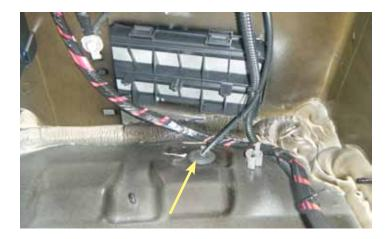
29. Locate the rubber grommet in your trunk located on the passenger side next to the vent. Drill or cut out the center as shown. Slide the end of the activation cable, with red and black wires from the BAP module, down through the drilled or cut hole in the grommet.
