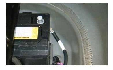
37. Re-install your negative battery terminal to your battery and your interior in your trunk Removed in step 1. Remove your jack and jackstands and start your vehicle.
