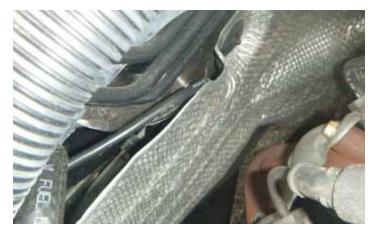
31. Route the wire up to the front of the vehicle, tie wrapping it around the fuel lines every 1-2 feet. Route the wire behind the heat shield, as shown, to the pressure or vacuum switch.
