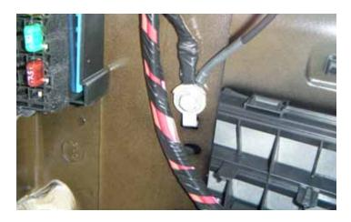
12. Install the ground wire running off of the BAP module to the factory ground located to the right of the fuse box.
