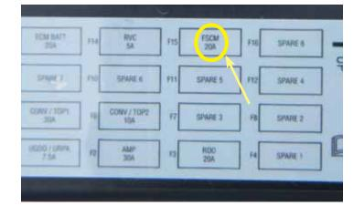
8. In the passenger side trunk of the car, remove the fuse box cover and locate the FSCM fuse on the fuse box cover and remove that fuse from the fuse box.
