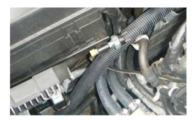
21. Wrap the wire in the supplied high temp black loom. Zip tie the power wire to factory wiring harness to hold it into place.
