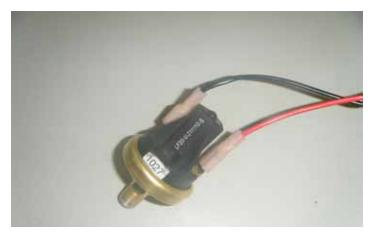
33. Using the butt splice connectors supplied with the kit, Connect the remaining wires from the pressure switch connector to the red and black wires in the activation cable. The polarity of the wires is not critical. Use a heat gun to seal the connectors after they have been crimped.
