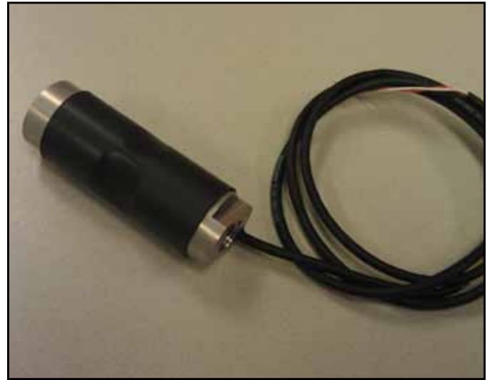
LPE intermediate load cell adapter PN L350180000
