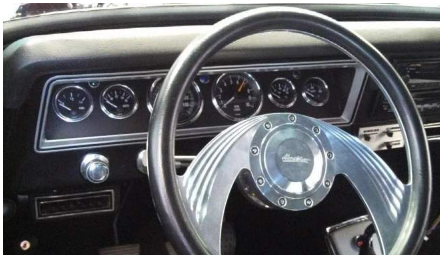
LPE customer vehicle with LS7 engine and CAN2-002 module used to control the VDO oil pressure and water temperature gauges.
