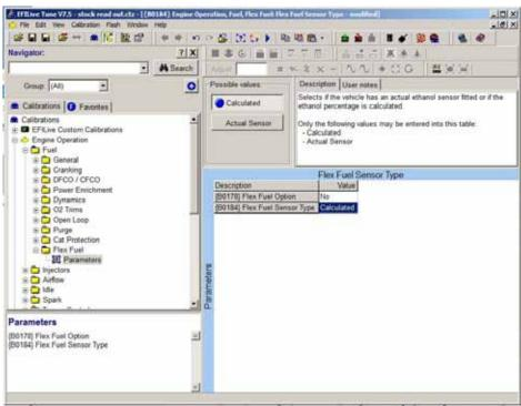
Double-click on 'Parameters' to bring up the window shown in the illustration above. This calibration is currently set to "Flex Fuel Option" "No." Set the "Flex Fuel Option" to "Yes." "Yes" indicates the vehicle is capable of running on Ethanol/gas blended fuel. Set "Flex Fuel Sensor Type" to "Actual Sensor."
