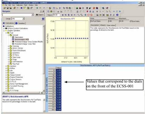
4. In the "Navigation" window, under the "Calibrations" tab on the left side of the screen, navigate to the Flex Fuel Parameters ("Engine Operation" → "Fuel" → "Power Enrichment"), to reach the Power Enrichment Fuel related calibration parameters. Adjust the "P.E. Mode Commanded Fuel" and "P.E. E80 Mode Commanded Fuel" tables to the desired values.
