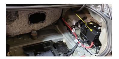
8. Remove the rear body fuse block cover.
