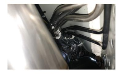
47. Route the FPVB activation wires alongside the fuel line between the fire wall and the engine.
