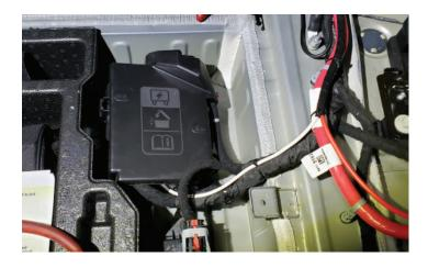
29. Reinstall the body wiring harness junction block cover.
