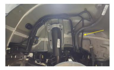
40. Reconnect the three connectors and mounting clips.
