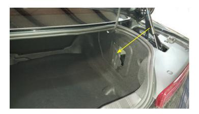
63. Reinstall the battery access panel that is located in the trunk.
