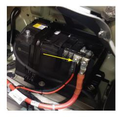
13. Remove the body wiring harness terminal nut using a 13mm socket.
