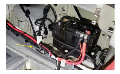
17. Route the black wire from FPVB to stud indicated by the yellow arrow. Cut the black wire to length, slide on 1.25" of heat shrink, crimp eyelet\*, and then heat up the heat shrink.
