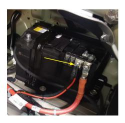
15. Slide the red wire ring terminal over the stud. Reinstall the nut and torque to 106 lb-in (12 Nm).
