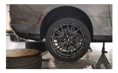
31. Remove the passenger rear wheel using a 22mm socket.
