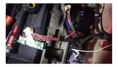
26. Remove pin 29, red/violet wire, from connector X1 using a depinning tool.
