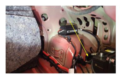
34. Run the FPVB control wires to the grommet indicated by the yellow arrow. Mark FPVB control wire loom at grommet. Cut the loom (not the wires). Remove the section of loom from the control wires. The loom will be used later.
