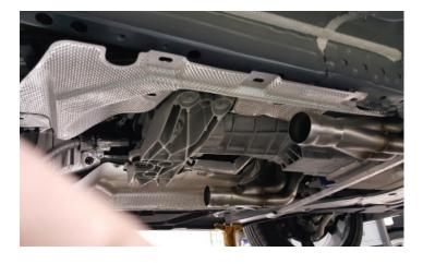
44. Remove the heat shield to access the fuel line.
