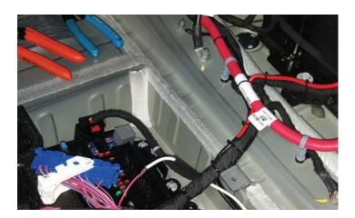
23. Slide a section of heat shrink over the Booster wire (white), and then connect the white wire to the red/violet wire from X2 pin 3 (using splice clip) and then heat the heat shrink. Reconnect the connector back onto the body wiring harness junction block. Vehicles that are not equipped with the electronic axle positraction-limited slip differential (-G96) please skip to step 29.
