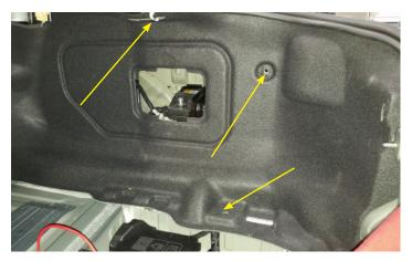
59. Reinstall the rear compartment side trim by reinstalling the 3 push rivets in the location shown by the yellow arrows.
