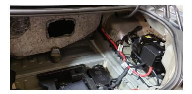
Slide the rear compartment side trim out of the way to gain access to the wheel well. Use a weight to hold the panel out of the way.
