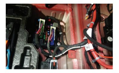
28. Slide a section of heat shrink over the Booster wire (white), and then connect the Booster wire (white) to the red/violet wire from X1 pin 29 (using splice clip) and then heat shrink. Reconnect the connector back onto the body wiring harness junction block.
