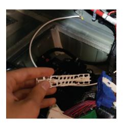
20. Remove the white security lock from connector X2.
