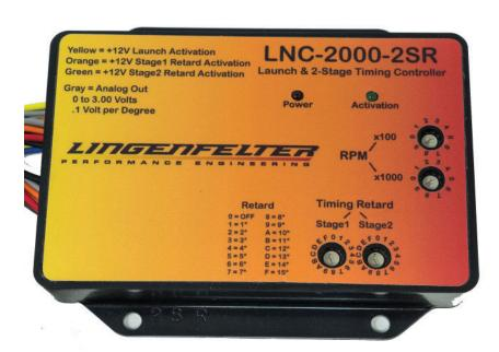
The amount of spark retard for each stage is determined by the appropriate switch for each stage. Example - 8 degrees at launch set Stage1 switch to "A" and apply an activation signal to the Orange wire at launch. 6 degrees for Stage2, set Stage2 switch to "6" and activate the second stage with a timer or output from a nitrous controller. This would result in a total of 14 degrees of retard once both stages are activated.
