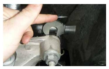
6. This illustration shows how the rear (single slot, XX04468-003) subframe spacers are installed.
