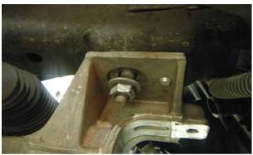
4. Loosen, but do not remove the four (4) front subframe nuts. The nut must be loosened enough for the subframe to drop by 1/2".
