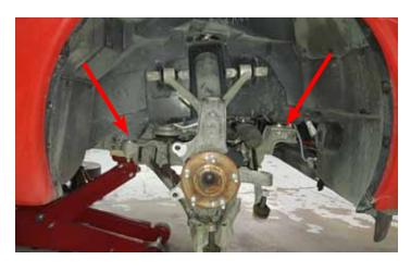
3. You will be installing two spacers on each side of the vehicle. The locations in the front wheel wells are indicated by the arrows.
