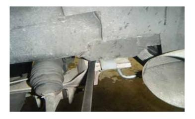
5. You may have to pry down the subframe from the body using a pry bar as leverage. A temporary spacer may be used between the subframe and the body to hold the subframe down until you are prepared to install the subframe spacers.
