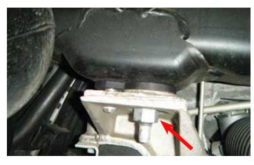
8. Tighten the four (4) engine cradle nuts. Torque the engine cradle mounting bolts to 110 Nm (81 ft-lbs). You may need to pry down on the subframe to get it to lower.
