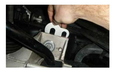
7. This illustration shows how the front (double slot, XX04468-004) subframe spacers are installed.
