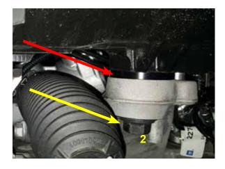
7. Remove the subframe bolt labeled 2. Insert one (1) of the smaller spacers (XX06699-0007) between the body and the subframe. Re-install the bolt but do not completely tighten.
