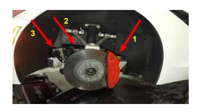
3. You will be installing three spacers on each side of the vehicle. The locations in the front wheel wells are indicated by the arrows. The number associated with each subframe bolt will be mentioned later in the instructions.
