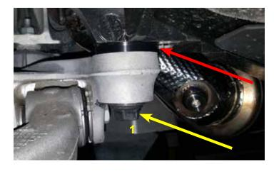
6. Remove the subframe bolt labeled 1. Insert one (1) of the smaller spacers (XX06699-0007) between the body and the subframe. Re-install the bolt but do not completely tighten.
