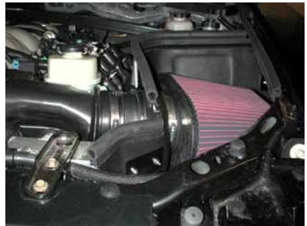
Figure D: heat shield with rubber seal.
