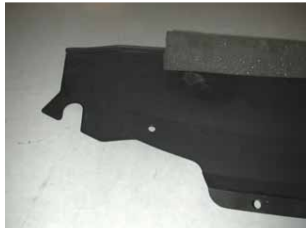
Figure B: radiator shroud without clips.
