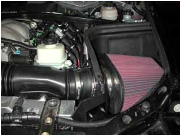
Figure C: heat shield without rubber seal.
