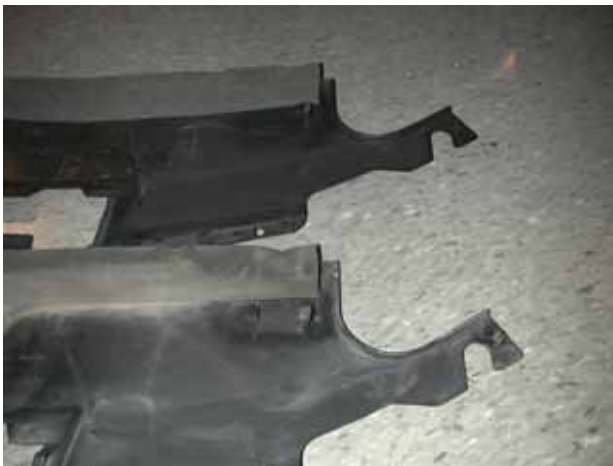
Figure A: radiator shroud with clips.
