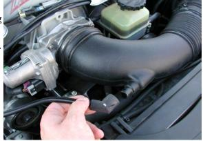
**Step 5 -** Pull the coolant overflow tube from the retainer on the air box and free the MAF wire loom from the airbox. Pull straight upward "firmly" to remove airbox. You will feel resistance, however the airbox should pull out without removing any fasteners.
