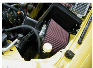
**Step 26** - Reinstall the stock airtube by first plugging in the MAF connector. Reinstall the grey retaining clip at this time.
