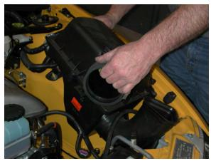
**Step 6 -** In the void where the airbox was, you will see a fastener with a T-30 Torx head, remove this fastener. This will serve as a mounting stud for the air box in a later step.
