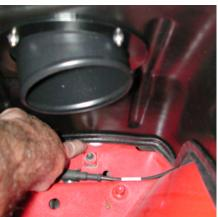
**Step 24** - Remove the air filter from its packaging. This filter comes pre-oiled and is ready to be installed. Filter maintenance kits are available through LPE.
