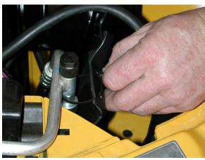
**Step 22** - If there is a gap between the airbox seal and the body of the car, push the seal towards the body.
