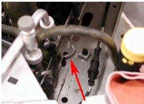
**Step 14** - Using pliers, grasp a corner of the perforated section. Use a twisting motion to remove the section, twist in the same direction until free from the airbox.
