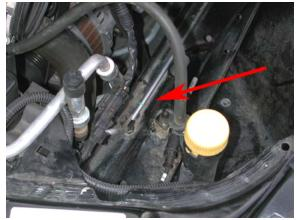
**Step 13** - If the line is shaped as shown (see image), you must remove the small perforated section of the air box (STEP 14).
