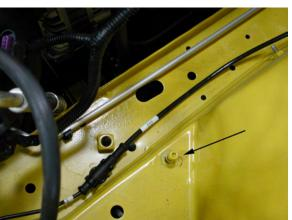
**Step 7 -** Remove one of the black rubber grommets from the bottom of the stock airbox. Insert this grommet into the hole on the inner fenderwell as shown, with flat side out.
