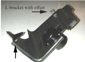
**Step 11 -** Using the supplied M6 flange nut, install the factory Torx head stud (removed in an earlier step) onto the "L" bracket as shown.
