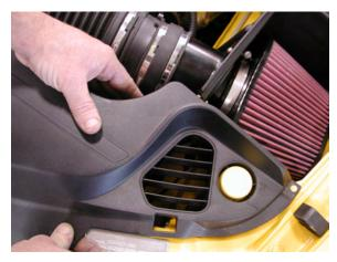
**Step 31** - Install the airbox seal on the top edge of the airbox as shown.
