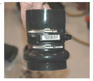
Slide another 90-110 mm clamp over the straight hose section and attach the supplied plastic air-bridge to the other end of the 3.9" hose with the nipple on the hump hose in the 10 o'clock position as shown.
