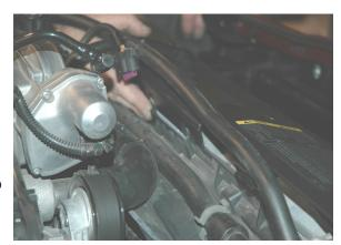
Remove the 3/8" barbed plastic quick couple from the accordion section of your stock air intake system (see picture).
