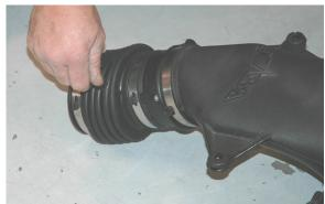
Install the quick coupler into the silicone hump hose by pushing the barbed side into the 3/8" nipple on the hump hose. Do not use lubricant.
