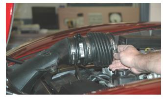
Work entire assembly free from push pins & remove assembly from car.
