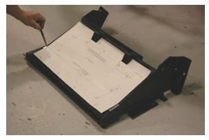
Secure the template in several places with tape. Use a center punch to mark the centers of the holes to be drilled. You should have 19 center punch marks. It is important to make sure you do not remove the template until all 19 holes are marked.
