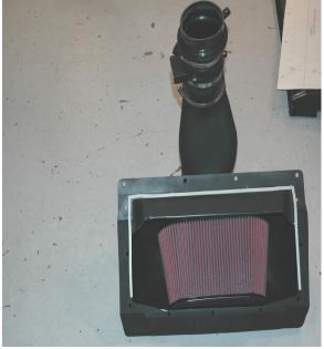
Slide airbox and filter assembly in place as shown.
