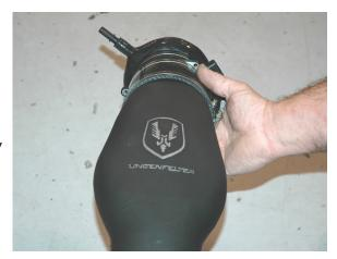
Remove the protective cover from the LPE supplied air filter.
