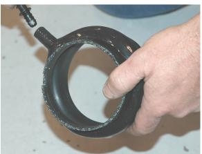
Install 90-110 mm clamp over the notched side of the hump hose and install the black plastic side of the MAF sensor into the hump hose. Be sure to align the cut out notch on the hump hose with the protrusion on the MAF sensor.
