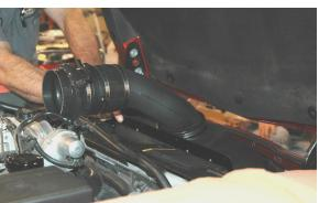
Place the remaining 90-110 mm clamp on the hump hose and connect the 4.0" hump hose to the throttle body. Push the hose firmly as shown to seat the hump hose onto the throttle body. Make sure the bottom is butted up to the throttle body flange. Tighten the clamp securely.
