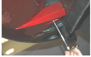
Guide the side wings of the radiator shroud around the lower brackets. Remove the shroud from the top side, pushing condenser rearward as necessary for clearance. If the shroud does not clear the bumper during removal, it may be easier to free it from the under side of the vehicle.
